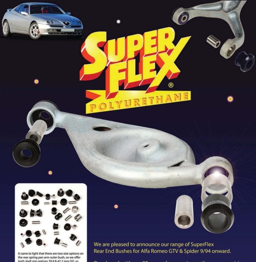
It came to light that there are two size options on the rear spring pan arm outer bush, so we offer both shell size options 39.9 & 42.2 mm OD, so please be aware of this option when ordering. The spring pan arm outer bushes are designed to rock as the original greased steel ball, whilst minimising radial movement – hence the hour glass profile & suitable stainless shell. The sharp edges of the arm housing would be detrimental to a conventional flanged bush.
