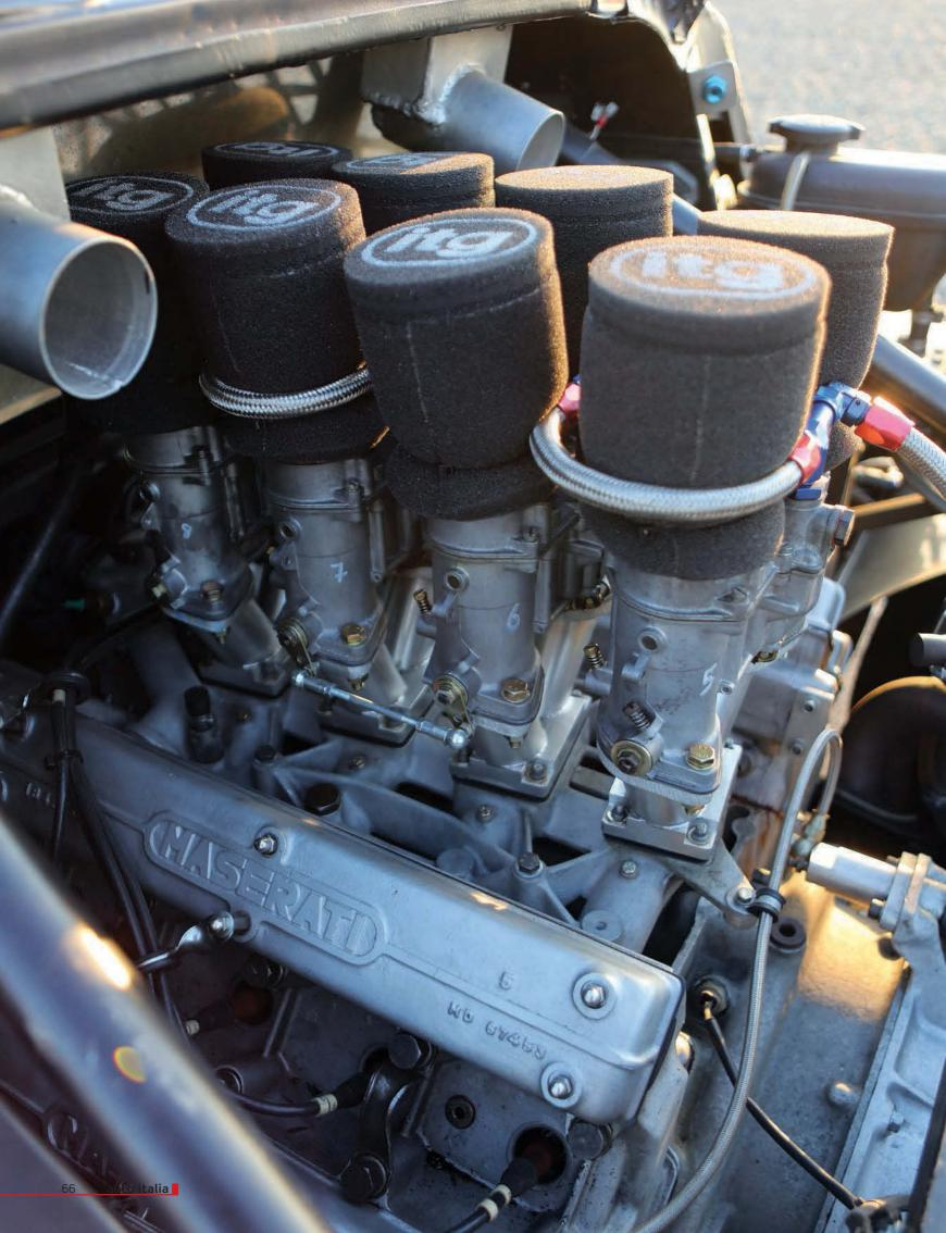
Autodromo di Modena and the final configuration, which featured the Maserati 2.7 V6 engine followed by the 3.0-litre unit of the Merak and the Citroën SM. The SM's transmission was also employed. He also mentioned the three mysterious special electronic injection 24-valve engines that Maserati made for Ligier. They were never used because the company had been sold during that time. One of these units is on display in Bernard Guénant's Trident showroom.
