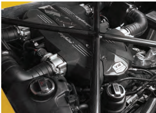
ABOVE: The engineers found another 40bhp by raising the rev limit to 8300rpm, altering the variable valve timing and redesigning the exhaust
