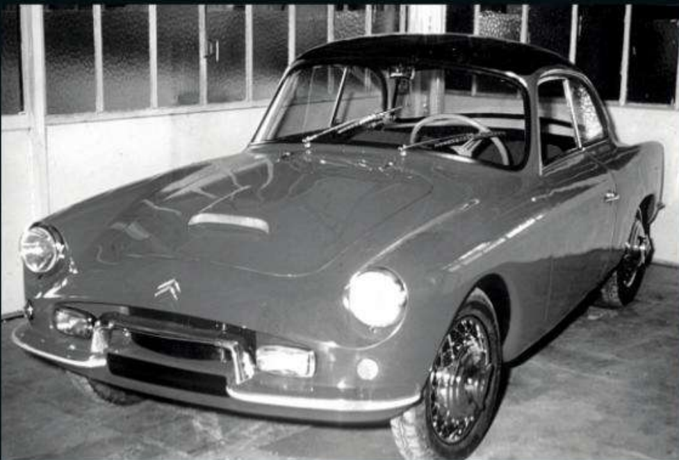
UMAP was designed by Gessalin on 2CV underpinnings, and Chappe produced the moulds
