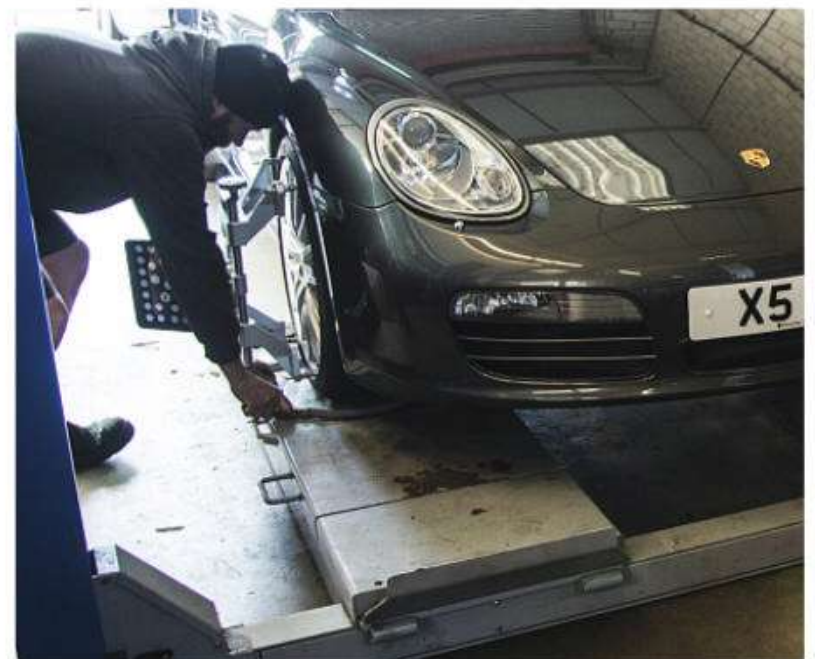
The latest computerised set-up sees to steering and wheel alignment
