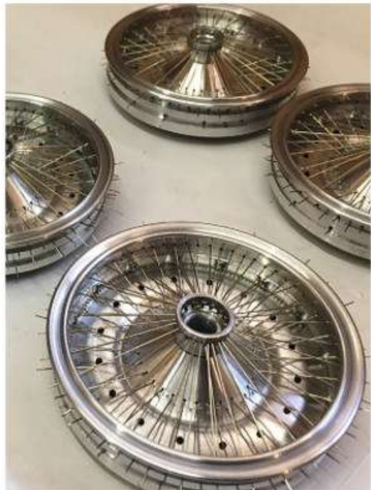
Top: the steering works, and the throttle operates meshed gears on the carbs. Above: spokes are drilled and fitted individually
