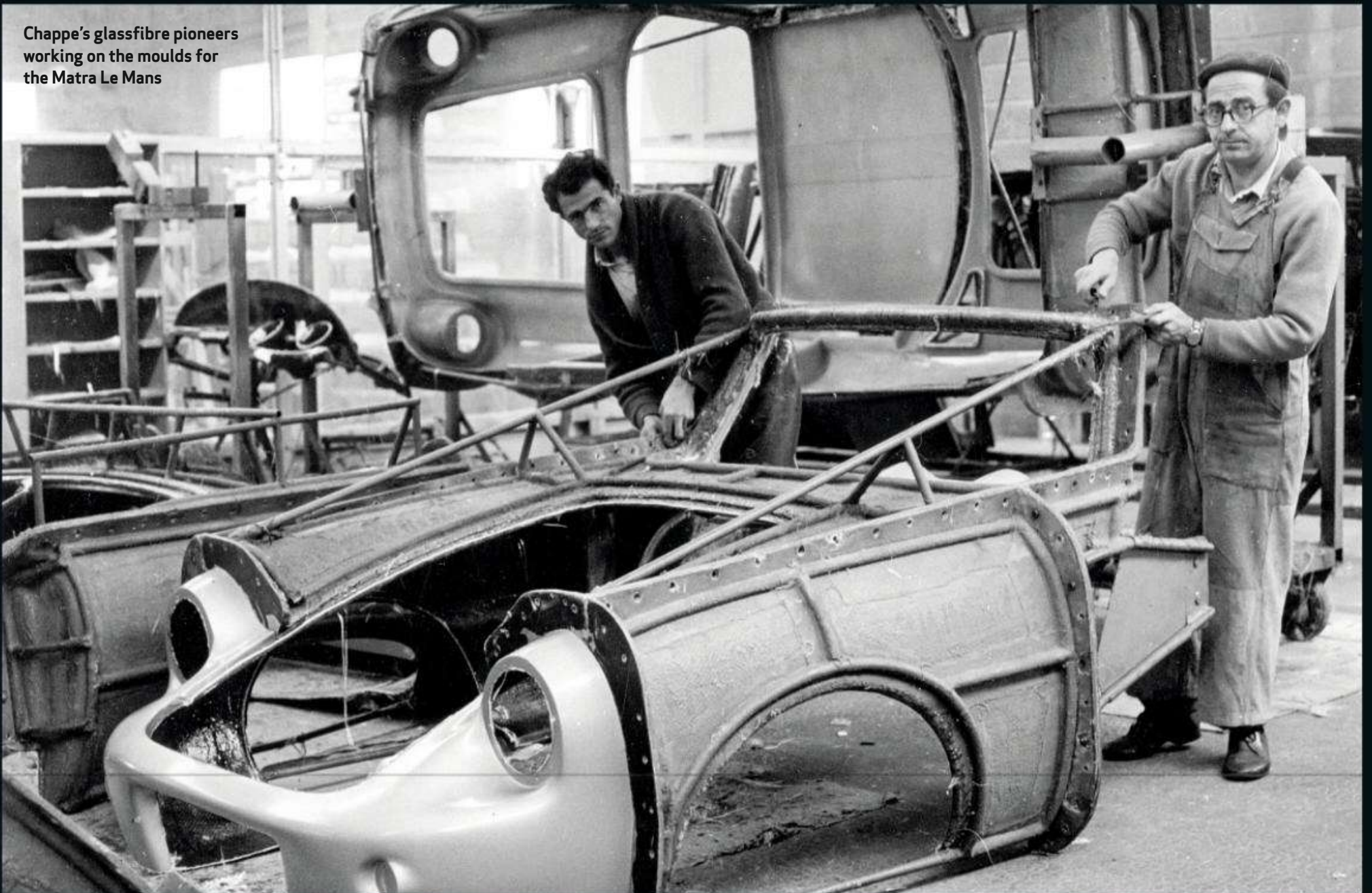
Panhard-CD prototype was steel, but production cars and Le Mans racers were glassfibre
