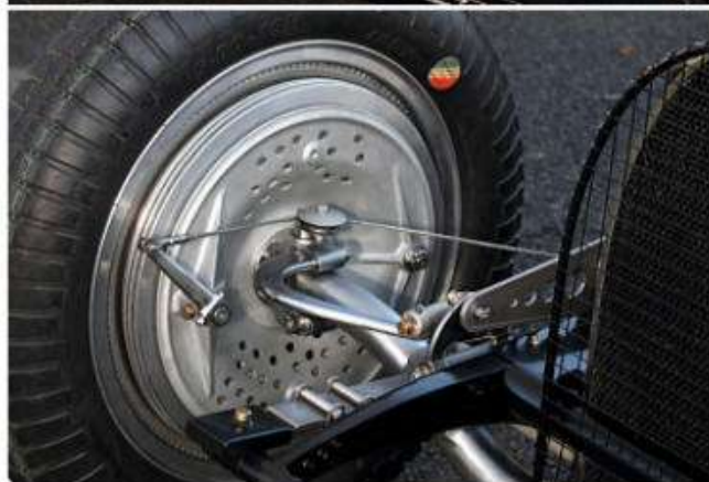
Type 59 was the last of the two-seater Grand Prix titans. Below: wider ventilated drums helped reduce brake fade
