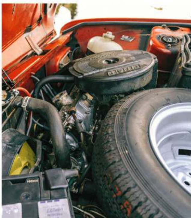
Compact overhead-cam 'four' is canted slightly forward to make room for the spare wheel under the bonnet, which results in a generous boot
