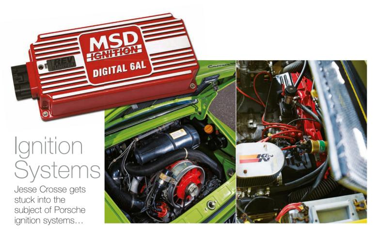
f you own an older Porsche from the 1960s or 1970s, the engine will have been fitted with a Bosch distributor and old-fashioned contact breaker points. The 356, 912 and 914 had the most basic ignition system of all - the inductive discharge system. The spark is produced by an ignition coil containing two sets of windings, primary and secondary. When connected to the car's electrical supply (12 volts in this case) current flowing through the primary coil generates a magnetic field.
