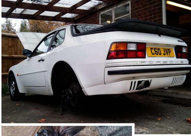
wheels off I cleaned and added a little anti-seize compound to the studs. With all the nuts installed I torqued them to the correct 130Nm (about 95lb ft).
