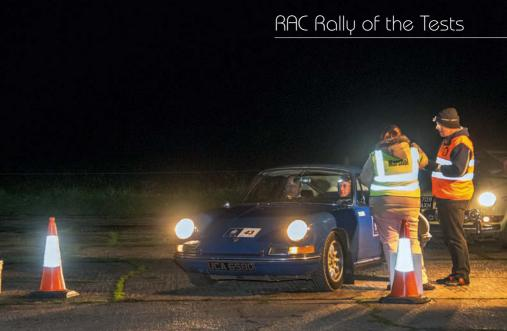
'My' machine was the least racy of the lot, toting no more than the usual carb-fed 130hp motor it would have had when new. It had standard arches, brakes and body work. Roll-cage, fire extinguisher and armour plating aside, it was standard. Even so HERO did insist on bolting a set of skinny competition-specification gravel tyres to its wheels for reasons for which I would come to be eternally grateful.
