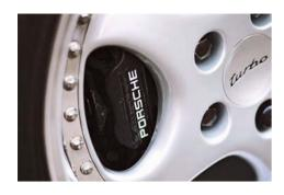
commonly known as 'teardrops'. This became one of the Turbo's signature trademarks, that was carried over to the 993 and various other models. The 17-inch wheels were based on those found on the Carrera Cup car but were made from more durable aluminium instead of porous magnesium.
