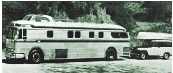
Phil Berg's fabulous land yacht Savitar was completed by Chris Bohman in 1957. Mercury Sun Valley made the observation dome on this Greyhound body.
