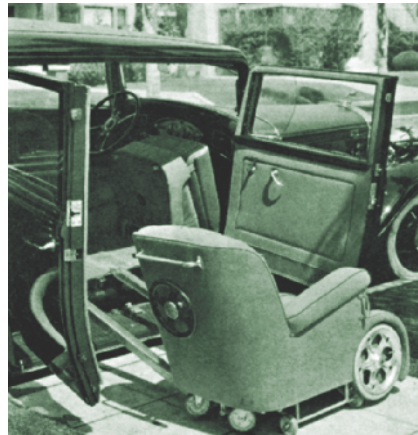
Another pillarless Lincoln, this time showing the wheel on the chair back that let down the ramp wheels.
