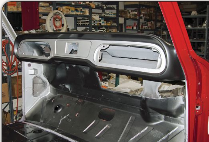
Before the exterior was painted and long before the seats, gauges, steering column and other related components were installed, the two-tone interior's metal work was thoroughly disassembled and completely refinished in black and silver urethane.
