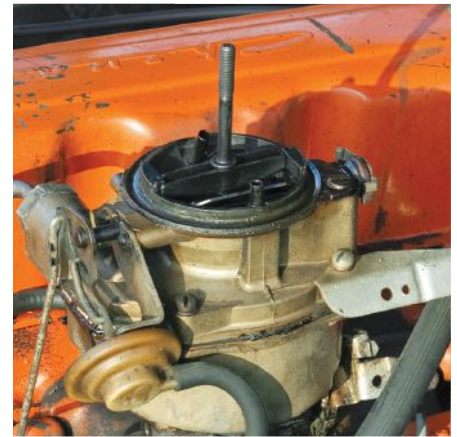
Still wearing its factory-applied orange enamel, the Hi-Thrift 194-cu.in. straight-six engine is punchy around town and relaxed on the highway with 120 hp, even with its single Rochester carb. The "300" emblem stands as an enduring symbol of the combination of thrifty economy and unique features.
