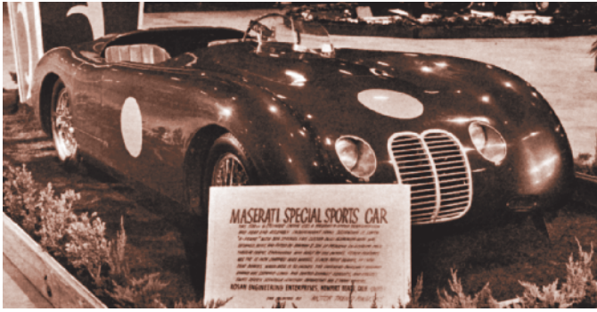
Chris Bohman, who took over his father's business in 1950, built this aluminum full-custom body on a six-cylinder Maserati chassis for Rosan Engineering.
