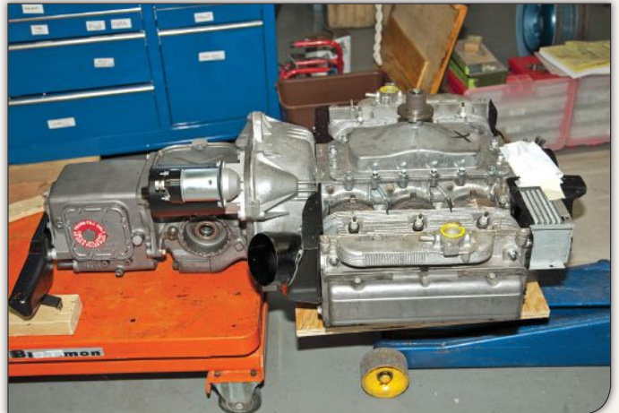
The unique Corvair driveline components—with the differential sandwiched between the four-speed transmission and air-cooled, flat-six engine—were mated together before the entire unit was installed as one under the truck's bed.
