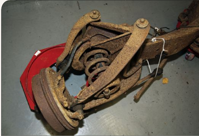
Despite pervasive rust, major parts of the front subframe, including the crossmembers and the A-arms, were salvageable, though required complete restoration. New bushings, ball joints, tie-rod ends, shocks and springs were fitted to make it new again.
