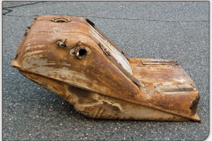
With the gas tank corroded and too far gone, and with new, reproduction tanks now available for the forward-control Corvair 95 trucks and vans, it was an easy choice to ditch the old rusty one for a shiny new one.
