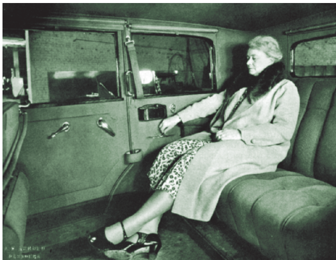
Milady had only to touch a switch near the armrest, and the rear divan slid forward electrically. Arrival at full-front position put passengers nearer the rear door. Seat mechanism used an electric motor and operated much like power front seats.
