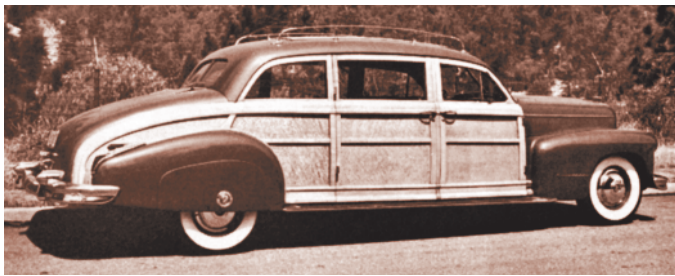
Maurice Schwartz rebuilt the Series 75 limousine for Harry Karl as a gift for his wife. Stretched trunk integrates well with rear fender.
