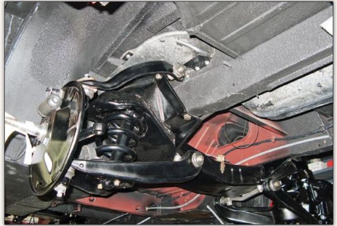
Once rusty and now shiny front subframe and suspension—a mix of restored and replacement parts—are testaments to the owner's thoroughness, which presents as well underneath as it does on top, with a stellar finish all around.
