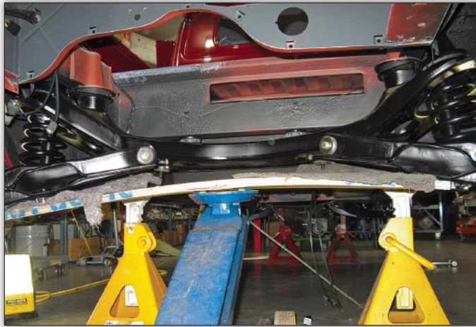
Rear subframe being lifted into place from below with a heavy-duty, four-ton floor jack. The owner prefers lifting such sub-assemblies from below, as opposed to lowering the car onto them, due to the ability to make small adjustments with a jack.
