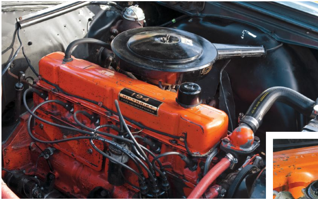
Still wearing its factory-applied orange enamel, the Hi-Thrift 194-cu.in. straight-six engine is punchy around town and relaxed on the highway with 120 hp, even with its single Rochester carb. The "300" emblem stands as an enduring symbol of the combination of thrifty economy and unique features.
