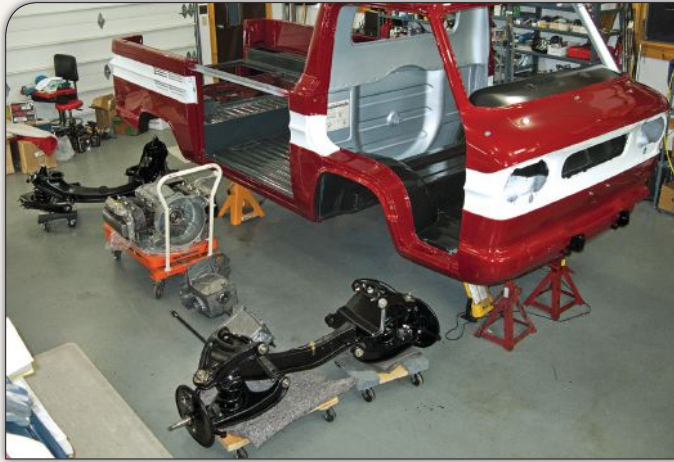
Before the interior or any glass was fitted to the finished body, the front and rear subframes and driveline were installed in the Rampside. Note the metal bar in place of the ramp door to ensure body rigidity and integrity before the door's installation.
