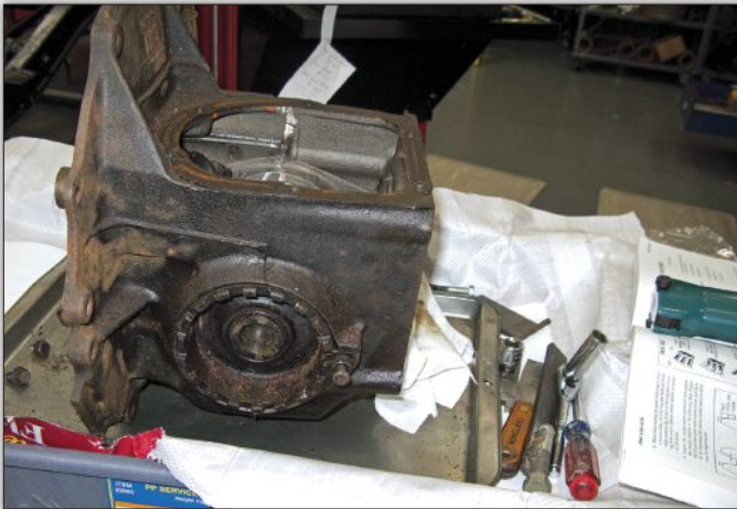
The NOS differential's lubricant also gummed up the works and required the same treatment as the transmission. The owner decided to swap out the truck's 3.89-geared differential for a sporty, but taller 3.55, an optional ratio from the coupes and sedans.
