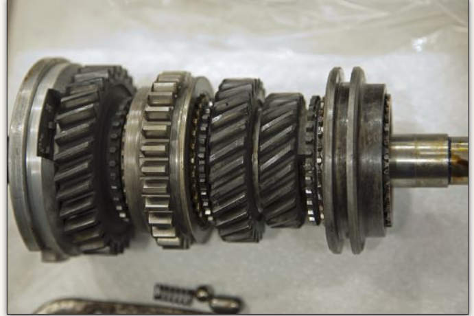
The NOS four-speed transmission—a step up from the original three-speed and an option when new—also needed a rebuild because of its decades of storage. Its lubricant, too, had hardened, and a thorough cleaning and fresh seals brought it up to snuff.
