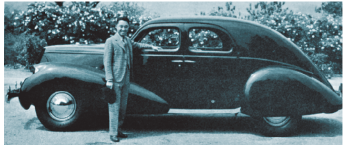
Marquis Hachisuka put a taper in the rear fenders and made them removable. He blanked in the backlite and rear windows, and recessed the headlamps.
