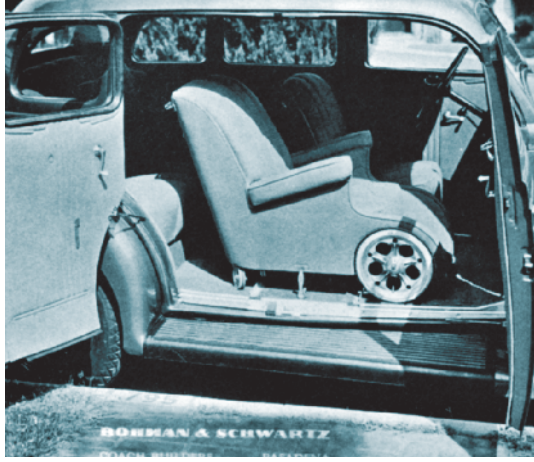
B&S did a series of wheelchair modifications, this one on a 1935 Plymouth. The center pillar was removed to make way for the chair mechanism.
