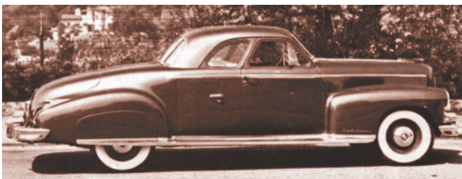
Three-passenger coupe for W. A. Woodward on a 1949 Cadillac 75 base had blended stock panels, stretched deck and golfbag doors.
