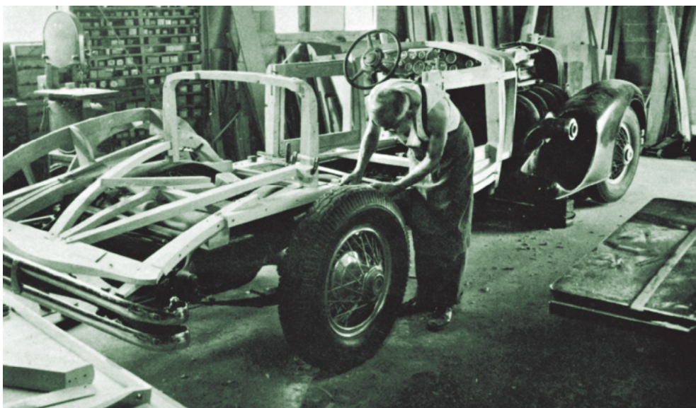
At age 70, Schwartz began to take on restoration projects for Harrah's Automobile Collection and others. Here he's shown starting to frame in a Duesenberg SJ Speedster. Photo was taken in 1959.
