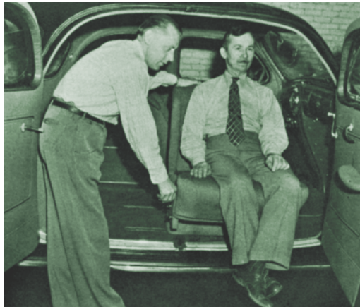
Bohman (left) and Schwartz demonstrate the pivoting passenger's seat in this pillarless Zephyr.
