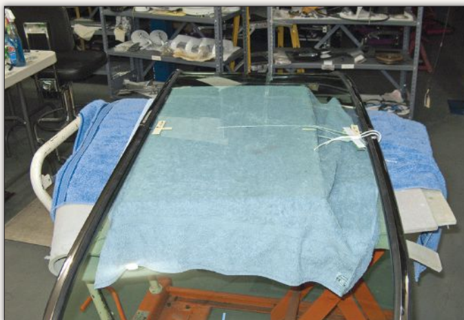
After the original had gone missing over the years, the windshield was the only piece of glass that needed to be replaced. All of the other glass pieces were treated to a fine polish to remove any minor pitting, scratches or rust streaks.
