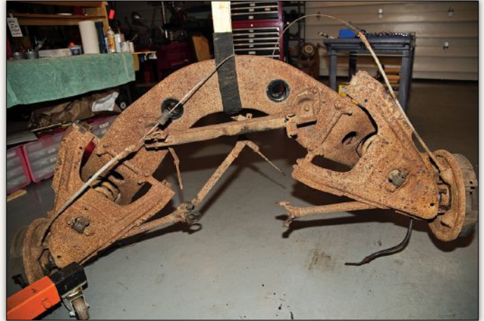
The rear subframe, yoke-shaped to accommodate the complete drivetrain mounted underneath the Rampside's load floor, also needed a complete rebuild. With no plans to use it for heavy loads, lighter-duty springs were fitted for a softer ride.
