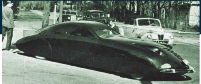
Rust Heinz's famous front-wheel drive Phantom Corsair was one of Bohman & Schwartz's greatest challenges. Its steel-and-aluminum body was handformed.
