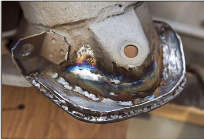
Getting subframes into better-than-new condition required heavy media blasting and rust removal before the welding in of any needed new metal. As much as possible, components were primed and finished inside and out to keep future corrosion at bay.
