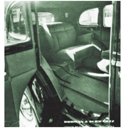
Look closely and you'll see a turntable in the rear floor that lets the chair pivot for feet-first exit.
