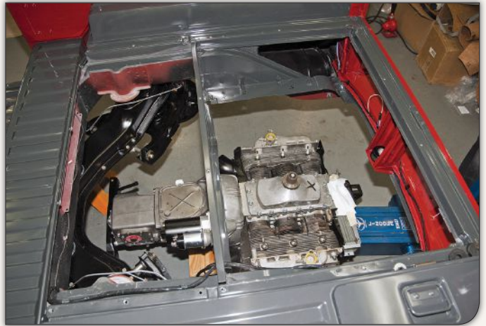
As seen from above with the service panels removed, the driveline is also installed from below with the use of a big floor jack. Note where the yoke-shaped rear subframe is curved to fit the Corvair's unique drivetrain.
