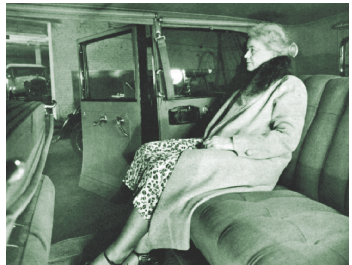
Milady had only to touch a switch near the armrest, and the rear divan slid forward electrically. Arrival at full-front position put passengers nearer the rear door. Seat mechanism used an electric motor and operated much like power front seats.
