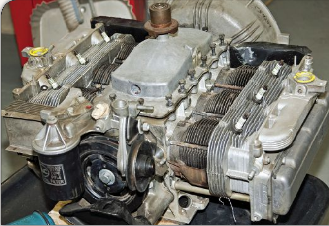
An NOS crate engine might seem like an easy swap, but 40 years of albeit dry storage left the top end in need of a rebuild due to the lubricant turning to sludge. A thorough cleaning, a fresh set of rings and a cylinder hone put it back in order.
