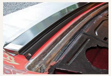
The section of the body with the worst corrosion was the area at the bottom of the rear window. It was due to water getting under the window and rotting out the metal channel. This rusted section was carefully cut out, using the replacement panel as a guide.
