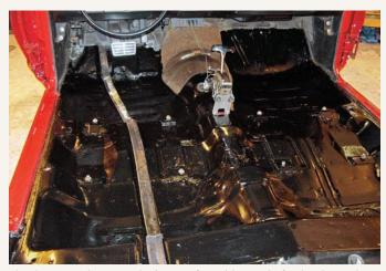
Thanks to northern Sweden's use of sand instead of salt, the entire floor pan was solid and free of any corrosion. After everything was removed, the floor was degreased, then sanded smooth before a coat of primer and a thick coat of POR-15 were applied.
