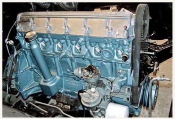
A cosmetic restoration of the original overhead-cam six engine included stripping its exterior, then priming and painting the block with several coats of the correct Pontiac Blue Metallic. The engine was not removed; rather, it was refinished in place.
