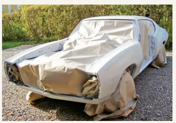
After taping off the interior and engine bay, two coats of a highbuild epoxy primer were applied, followed by a double wet-coat of primer sealer. Roger did all the priming work in his home garage in order to save money on the final refinishing process.
