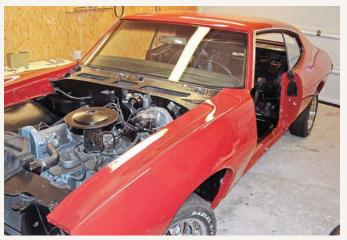
The Le Mans's top coats were sprayed with Standox Standoblue waterborne paint; three coats of base color, followed by three coats of clear. The entire body was then sanded with successive grades of paper to 2000 grade, then buffed to a brilliant shine.
