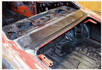
The replacement rear filler panel, which stretches between the quarter panels, was carefully trimmed to fit, then slowly MIG welded in place by a local autobody metal specialist. Fortunately, the water damage did not extend into the trunk area.
