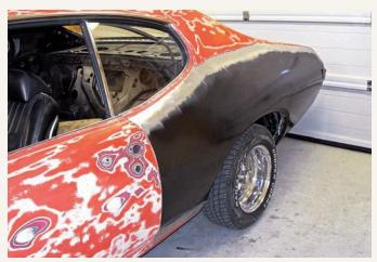
The Le Mans's body was in good shape, but ultimately, new reproduction quarter panels were installed on both sides because there was corrosion all around the rear fender lips. It cost the owner \$3,000 for the parts and labor to have them installed.
