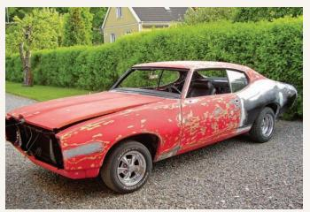
Because most of the existing paint and the condition of the body panels below were in such solid shape, the old paint wasn't stripped off, just sanded smooth after lots of block sanding. The bottom of the front fender did require a patch panel, though.
