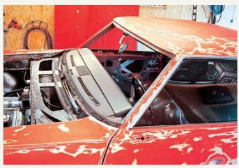
The windshield, as well as the rest of the glass, was taken out, which allowed for the removal of any surface corrosion in the windshield channel. Two coats of a rust-inhibiting primer were applied, then sealer before the final urethane topcoats.
