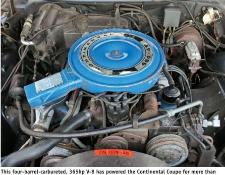
132,000 miles, and despite sitting inactive for 16 years, has never been rebuilt.
