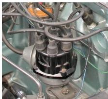
Mechanical components for old Pontiacs are easy to find, even in faraway Sweden. For an authentic appearance, original-style black ignition wires were used, along with all the correct hoses and fittings, including the original air cleaner.
