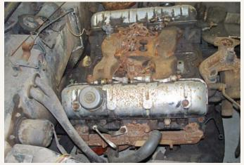
Despite the rough-looking condition of the engine, the powerplant was complete and salvageable. After minimal machining, the robust, supercharged Studebaker 289 cubic-inch V-8 was fitted with new pistons, valves, plugs, seals and bearings during the rebuild process.
