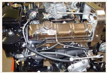
After the rebuild, the engine was almost unrecognizable as compared to when it first came into the shop. From the factory, Avanti engines had chrome-plated rocker covers, lifter cover, oil filler cap, air cleaner and voltage regulator.
