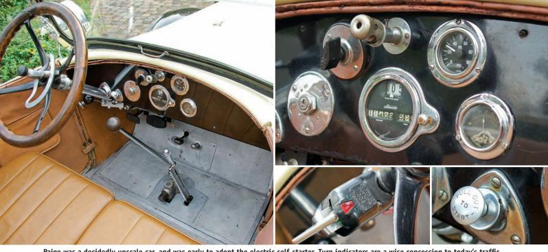
Paige was a decidedly upscale car, and was early to adopt the electric self-starter. Turn indicators are a wise concession to today's traffic volumes. Note the instrumentation lamp above the roller speedometer from Stewart. Seat leather has been only slightly updated from wear.
