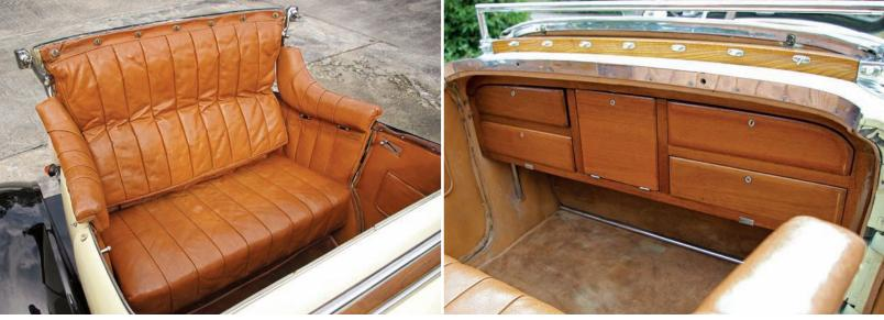
Rear seat forms half of a clamshell when lowered for the Brooklands' two-passenger version, with another panel forming a semi-tonneau. Cabinetry in the front bulkhead is fully functional and all original. So is the rear upholstery. This is the epitome of Twenties elegance.
