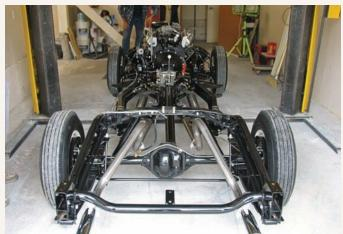
Mating the rolling chassis to the body required very careful placement and alignment underneath the completed body on the lift. Note the absolutely as-new condition of the freshly powdercoated frame, suspension and driveline components.
