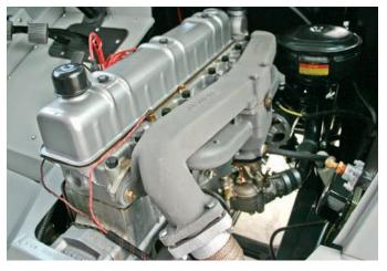
The command center of this 1951 Metro boasts a barstoollike driver's seat and a long shifter with which to shift the four-speed crashbox transmission. Instruments are minimal; these are originals restored to like-new. The Metro's engine, too, is the original, a rebuilt 220-cu.in. Silver Diamond straight-six.
