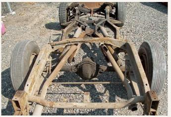
Though the chassis exhibited some surface corrosion beneath the fiberglass body, it was largely solid and intact. With its extrastrength center X-brace, the Studebaker Lark convertible chassis proved to be an ideal platform for the Avanti.
