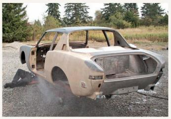
In order to return the Avanti to factory-original condition, part of the process of repairing and restoring the fiberglass body included a thorough steam cleaning, even of surfaces that might never generally see the light of day again.
