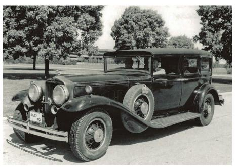
Riding a stately wheelbase that spanned 145 inches, the 1931 Stutz model MB limousine featured a body by coachbuilder LeBaron. Even this graceful machine offered road performance that was a step above the ordinary, courtesy of its DV-32 engine.
