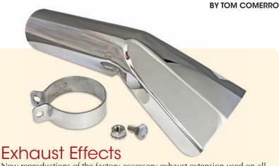
New reproductions of the factory accessory exhaust extension used on all 1937-'40 Chevrolet cars and trucks are now available from The Filling Station. This deflector has been made in stainless steel and polished to a show finish. The part is period correct at an overall length of 93/4 inches. Made for the 13/4-inch-diameter exhaust pipe, this part replaces GM accessory 985170. Cost: \$79.50.
