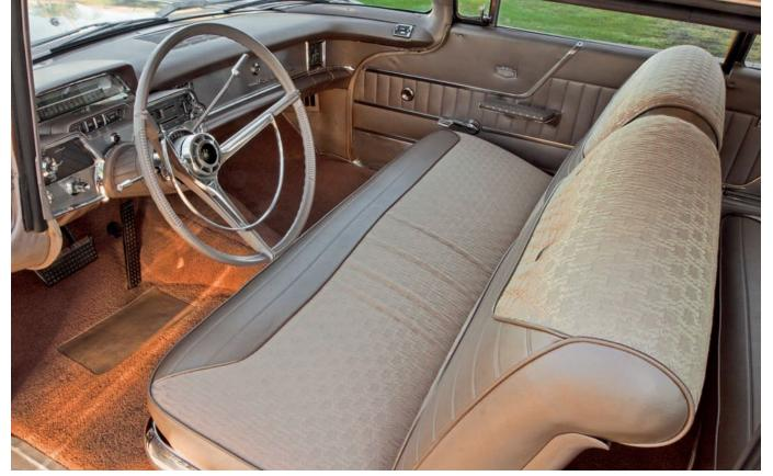
"Space planned for a new kind of comfort," opines the 1959 Mercury brochure. Indeed, the clearance hump for the transmission was reduced 45 percent, thanks to the engineers tilting the engine back and to the rear slightly; seating for six was rarely so comfortable.
