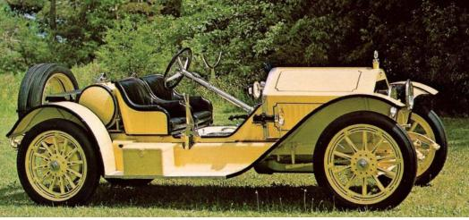
The sporty two-seat 1914 Bearcat was powered by a T-head four-cylinder, 50-horsepower engine. Stutz automobiles were targeted mainly to driving enthusiasts looking for a fast, good-looking car of distinction. It appealed to these buyers because of its outstanding racing record.
