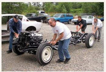
Ready to reunite the body with the frame, the crew at Avanti Northwest rolled the finished chassis, complete with engine and transmission, across the yard. Along with the powder coating, all wear items were replaced on the suspension.
