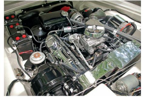
Studebaker's 280 horsepower supercharged "Jet Thrust" 289-cu.in. V-8 provided plenty of oomph for Studebaker's flagship, four-passenger GT car.
