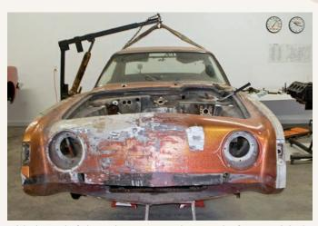
With the goal of the project to return the car to its factory-original condition, the restorer had the body removed from the chassis as part of the process of tearing the car down to its elemental components and almost starting from scratch.
