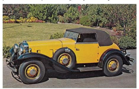
One of the last truly great automobiles from the dying Stutz Motor Car Company was the sensational and limited-production Super Bearcat roadster, which was built on a short 116inch wheelbase that provided superior handling and cornering power, plus the DV-32 engine.
