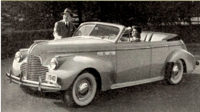
The new torpedo body shell used for the convertible coupe and convertible sedan did not make its debut for Cadillac (Series 62) and Buick (Roadmaster Series 70, Super Series 50) until March of 1940. It took six extra months to get the open-body-style dies made and to then start production.
