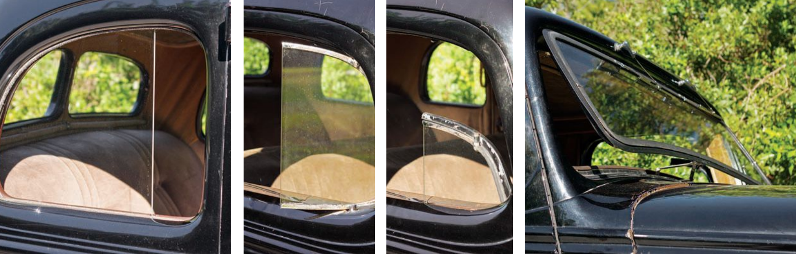
Only the De Luxe Terraplane offered such complete ventilation with its multi-position vent windows and rear quarter windows that open, too. The crank-out windshield creates excellent air flow as does the speaker-sized vent under the rear seat.
