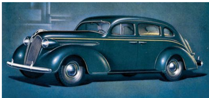
By the late 1930s, body stampings among the Chrysler Corporation line saw much interchangeability. The 1937 Dodge and Plymouths not only shared bodies, but had the same wheelbases as well.
