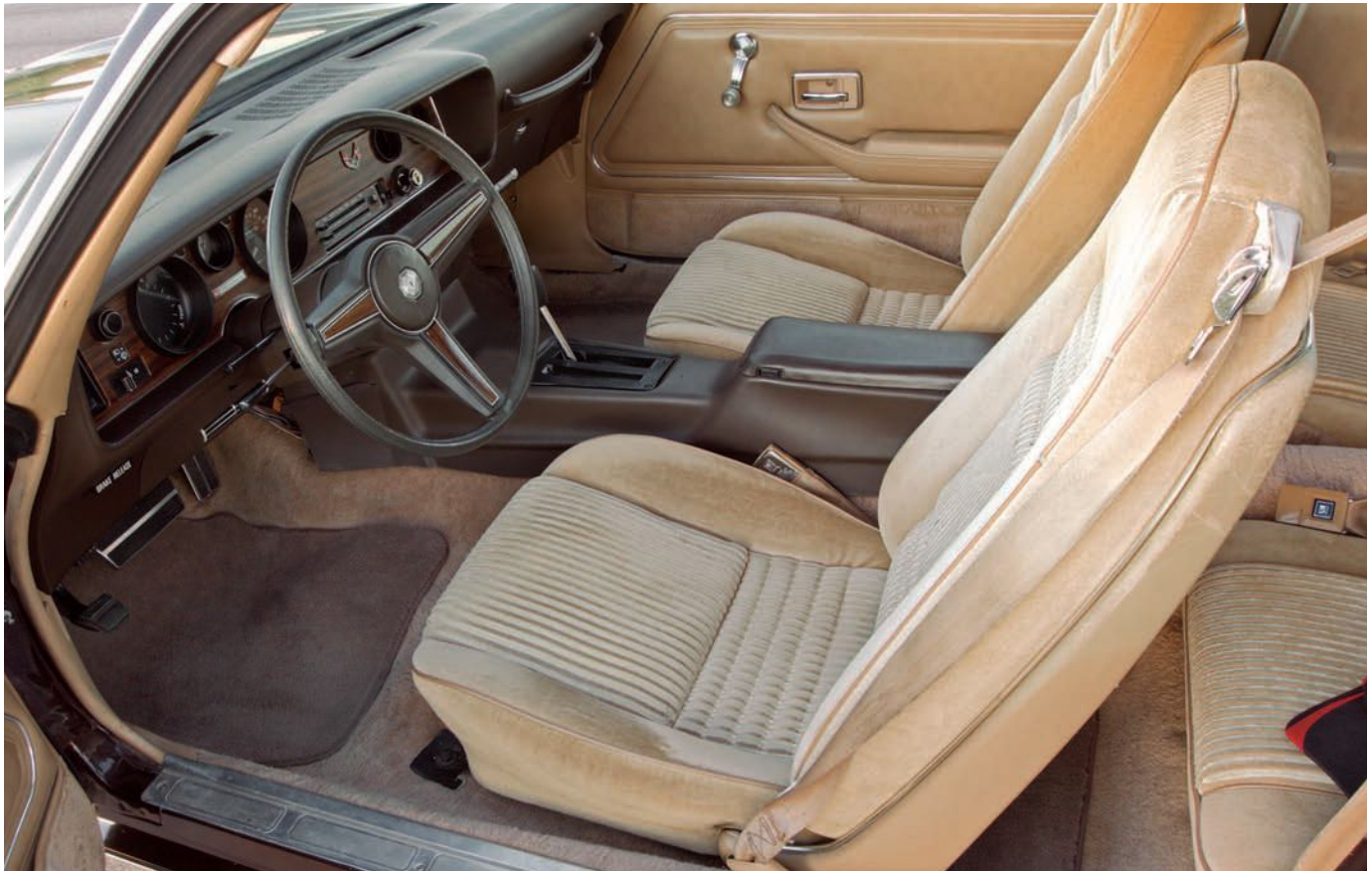
Esprit features included Custom trim with upgraded bucket seats, steering wheel and door panels; dash assist strap; bright pedal trim; color-keyed seat belts, rear ashtrays and additional acoustical insulation. Camel Tan Pimlico cloth seating surfaces were optional.
