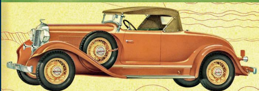
Plymouth and De Soto roadsters for 1932 shared the same body, both had the same wheelbase as well, but the Plymouth was a four-cylinder and the De Soto a six-cylinder.
