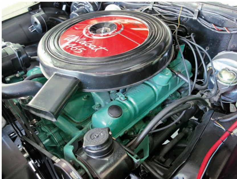
The 340hp, 425-cu.in. V-8 that was optional on 1963 Rivieras was standard in 1964. Many hours of detailing work improved the look of this engine bay.
