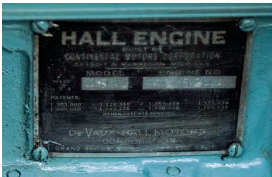
Elbert Hall redesigned the Continental 22A to create the Hall 40A, an engine used exclusively in De Vaux automobiles. With a modified block, cylinder head and intake and exhaust manifolds, the 40A made a respectable—for a light, affordable car—80 horsepower in 1932.
