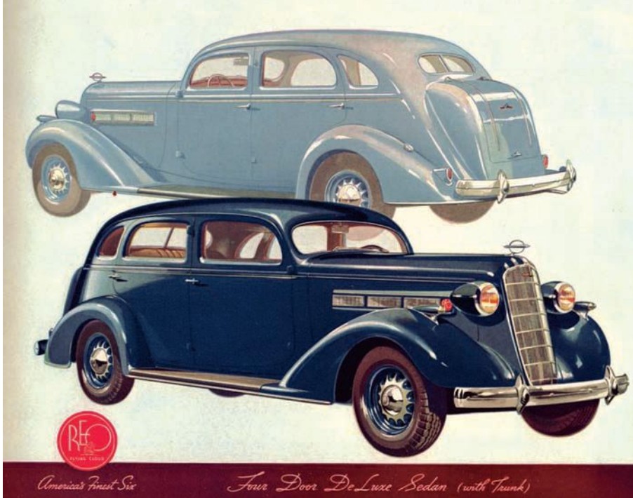
Graham and REO in 1936 used Hayes bodies that were the same stampings. REO's final year of car production was 1936, and for it, the company only offered enclosed coachwork.
