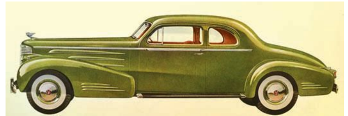
The 1938 V-16 two-passenger coupe body by Fleetwood used the same wheelbase of 141 inches as the V-8 model 75. Note the difference in the trim between the V-8 and the V-16.
