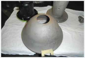
As some of the smaller subassemblies were removed from the car they were further torn down as needed and media blasted. Though it might appear minor, the process exposed extensive pitting on the exterior surface of this headlamp bezel.
