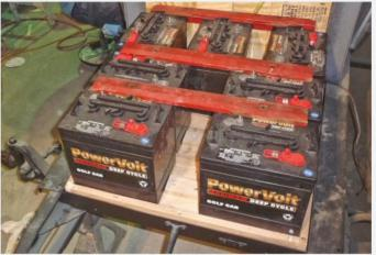
A Detroit Electric is powered by 14 six-volt batteries. Seven are located at each end of the chassis. Each of the battery trays had to be fabricated from oak using the original trays as patterns. Original clamps assist with the test-fit of the new golf cart batteries.
