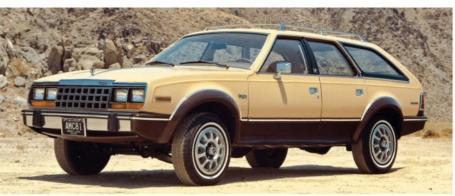
The American Motors Eagle was developed by Lunn in record time. Created by joining an AMC Concord body with Jeep four-wheel drive, the Eagle proved to be a decent seller for AMC.
