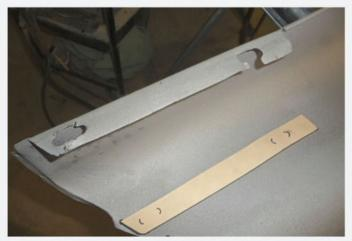
The fender mounting lips were damaged as well. This image demonstrates the value of simple card stock to experienced restorers. With the damaged lip still in place, a template was traced, cut, verified, and ready to transfer the image to new steel.
