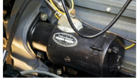
The 60hp, 194-cu.in. OHV six-cylinder engine was a refinement of the 1929 "Cast Iron Wonder." It benefitted from a new crankshaft and Carter W-1 carburetor. The generator serves a six-volt, negative-ground system.
