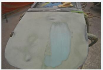
The corrective filler and glazing putty—the latter being 3M Piranha Advanced Finishing Putty—stages performed on the battery covers and doors concluded with careful sanding using 180-, and then 220-grade paper, resulting in a smooth surface.
