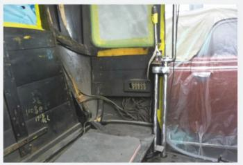
With the main body protected in epoxy primer, the rest of the interior was removed and retained to use for patterns later. Once again most of the wood was devoid of damage; however it was determined the remaining wiring would need replacing.
