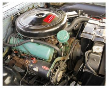
The engine compartment maintains a patina of originality. Assembly line grease pencil markings and some factory applied decals and tags are still in place. The 315hp 394-cu. in, four-barrel Rocket V-8 contains a forged-steel crankshaft and connecting rods, aluminum pistons, hydraulic lifter cam, conical valve springs, wedge-shaped combustion chambers and largeport intake and exhaust manifolds.
