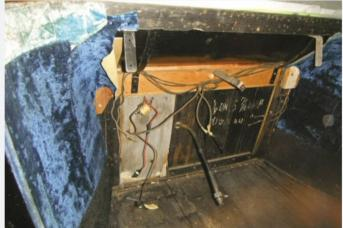
With the jumpseat and its mechanism removed, access to the Detroit Electric's wooden firewall was now unimpeded. With the exception of one panel, damage was nonexistent. Forward wiring would need replacing and the instrument panel was missing entirely.
