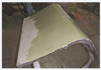
The next step was a coat of glazing putty. This extra process fills in any of the barely perceivable pin holes and fine scratches. According to the restorer, this is a point in time at which it appears to owners as though little work has been done.
