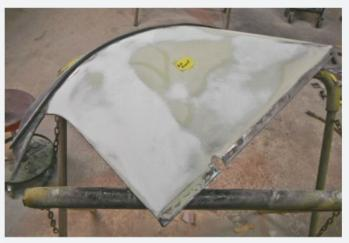
Once all of the patch panel seams had been MIG welded, and the welds ground smooth, each of the fenders were treated to the aforementioned body filler process in sections, concluding several weeks of painstaking effort.
