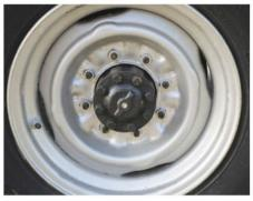
The truck's 16-inch eight-lug wheels are one-piece units now, but it was originally delivered with 16-inch split rims.
