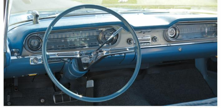
The instrument panel and De Luxe Safety-Vee steering wheel designs were revised. A Guide-Matic Power Headlight Control is on the dash.
