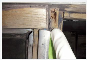
To the relief of both the Detroit Electric's owner and restoration team, wood exposed to decades of varying weather was found to be essentially devoid of rot. The few trouble areas that were discovered were small, as demonstrated here, and easily manageable.
