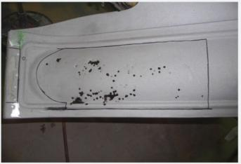
Metal repair might seem straightforward but, when dealing with compound curves, it's always best to map out a specific area to be rectified. Before cutting, the area then serves as a static template to assist the fabrication of a patch panel.
