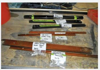
With multiple projects underway at the shop, organization was—and should always be—a critical part of the process. Here interior trim has been properly labelled while its corresponding hardware has been documented and secured in plastic bags.
