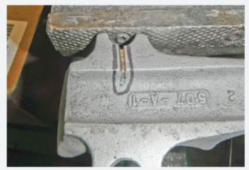
Little details can delay projects. In this case the team uncovered surface stress fractures in the rear bumper brackets during media blasting. Unobtainable and costly to cast, the cracks were ground out and later filled with weld, then filed smooth.
