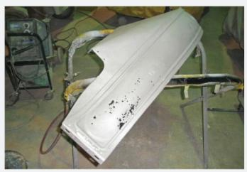
Media blasting the steel fenders uncovered both a high level of corrosion and an array of prior repairs with body filler, the latter visible along the runningboard mating edge. The fenders were also dimpled in several areas.
