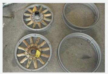
Not to be forgotten were the Detroit Electric's wooden artillery-style wheels. A special tool was required to separate these two-piece subassemblies, which had also been media blasted. Fortunately, again, the wood was unaffected by exposure to elements.
