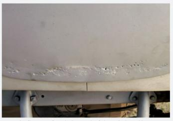
Due to its flatter surface design, each of the car's door skins were stamped from steel at the factory. Prior repairs and new corrosion were exposed, adding to the team's list of repair needs. Note the lighter hue of the aluminum panels versus steel.
