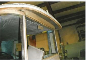
As instructed, media blasting also removed paint from factoryexposed wood. The interior portions of the window frames would be sanded at a later date to remove as much paint as possible. Of note: the front glass had been removed by a previous owner.
