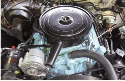
Mighty 389-cu.in. V-8 puts out a torque-laden 303hp; power steering and brakes and air-conditioning were optional, but alternator came standard with air-conditioning-equipped cars.
