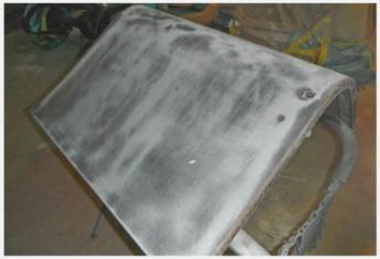
Following the initial epoxy primer/sealer, a skim coat of Rage Gold body filler was applied and dusted with a feather coat of black paint, the latter of which would help easily differentiate the high and low spots on the panel during block sanding.
