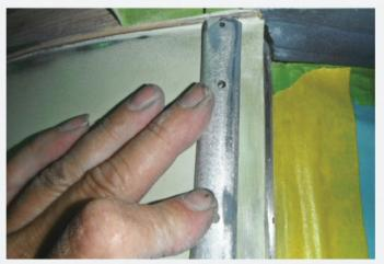
Some noticeable gaps existed between the main body and trim pieces. Here the trim is removed to prepare the main panel for primer and then test fit to confirm tolerances. Join us next month for the second installment of the Detroit Electric's restoration.
