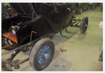
After amassing a list of needs during the car's initial evaluation upon delivery, the Coastal Classics team was ready to start the restoration. Disassembly began with the removal of the bumpers, all four fenders and the associated running boards.
