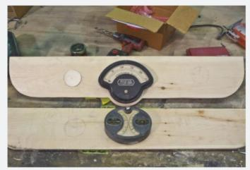
With the original instrument panel missing, the team had to begin the painstaking process of fabricating a new one. This was accomplished by studying the panel bracket position and bolt pattern, interior dimensions and images from period literature.
