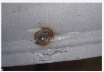
There were several small, randomly-spaced pin holes in each of the fenders. Media blasting not only removed the paint and exposed the damage, it stripped away all of the corrosion enabling the team to MIG weld the holes shut.
