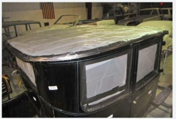
While fender repairs had commenced, the car's body was prepared for media blasting by covering the original glass. So, too, was the leatherette top, believed to be a prior replacement that merely needed to be detailed, saving time and expense.
