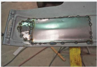
While work was underway on other parts of the body, fender repairs were still ongoing. This image shows a patch panel secured with tack welds, which helps prevent both the patch and fender from warping. Additional tacks will be applied until the seam is completely filled.
