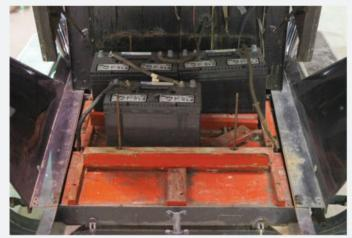
In order to make the Detroit Electric functional, a previous owner installed incorrect and oversized 12-volt batteries. Though drivable, it was clear that the alteration only accelerated the damage to both the front and rear wooden battery trays.
