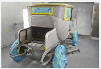
After media blasting and a second evaluation, the body shell and chassis, as well as all of the body panels, were carefully prepared to receive a protective application of epoxy primer. The primer was allowed to cure before work progressed.
