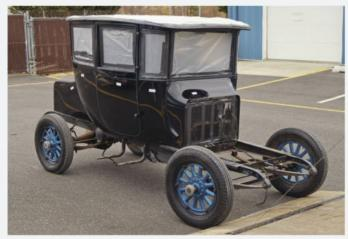
The Detroit Electric's body and chassis is ready for media blasting. Because the body is made from a combination of steel and aluminum over wood framing, heat generated during the process could warp the softer aluminum quickly, thus the cautionary labels.
