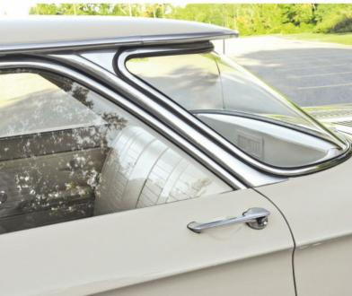
Fold-down rear seat boosts interior carrying space and was a popular Corvair option. Corvair was the last General Motors car to utilize the flattop roofline, with its complex wraparound glass and extended sheetmetal roof panel.
