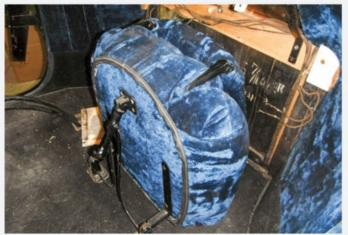
Although the forward folding jumpseat had fluid movement, a prior restoration left it shod with an incorrect and terribly dated blue crushed velour upholstery. The seat springs within had also lost their ability to support weight.
