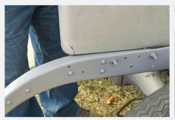
Though aluminum is easier to form and doesn't rust, its light weight and softer composition makes it more susceptible to other forms of damage. In several locations the metal had either been punctured or, in this photograph, had fractured.
