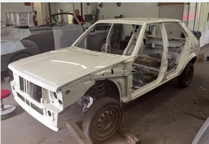
Spinnaker White replaced Chianti Red for the exterior. To facilitate the color change, the body was painted while disassembled. The shop would then bolt on the hood, doors, fenders, and hatch, properly align them, and install the front and rear glass.
