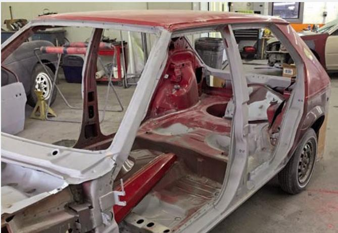
During teardown, a serious rust issue was revealed at the driver's-side rear shock mount. At Ray Donch Body Werks' request, the door jambs were sanded to ease refinishing, and the shop would then sand the rest of the body bare.
