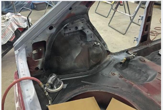
To ensure the Horizon was structurally sound before work continued, the rear shock mount area was repaired first. Its rusted portion was cut out, the surrounding metal was cleaned, and then a rust-free replacement panel from a donor car was MIG welded in.
