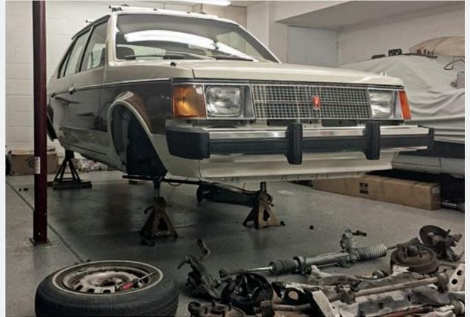
After the body and interior were finished, work began on the chassis. The wheels, brake system, anti-roll bar, front suspension, component crossmember, and steering rack were removed. Some of these parts were restored, but the wear items were replaced.
