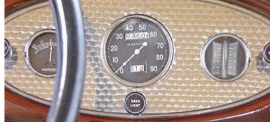
The 90-mph speedometer was common to late Model B's and V-8s. Flanking it are an ammeter and fuel gauge, along with a hand throttle, dash light, and choke.
