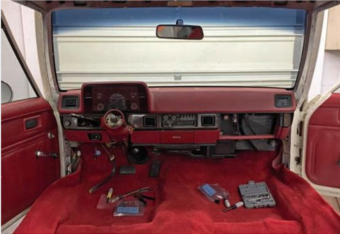
The dashboard and door panels are original, and the carpet is new. Though not installed yet here, the headliner and the front buckets and rear seat were professionally recovered with NOS material by Rich's Auto Upholstery in Gibsonia.
