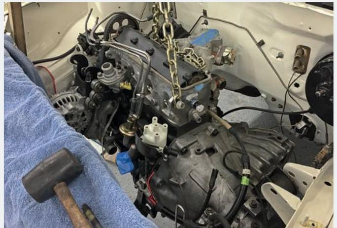
To avoid damaging the paint, the Horizon was perched on jackstands, and the rebuilt engine with the automatic transaxle was slid under the front of the car and then lifted into the tight engine bay and secured to the mounts. The chassis parts were then bolted in.
