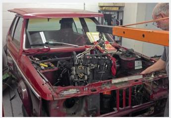
Robert and his uncle Paul inspected the non-running Volkswagen 1.7-liter engine to diagnose its issues. Under the previous owner's care, a catastrophic engine failure resulted in multiple holes in the block. Paul removes the ailing engine with a hoist.
