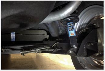
Most of the rear suspension components were also refinished with Nason SelectPrime 2K and Nason Chassis Black. NOS natural steel backing plates coated with Cosmoline and the brake drums were used. Note the Mopar decal.
