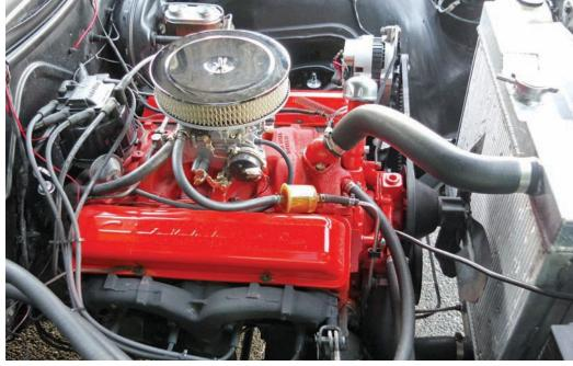
This 283-cu.in. V-8 has not needed major repair, although it's enjoyed new paint and, for reliability, the replacement of its carburetor, radiator, and distributor.
