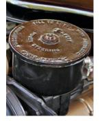
A hallmark of the new-to-the-model-year 371-cu.in. J-2 engine option—aside from the identifying decal—is the unique air cleaner assembly with dual offset air induction filters that funnel air into a trio of Rochester two-barrel carburetors. Power steering was standard equipment in the 98 Series (above).
