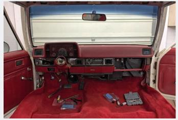
The dashboard and door panels are original, and the carpet is new. Though not installed yet here, the headliner and the front buckets and rear seat were professionally recovered with NOS material by Rich's Auto Upholstery in Gibsonia.
