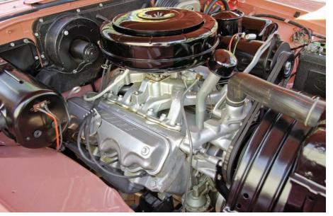
Recognizable by the scalloped valve covers, Chrysler's 331-cu.in. Spitfire polyspheric V-8 engine from 1956 never made the headlines the way the Hemi V-8 did.
