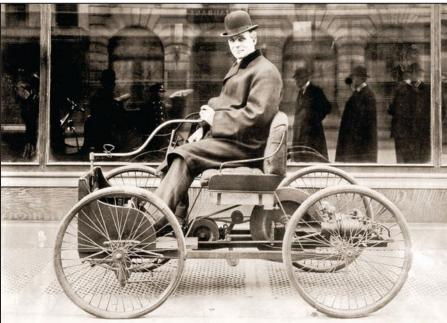
**HENRY FORD'S QUADRICYCLE RUNS ON FOUR BICYCLE WHEELS AND A TWO-CYLINDER**, rear-mounted engine capable of propelling the vehicle at around 20 miles per hour. Ford debuted the Quadricycle on June 4, 1896, and it was indeed able to attain the 20-mile-per-hour mark. The 32-year-old inventor intends to make more Quadricycles in the future.
