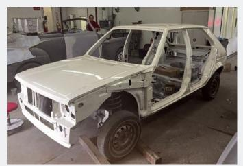
Spinnaker White replaced Chianti Red for the exterior. To facilitate the color change, the body was painted while disassembled. The shop would then bolt on the hood, doors, fenders, and hatch, properly align them, and install the front and rear glass.
