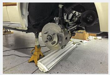
Up front, NOS MacPherson struts (with the parts decal still in place), steering knuckles, hubs, CV-style drive shaft assemblies and disc brakes were bolted in, and new lines and hoses were employed. Single-piston calipers squeeze the pads against rotors.
