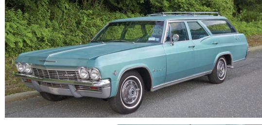
cessories like a four-barrel-carbureted 283 cu.in. V-8 (\$95), AM radio (\$50), and roof luggage carrier (\$43). That first upgrade replaced the standard overhead-valve V-8's Rochester two-barrel carburetor and offered an additional 25 hp and 10 lb-ft of torque, for a total of 220 hp at 4,800 rpm and 295 lb-ft of torque at 3,200 rpm.
