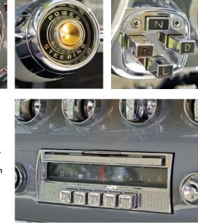
updated Spitfire engine. At 331 cubic inches, it featured the same bore and stroke as the previous year's Hemi, but produced 225 horsepower and made do with a compression ratio increased to 8.5:1. In other mechanical news for 1956, Chrysler introduced its pushbutton transmission control, a purely mechanical innovation that the company used in some models as late as 1964.
