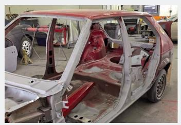
During teardown, a serious rust issue was revealed at the driver'sside rear shock mount. At Ray Donch Body Werks' request, the door jambs were sandblasted to ease refinishing, and the shop would then sand the rest of the body bare.
