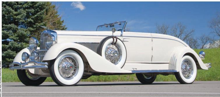
A second owner had the LeBaron body on this 1933 Duesenberg Model J replaced by a disappearing-top convertible coupe body by Bohman & Schwartz.
