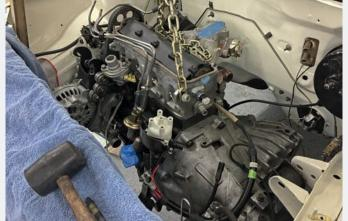
To avoid damaging the paint, the Horizon was perched on jackstands, and the rebuilt engine with the automatic transaxle was slid under the front of the car and then lifted into the tight engine bay and secured to the mounts. The chassis parts were then bolted in.
