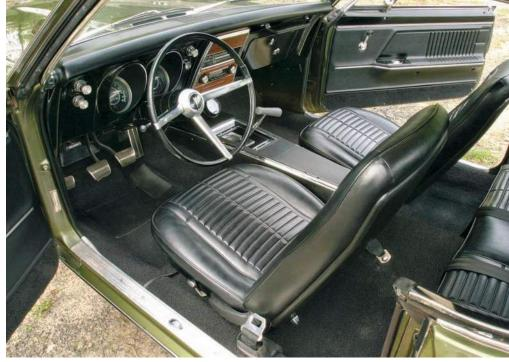
Though much of the interior was essentially unchanged from the Camaro, the seat upholstery pattern, steering wheel, woodgrain center panel, and passenger-assist grip were Pontiac specific. The extra-cost Custom trim is shown, as is an optional clock. (The T-handle shifter isn't stock.)
