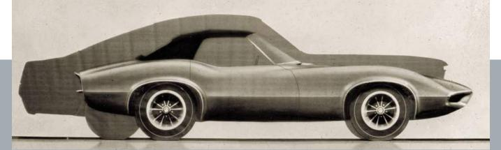
Designed and engineered to be significantly smaller and cheaper than the Corvette, but comparably quick, Pontiac's two-seat XP-833 fiberglass-bodied sports car appeared to pose a threat to Chevrolet's sports car. Assistant Chief Engineer Bill Collins formulated a proposal that aimed the XP-833 squarely at the Mustang, but GM's management still didn't approve it.
