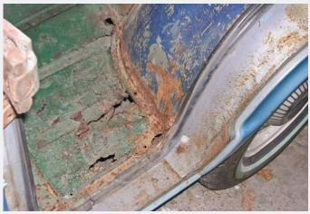
Even before sandblasting, the stability of the driver's-side floorboard is clearly completely compromised; a condition repeated on the front passenger side of the Greenbrier, due, in part, to its watercatching design and wheel proximity.
