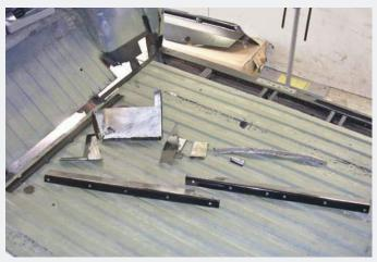
Self-etching primer was applied to metal left bare from sandblasting to protect it from flash-rusting while repairs were made to damaged sections. Here, nearly a dozen fabricated patch panels are set out, ready to be MIG-welded.
