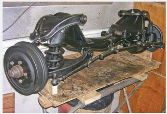
Both the front and rear suspension systems were removed from the chassis as subassemblies. Each was then broken down into individual components, painted, and carefully rebuilt. This is the completed front suspension assembly ready for installation.
