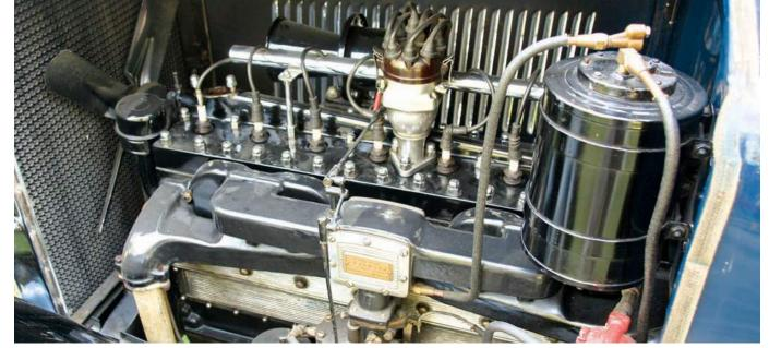
An eight-cylinder engine was unusual for a car in the mid-price field in 1925, and the Rickenbacker's is particularly stout, with nine main bearings. The 268-cu.in. engine produces 80 horsepower. By 1927, a twin-carb version would make 90 horsepower.
