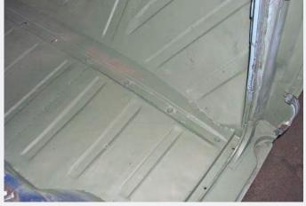
This is the view of a completed repair to the front passenger floorpan. The fabrication work included duplicating the factory bolt patterns. A final layer of self-etching primer helped seal the new and original metal until paint could be applied later.
