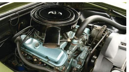
This original, low-mileage 326 H.O. engine features a Carter AFB carburetor, standard log manifolds, and dual exhaust with a crossflow muffler.
