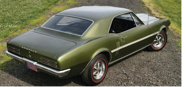
From the rear, the Firebird differed from the Camaro in the taillamp, bumper and fuel door designs, the model and automaker ID, and the louvers on the rear quarter panels. The H.O. received the side stripe, and the Rally II wheels were optional.
