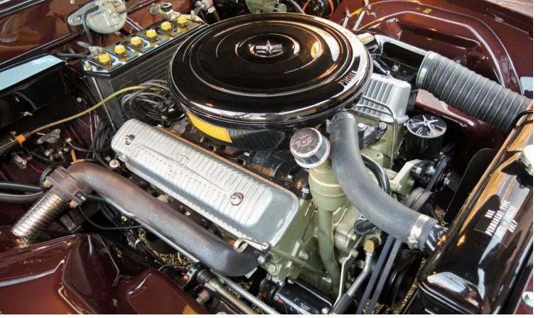
Lincoln extensively upgraded and modified its V-8 engine for 1956. Displacing 368-cu.in. and sporting a 9.0:1 compression ratio, the powerplant breathed through a Holley four-barrel carburetor to produce 285 horsepower and 402 lb-ft of torque.
