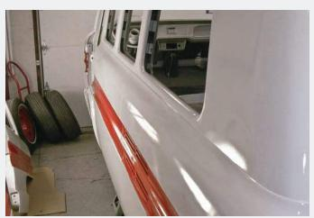
Rather than retain the original dark blue/light blue two-tone scheme, Cameo White and Cardinal Red were chosen. A PPGbasecoat/clearcoat system was used, consisting of two color coats and four applications of clearcoat. Sanding and polishing followed.
