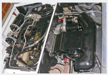
In this image, the engine bay has been painted Cameo White, and both the re-detailed 164-cu.in., air-cooled six-cylinder and the transaxle have been reunited to the chassis. Interestingly, the block is from a passenger car and did not require a rebuild.
