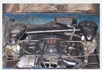
Removing the interior seating, inner side panels, and the rear engine cover allowed for a complete visual inspection. Several areas of rust could already be seen; however, sandblasting that was scheduled to occur exposed far more corrosion.
