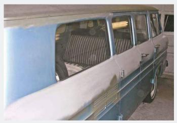
The first part of the restoration to be accomplished was the elimination of surface rust on the upper sections of the body, roof, and within the rain rails. Corrosion was removed via sanding, and the metal was quickly sealed in self-etching primer.
