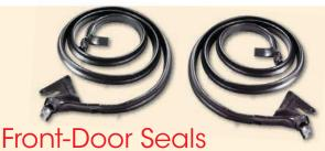
New front-door seals have just been released for General Motors' 1965-'66 B- and C-body four-door hardtop models. Made of a soft sponge-rubber compound, the seals will keep out moisture and excessive sound. The rubber features microcell technology, which provides even compression along the entire seal so you don't have to slam the doors to shut them. Each seal comes with sturdy nylon mounting pins, which are properly spaced for quick and easy installation. Cost: \$99.95/pair.
