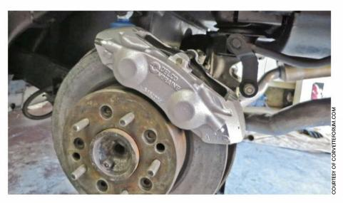
tested brake calipers with pads installed, ready to bolt on axles at the assembly plants. The calipers for each body line were assembled in a dedicated room on the pallets of a continuous oval conveyor line; Corvette had its own room.
