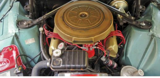
Limited use led to the 300-hp, 390-cu.in. V-8 developing many fluid leaks, which were quelled by installing new gaskets. This engine, and Cruise-O-Matic automatic transmission, were later completely rebuilt. A front disc-brake/dual-master-cylinder conversion was performed for added safety in modern traffic, the switch to high-performance ignition wires and coil was made, and the car now rides on Granada wheels.
