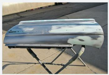
After fabrication work had been completed, the restoration team applied a skim coat of filler on each of the body panels where needed. The material was then sanded smooth, with special care taken to maintain factory body lines during the intensive process.
