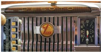
The instrument panel is a feast for the eyes. It's one of the finest-crafted and nicest-detailed dashboards ever seen in an American production car. All the necessary gauges are included; the vertical radio sits on the left side of the chrome speaker grille, with a clock on the right.
