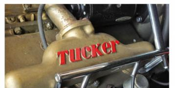
The originally planned low-revving, massive 589-cu.in. engine was replaced early on with a Franklin flatsix engine originally designed for helicopters and significantly reengineered by Tucker to accommodate water cooling. Despite the odd engine, Tucker used a thoroughly conventional 6-volt, positive-ground electrical system and battery/coil ignition. Dual exhaust pipes split to six tips to hint at cylinder count.
