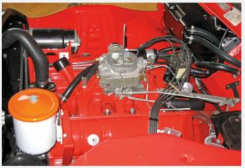
In many instances, bolt-on items—such as spark-plug wires and the carburetors—are secured to the engine after the latter has been reunited with the chassis. Accessory brackets, radiator, heater hoses, and throttle-linkage connections are also finalized.
