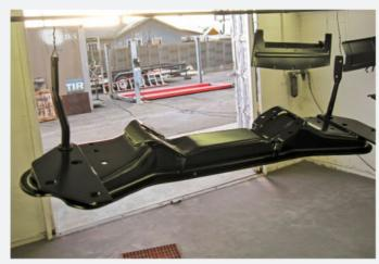
Receiving equal time in the paint booth were the Nash's suspension and other associated chassis parts, including this front crossmember. Each piece was media blasted, inspected, sealed in primer, and then — as seen here — finished in chassis-black enamel.
