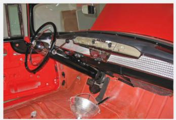
Reassembly of the hardtop's interior began with the installation of the completed instrument panel, steering column, and pedal assemblies. Hidden from view is a new wiring harness. Note that the owner resisted adding air conditioning from the parts car.
