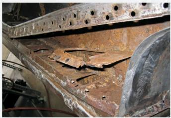
After disassembly, the body was mounted to a rotisserie, which provided easy access to every surface of the unit-body Nash for the restoration team. This included the underside, where some corrosion within and near the rocker panels was found.
