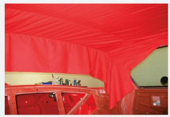
While it may seem easier to begin installing new upholstery with door- and side-panel assemblies, the best method is to begin with hanging the headliner, as seen here. The top-down method enables all seams to be hidden by the lower panels with less effort.
