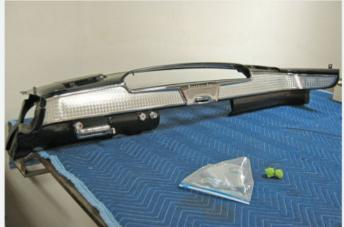
As we've outlined in other restoration features, many components are restored as sub-assemblies, such as the dashboard here. The 1957 Ambassador Custom Country Club's dash featured an engineturned insert, which was carefully restored and installed.
