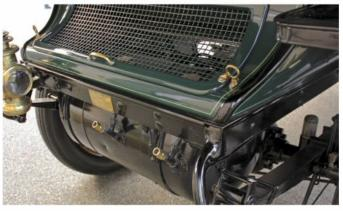
The fuel tank must be pressurized before it can feed gasoline to a pre-heated vaporizer to fuel the boiler and make steam.
