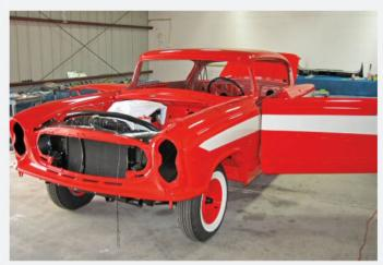
At this stage, the body has received its finish coat of Mardi Gras Red trimmed with Frost white paint. The car's suspension, engine, transmission, and remaining driveline system have been reinstalled, while the doors have been hung and balanced.
