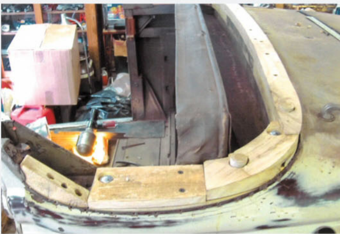
Wood was still an integral part of the Buick's body structure, which typically deteriorates in open cars at an accelerated rate. Damage caused by exposure to the elements seemed to be minimal; only the upper foundation for the folding top needed to be rebuilt.
