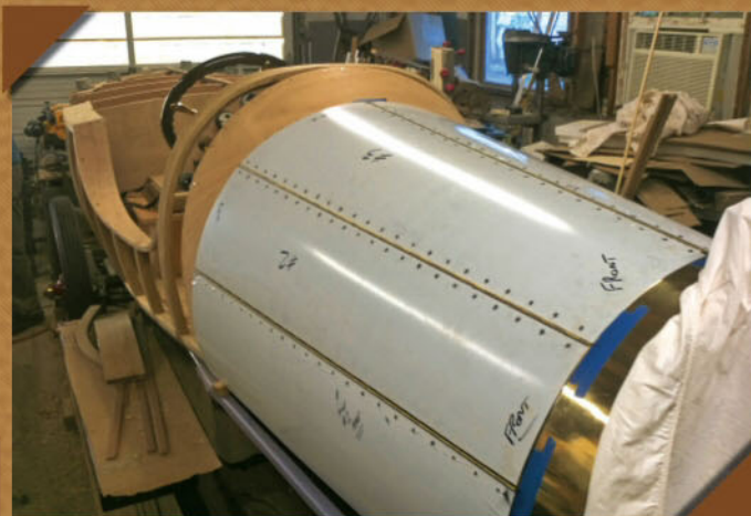
Artisans at Craft-Tech fabricated this six-panel bonnet from polished stainless steel that's coated to retain its luster. Aircraft-quality, pressed-in rivets secure 5-foot-long solid brass hinges with one-inch knuckles, identical to the movie car's.
