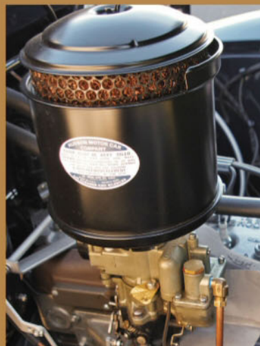
The flathead straight-six engine displaces 175 cubic inches and produces 92 horsepower; all the various instructional stickers have been accurately replicated; large air-cleaner assembly sits atop the single downdraft Carter carburetor; forward-tilting hood provides unrestricted access to the entire engine bay.
