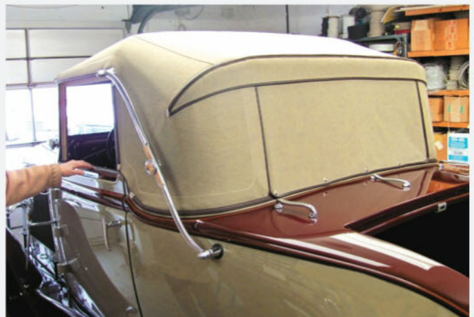
The Cabriolet is now just days away from completion, with a new top having just been fitted in conjunction with chrome trim. All that's left are the installation of the conspicuously absent rear window, and final adjustments.
