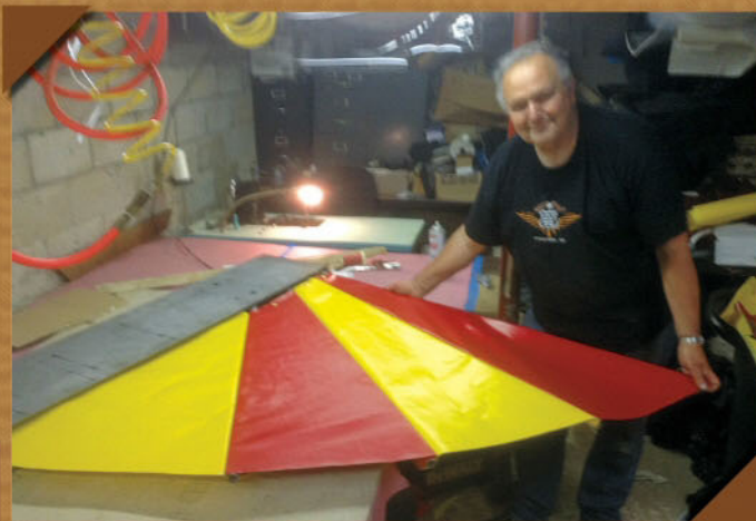
Chitty's colorful vinyl wingspans were carefully sewn by Tony's friend, Bill Webb of Boat Tops in Mastic Beach, New York; they electrically extend from, and retract into, hinge-opening boxes Tony made in rustproof 1/16-inch galvanized sheetmetal.
