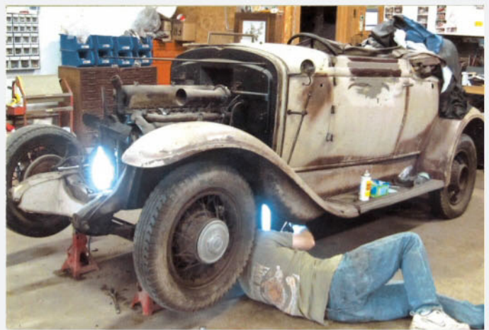
Once the wooden body framing had been meticulously restored, final disassembly could commence. With the Buick up on jackstands, any links to the lower half of the engine and transmission were disconnected, as were the brake and steering systems.
