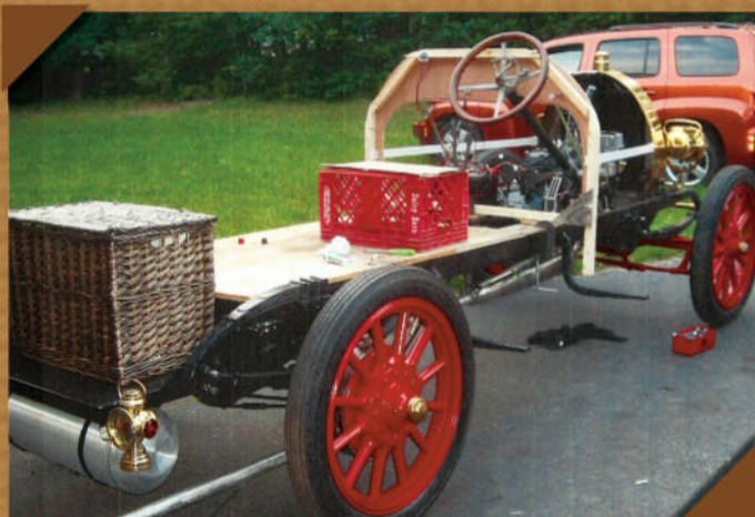
With the fuel tank and picnic hamper in the extended part of the rolling chassis, Tony used a milk crate to figure the approximate height of the front seat and body center-line. A loose oil-return line left a puddle on the driveway on first start-up.
