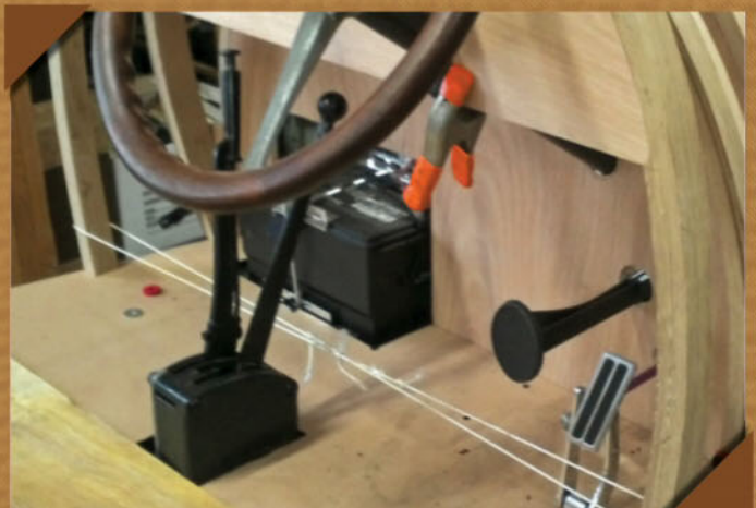
The curved "crossbows" of the cowl frame are visible in this photo, which shows two of three pedals being positioned in relation to the seat, shifter, and wheel. Tony mounted the battery with interior access, under a removable cover, for ease of use.
