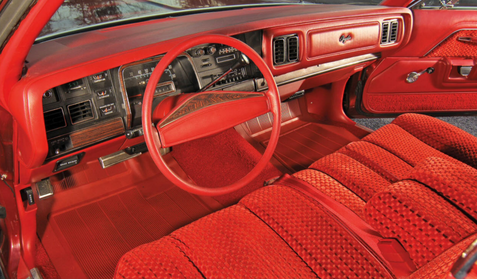
The optional cloth-upholstered 50/50 split bench seat features separate controls for driver and passenger, and the passenger seatback reclines.
