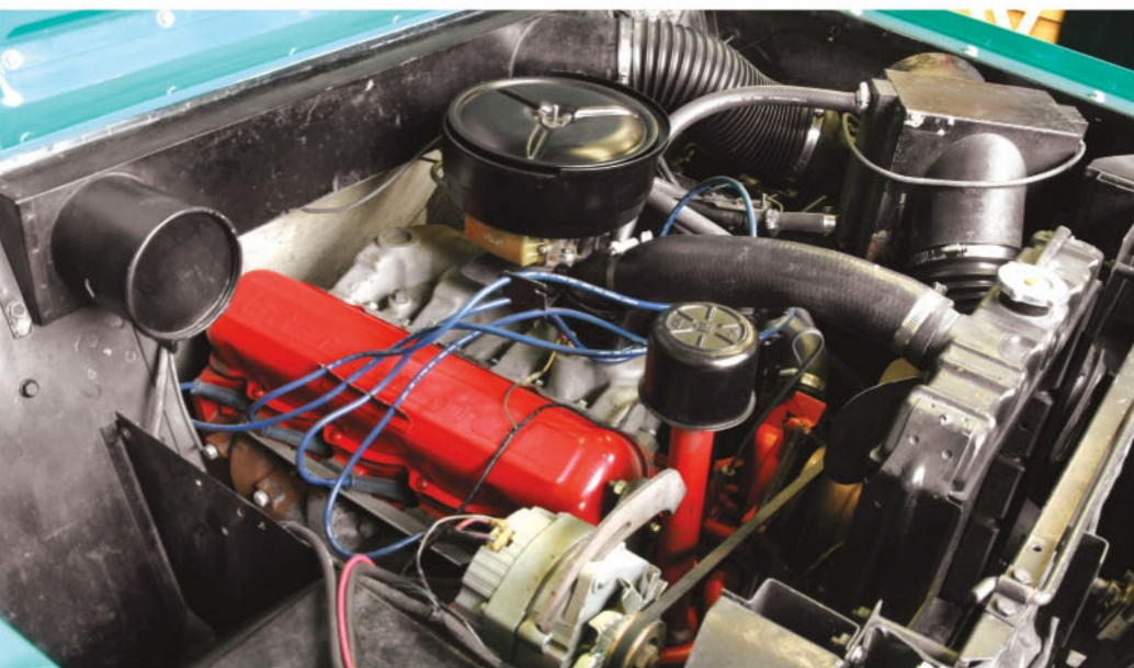
International Harvester's Comanche slant-four displaces 152 cu.in. and makes 93 horsepower. It was derived by subtracting the left-side cylinder bank from the 304 V-8.
