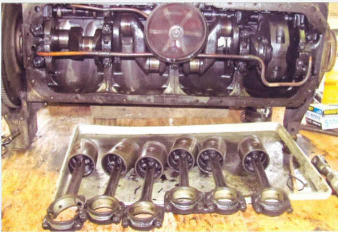
Buick's straight-eight engine, of which there were three different displacements, was introduced for the 1931 model year. The Series-50 line received the 220-cu.in. version rated for 77 horsepower. This engine was found to be sound once it was thoroughly cleaned.
