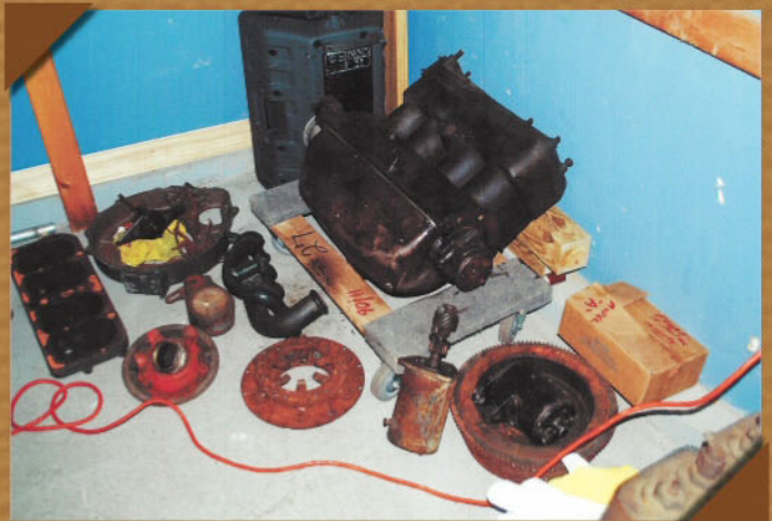
The Overland four-cylinder was deemed too costly and time-consuming to restore, but this 1928 Ford engine was a fine stand-in, being simple to rebuild and upgrade, and making the right sounds. Right-hand drive made installation a challenge, though.
