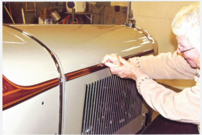
Earlier, the Buick had received a new layer of Capitol Maroon and Lorenzo Gray two-tone paint, at which point the body was reunited with the chassis. A final touch was replicating the factory pinstripe pattern, done by a friend of the owner.
