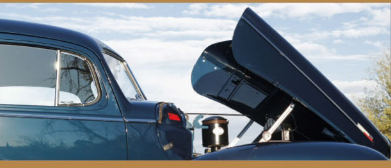
The flathead straight-six engine displaces 175 cubic inches and produces 92 horsepower; all the various instructional stickers have been accurately replicated; large air-cleaner assembly sits atop the single downdraft Carter carburetor; forward-tilting hood provides unrestricted access to the entire engine bay.
