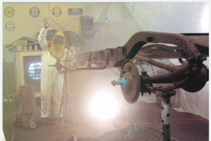
The Buick's steel frame in the process of being media blasted. A decision was made to leave the semi-elliptic springs, front axle, and rear differential in place. Note that the spindles have been carefully wrapped to prevent damage by blasting media.
