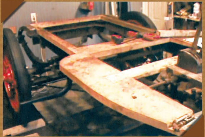
The Overland was stripped down to its original floorboards, which exposed much of the ladder frame, and the gearshift and emergency-brake levers (far right) that would be retained. "I was deciding exactly where to stretch the chassis," Tony says.
