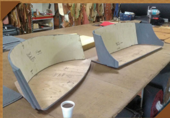
Left to right, the rear- and front-seat bases were fabricated of epoxy-primed wood, with flexible side panels that made them removable as required; they were trial-fit more than 20 times before being padded and upholstered in durable marine-grade red vinyl.
