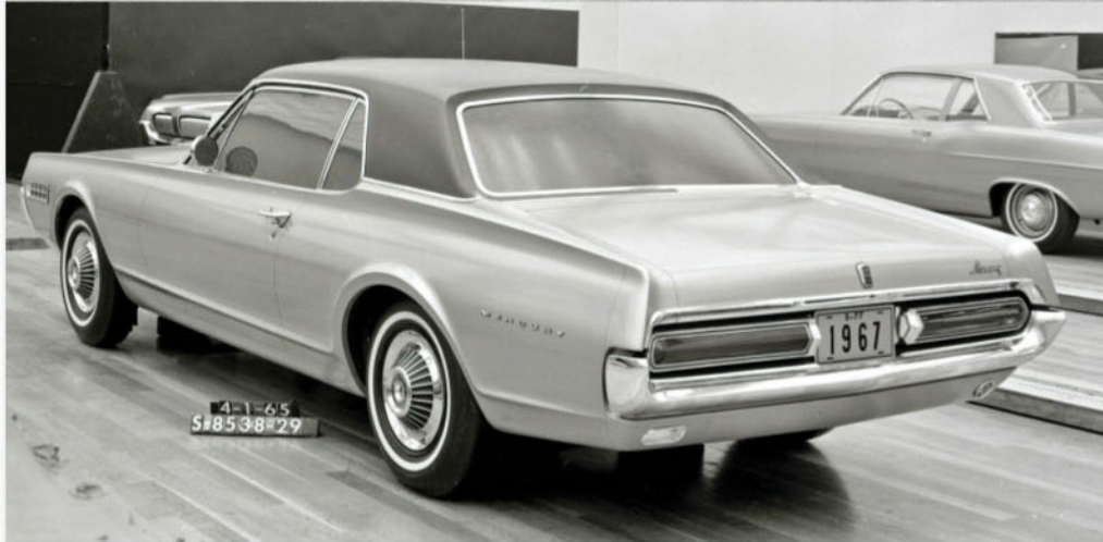
Top: Multiple roofline treatments were considered, even at this late (Feb '65) stage. Above: By April, the lines were largely locked in. Note the taillamps are now a single piece, not yet segmented by the tight chromed ribs that the production car wore.
