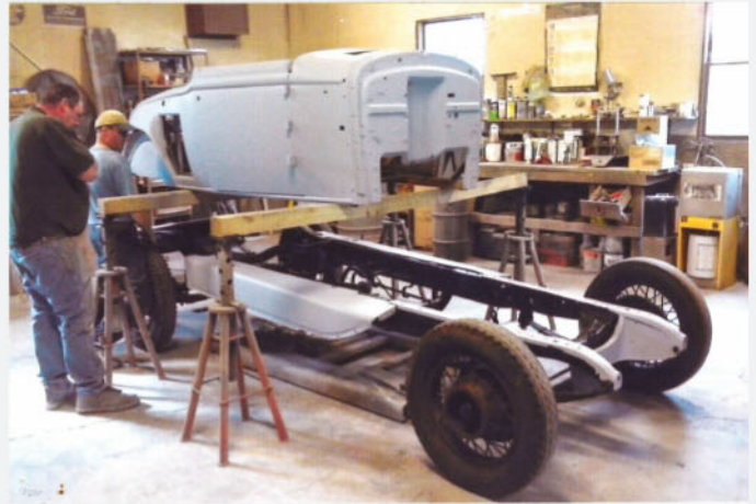
After the metalwork was completed, the two-/four-passenger body was given a final coat of primer and allowed to cure. It was then test-fitted against the restored chassis, reassuring the team that factory geometry had not been compromised during the process.
