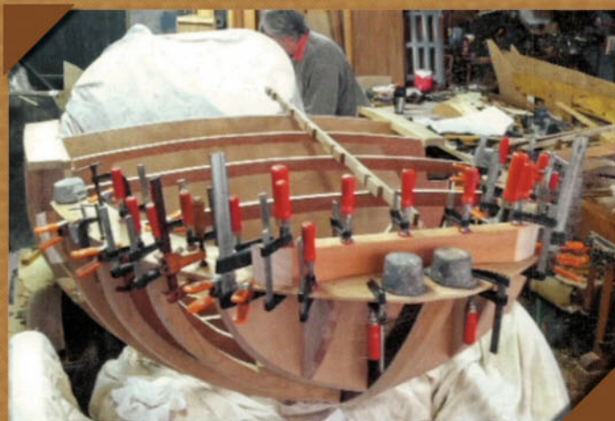
The body was built like a cedar-strip canoe, and each skeleton piece used nine to 12 layers of laminated oak. Tony notes, "We used boat-building adhesives that are designed to withstand temperature swings; once glued, they're very difficult to take apart."
