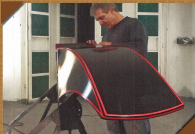
George Papalexandrou of Auto Body Specialties of Patchogue, New York, fabricated four fiberglass fenders, exactly duplicating Tony's plywood models. These were sprayed red, pinstripes masked, over-sprayed in black, stripes revealed, and clear-coated.
