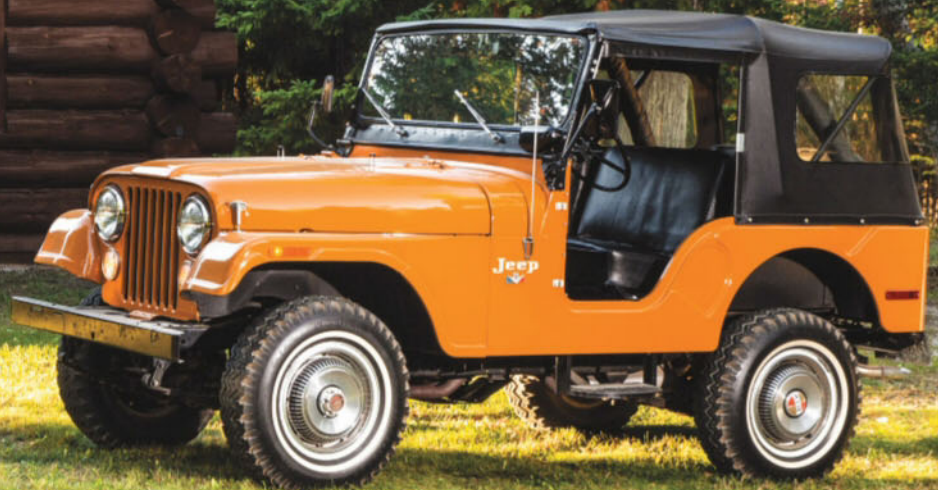
Above a ('55-'71) short-nose CJ-5; below, a long-nose rig ('72-'83). Notice how the long-nose fender has additional sheetmetal and an accent line between the wheel opening and the cowl.
