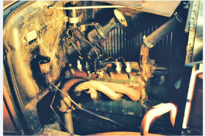
The closed-cab pickup, designated model 82-B by Ford, was meticulously evaluated during its disassembly. Looking worse for wear—though in sound, running condition—was its original 201-cu.in. four-cylinder engine, rated for 40 hp at 2,200 rpm.
