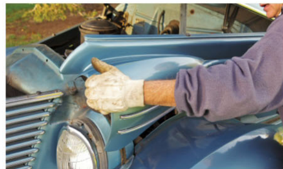
This 245.3-cu.in., 101-hp six-cylinder still uses its original plugs and wires. After unlocking the hood by twisting the ornament, the side panels can be removed.
