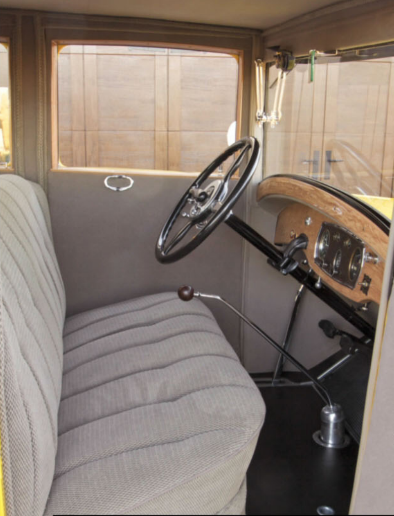
Though this Packard 526 was discovered in pieces, it was nearly complete. Items like these original chrome-edged gauges reside in a crackle-finished bezel; a Tropic-Aire heater was activated via a button on the passenger's side of the instrument panel, and the standard tool kit resides in a hidden interior panel.
