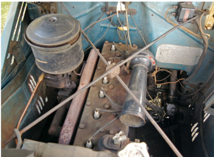
This 245.3-cu.in., 101-hp six-cylinder still uses its original plugs and wires. After unlocking the hood by twisting the ornament, the side panels can be removed.
