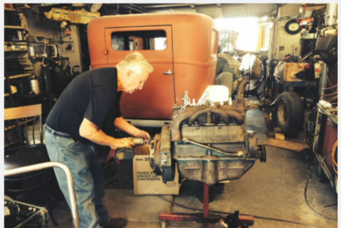
Friend and fellow club member John Cook began the task of examining the 201-cu.in. four-cylinder after it was secured to an engine stand. The three-speed manual transmission has already been removed; the clutch and pressure plate are next.
