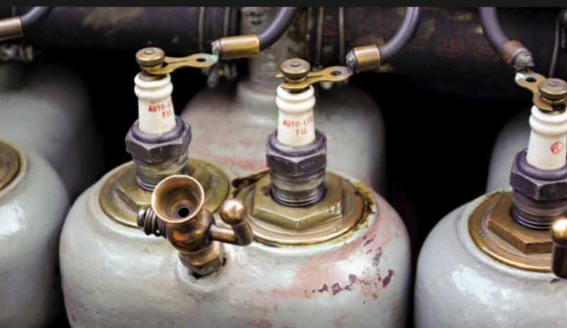
Electrical system was added to the car. Flathead four-cylinder with priming cups is very smooth and powerful, and starts easily. Dual plugs connect to Delco four-coil ignition system.
