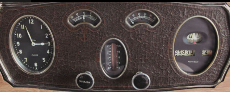
Though this Packard 526 was discovered in pieces, it was nearly complete. Items like these original chrome-edged gauges reside in a crackle-finished bezel; a Tropic-Aire heater was activated via a button on the passenger's side of the instrument panel, and the standard tool kit resides in a hidden interior panel.
