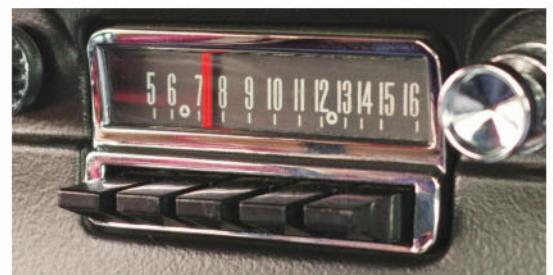
The Rally-Pac was a production Mustang option that solved the issue of where to fit a tach and clock. An AM radio was also installed.
