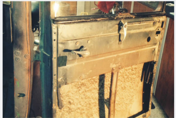
By 1931, the Model A's doors were made entirely of steel. To combat a hollow, tinny noise, a sound-deadening material was sprayed onto the door skin, which is exposed here. The predominantly dry Southwest climate prevented rust from snacking on the metal.
