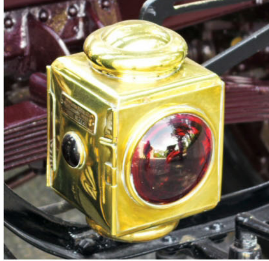
Brass taillamp is kerosene-fired. The deck conceals folding "mother-in-law" seat for third passenger.
