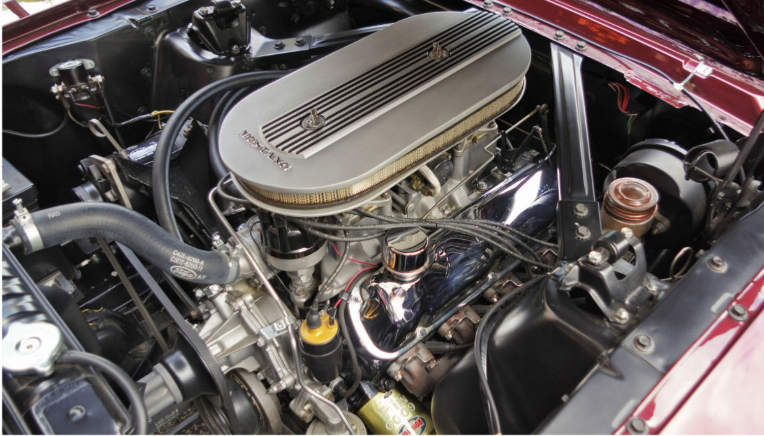
A 302 cubic-inch engine was fitted with 3 x 2 carburetion, chrome rocker covers, and an aluminum air cleaner assembly.
