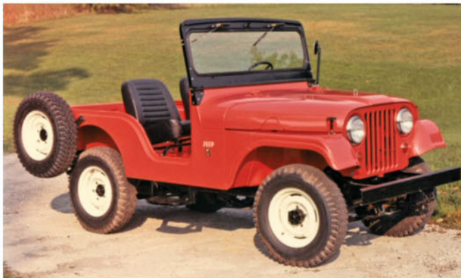
Above a ('55-'71) short-nose CJ-5; below, a long-nose rig ('72-'83). Notice how the long-nose fender has additional sheetmetal and an accent line between the wheel opening and the cowl.
