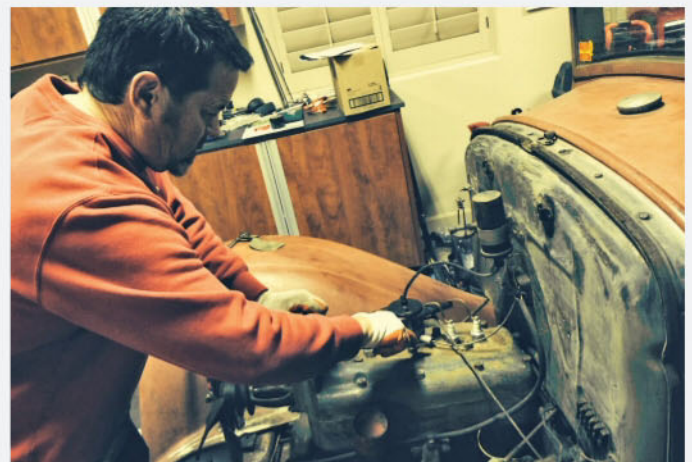
After the small parts were removed from the Ford's exterior, the hood, stainless-steel radiator shell—an accessory in 1931—and radiator were removed, allowing easier access to the engine. Several bolt-on parts were taken off the four-cylinder.
