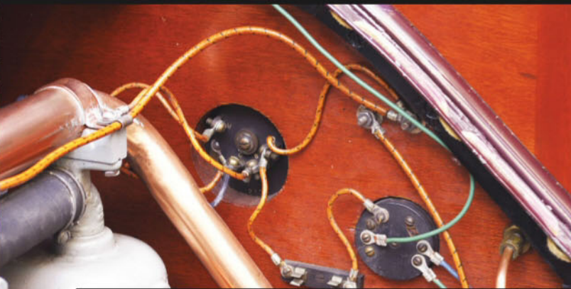
Electrical system was added to the car. Flathead four-cylinder with priming cups is very smooth and powerful, and starts easily. Dual plugs connect to Delco four-coil ignition system.
