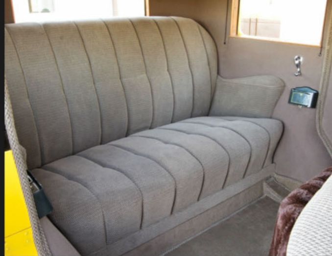
As befitting a Packard, the rear seat offered luxury at arm's reach—an outboard ashtray at each armrest, ribbed cloth seating, and legroom that seems surprising even in a 126-inch-wheelbase car.
