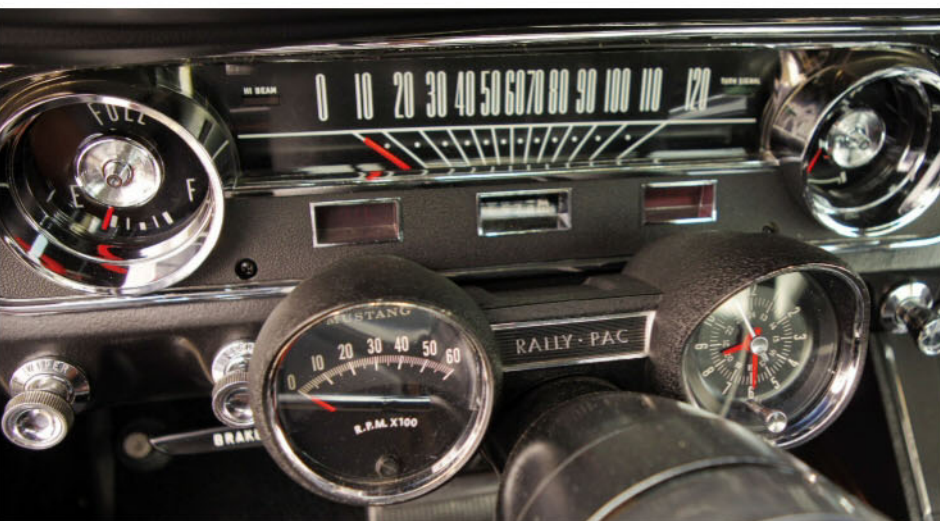
The Rally-Pac was a production Mustang option that solved the issue of where to fit a tach and clock. An AM radio was also installed.
