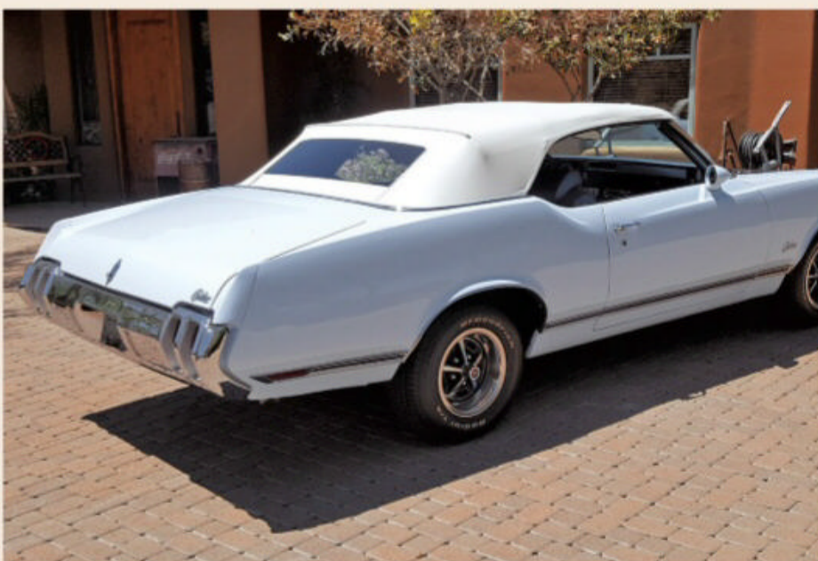
Matching the original factory build, a new white vinyl top was fitted. Hidden from view are new electrically controlled top rams. An original bumper, polished earlier, has been installed, along with new taillamp assemblies. Note the sport mirrors.
