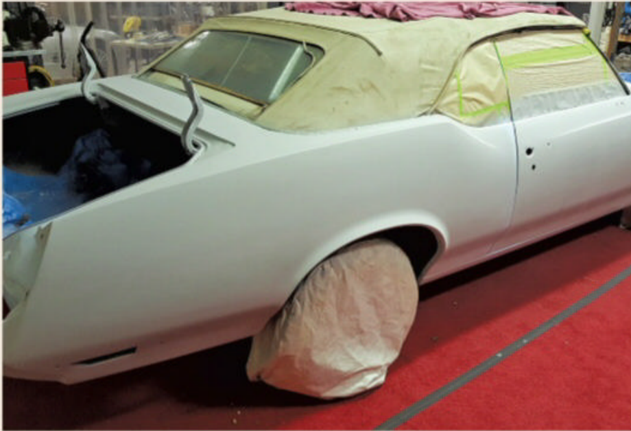
The rest of the Cutlass Supreme was given a final coat of sealer primer, which was then wet sanded smooth using the common step process. When completed, parts of the body that wouldn't need paint were masked, underway here.
