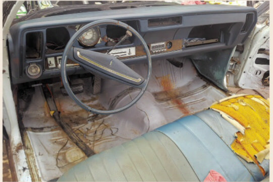
After ensuring the 350-cu.in. V-8 functioned, the instrument panel was disassembled, exposing the original color of the dash vinyl. Note that the dash pad and face were undamaged, even though the steering wheel was cracked in several spots.
