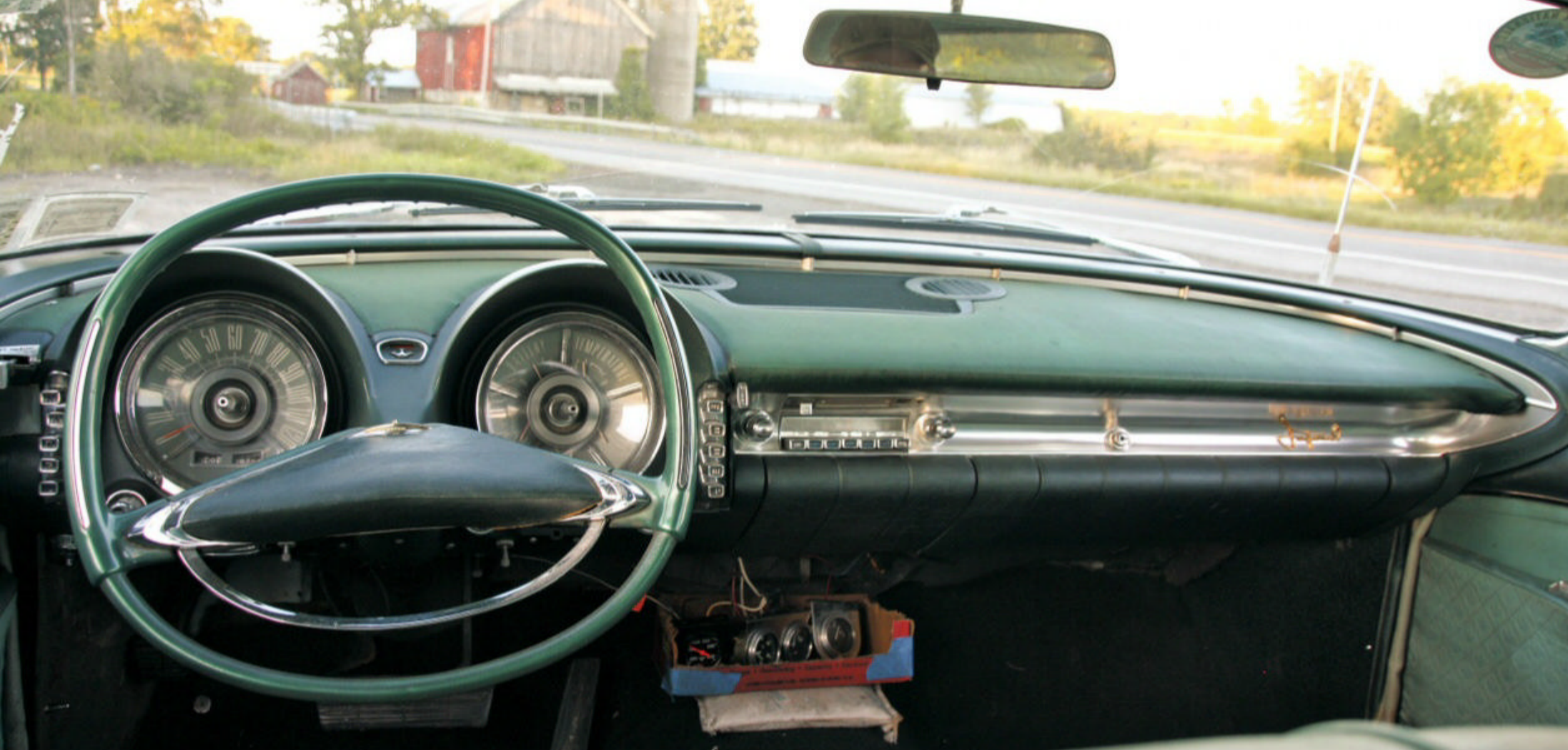
Functional pushbutton transmission controls, electroluminescent gauges, and an elliptical wheel add to the appeal of the budget classic.
