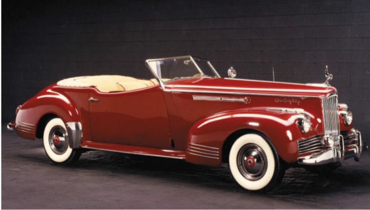
The Twentieth Series Packards for 1942 included this One-Eighty Darrin Convertible Victoria, priced at a lofty $4,595, the only non-Clipper built on that chassis. Just 672 copies of the One-Eighty were built, incorporating all 11 body styles. The engine was a 356-cu.in. L-head straight-eight with 165 hp.
