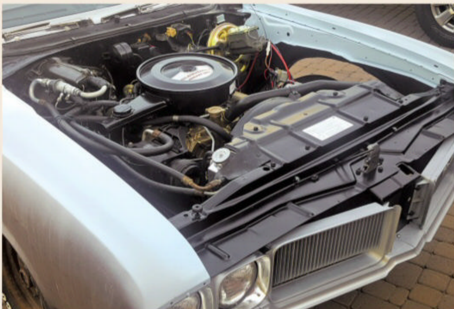
After block sanding the front end of the convertible's body panels, the headlamps assemblies and grilles were installed. This allowed the owner to check tolerances while aligning the convertible's iconic, toothy hood after this photo was taken.
