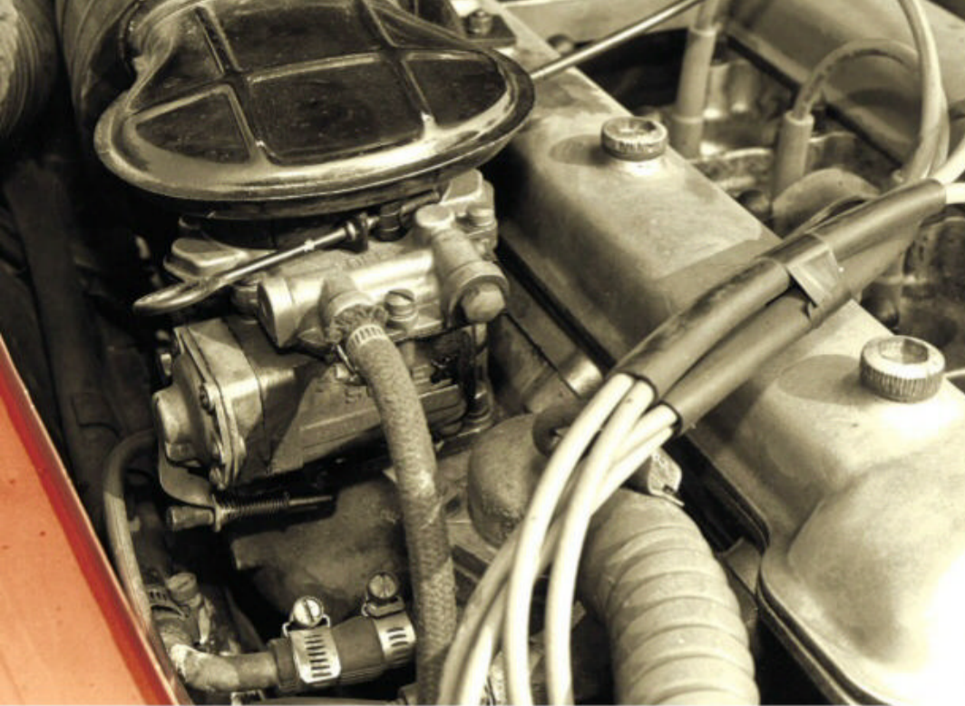
The Spider uses a single downdraft Solex to feed the fuel (left). A large air cleaner on the coupe serves two sidedraft Weber carbs to give it a little extra poke (right).
