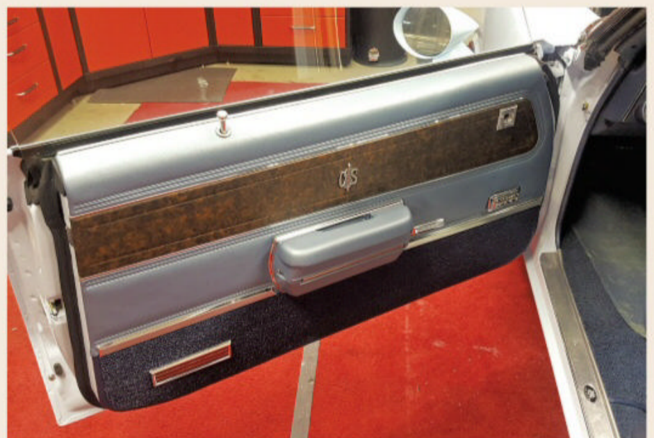
One of the last components to be installed within the convertible were new door panels and weather seals. The upscale nature of the top-of-the-line Cutlass Supreme is on full display here via the combination of carpet, vinyl, and woodgrain trim.
