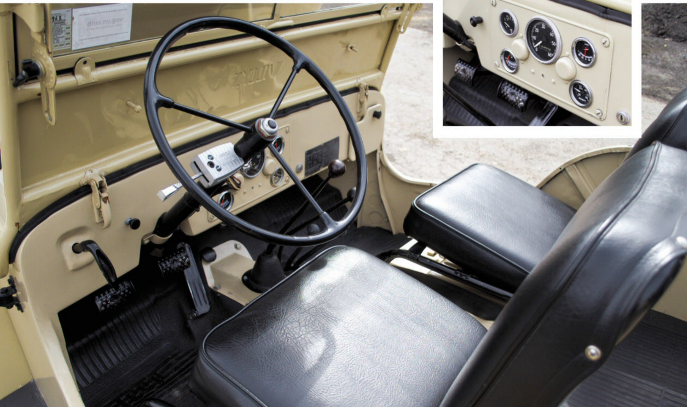
Stark interior offers center-mounted instruments and an array of sticks for the Warner T-90 three-speed, accessory overdrive, and the two-speed Spicer Model 18 transfer case. Early CJ-2s had column-mounted shifters (for the transmission), but floor shift became standard mid-production for the 1946 model year.
