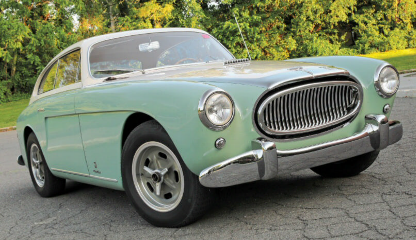
Because they were hand-built in tiny numbers, no Cunningham is identical to its fellows, but this 1952 C-3 coupe is about as typical as the homologation cars get. All C-3s utilized Chrysler engines, and all but the prototype had bodies made in Italy.
