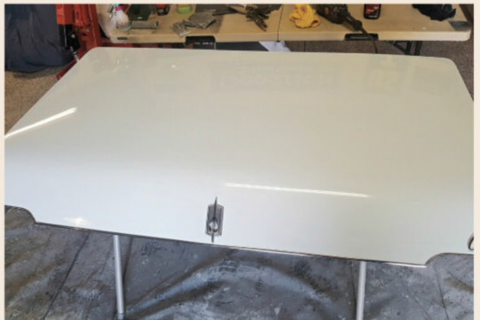
The owner had not painted a car in nearly two decades. To test his ability, he painted the decklid while it was removed from the car; it would be easier to correct if a mistake was made. Happy with the result, he installed its corresponding trim.
