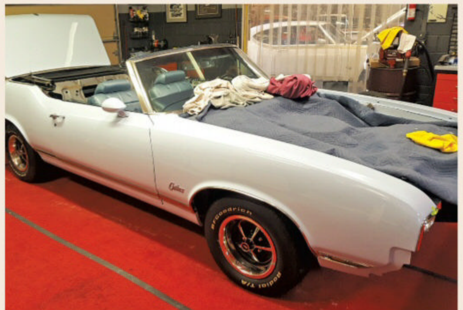
Final reassembly took a leap forward in early 2019 with the installation and alignment of the decklid, as well as side trim and markers, emblems, and door handles. A new windshield has also been installed, along with restored A-pillar brightwork.
