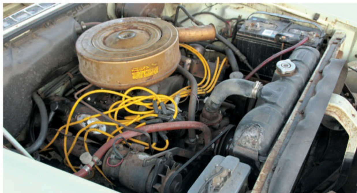
This Imperial Custom has covered around 90,000 miles, thanks to this powerful and durable 413-cu.in. V-8; its four-barrel carb will be replaced to enhance driveability.
