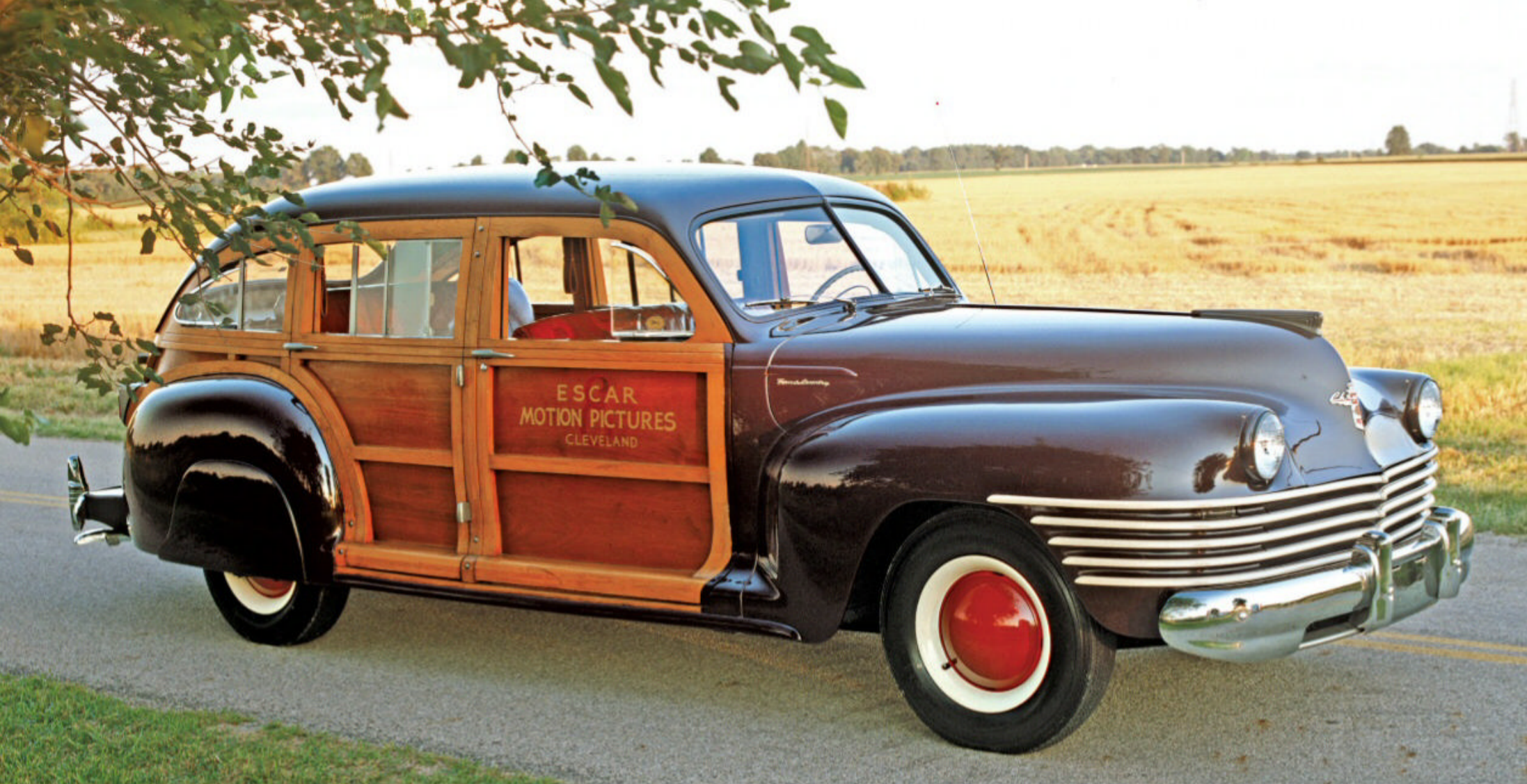
Five horizontal grille bars, painted not chromed, marked the 1942 Chryslers. There were 999 Town & Country wagons built in six- and nine-passenger configurations, in the Windsor series. They used the 250.6-cu.in. L-head straight-six and were priced from $1,595.
