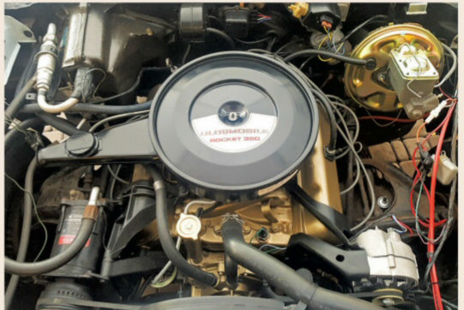
Having tested the optional 250-hp Oldsmobile 350-cu.in. engine, its exterior was restored with correct engine paint, as well as its bolt-on equipment. The air conditioning system was rebuilt, and a new power brake booster and master cylinder installed.
