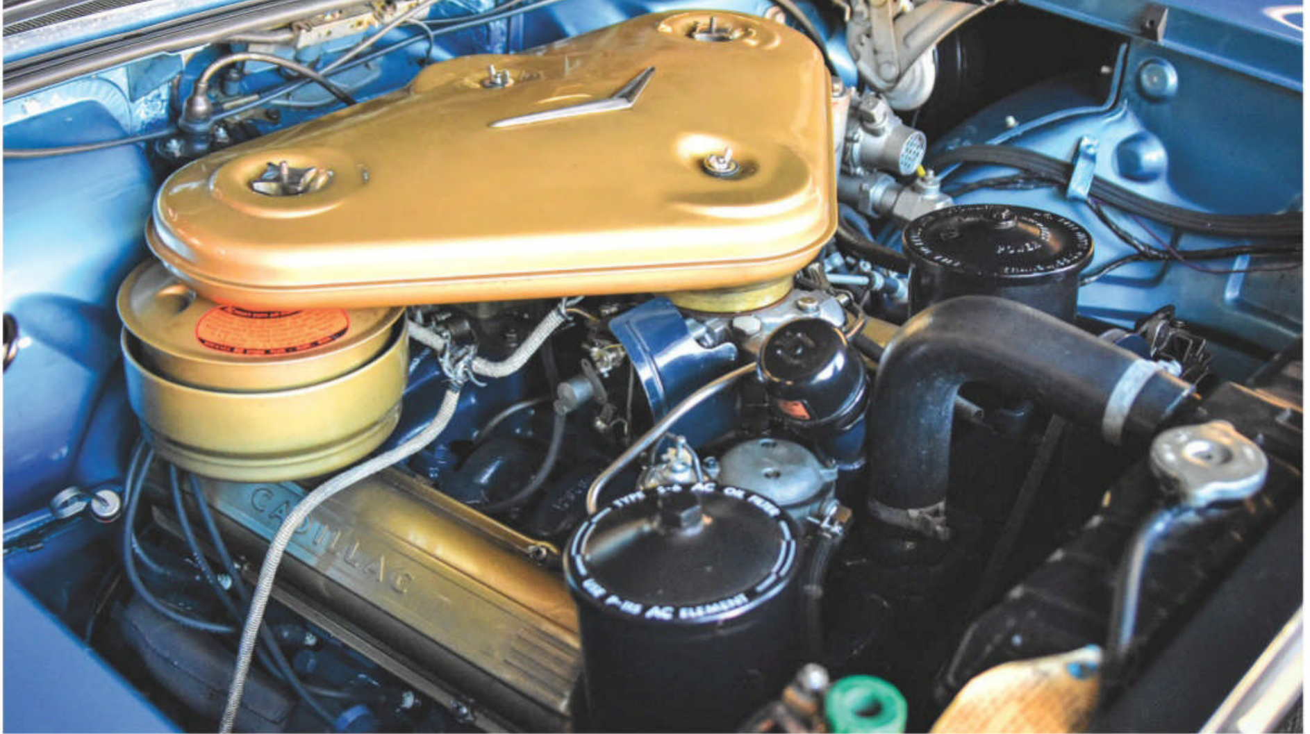
A pair of Carter WCFB four-barrel carburetors lurk under that triangular “bat-wing” air cleaner. They feed a 325-hp, 365-cu.in. edition of Cadillac’s famed first-generation OHV V-8. A single four-barrel, and 300 hp, was standard on the rest of the Cadillac line.
