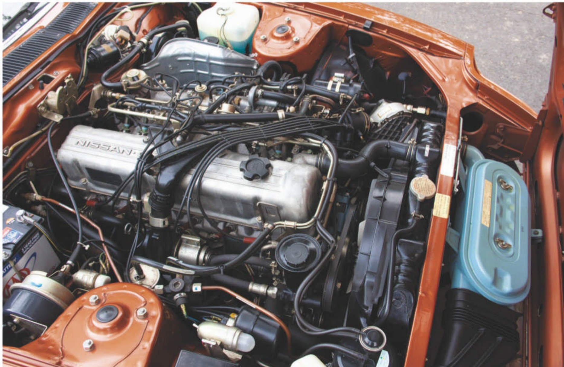
The 280-ZX engine bay was carefully laid out, with reasonable space for routine servicing. This example still wears a perfectly legible factory-applied mylar spark plug instruction sticker on the cam cover, seen above middle left, an item typically lost due to wear.
