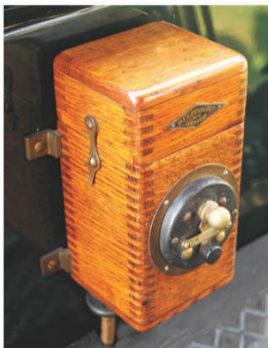
The dash-mounted Spark Coil, also called “Buzz Box,” is the Cadillac’s magnetic circuit breaker, a key part of which is a .25-inch diameter “cut-out plug” that needs to be inserted to start the car. A knob controls the contact arm, allowing the operator to easily switch between two batteries.
