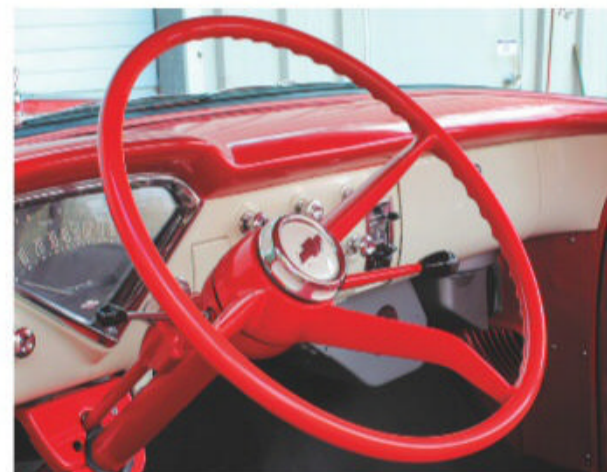
The instrument cluster includes gauges for temperature, amps, oil pressure, and fuel level, along with a 100-mph speedometer. This truck's odometer was reset to zero at time of restoration, and now shows just 1,541 miles.
