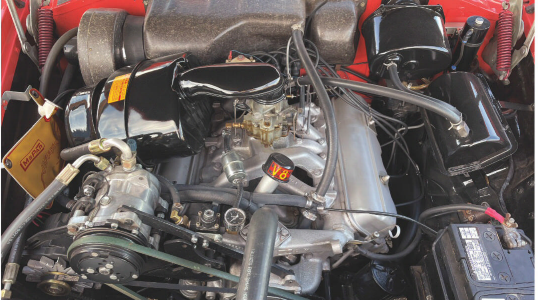
Since the FireSweep was Dodge-based, it received the Coronet's 325-cu.in., two-barrel, 245-hp polyspherical-headed V-8 as standard.
