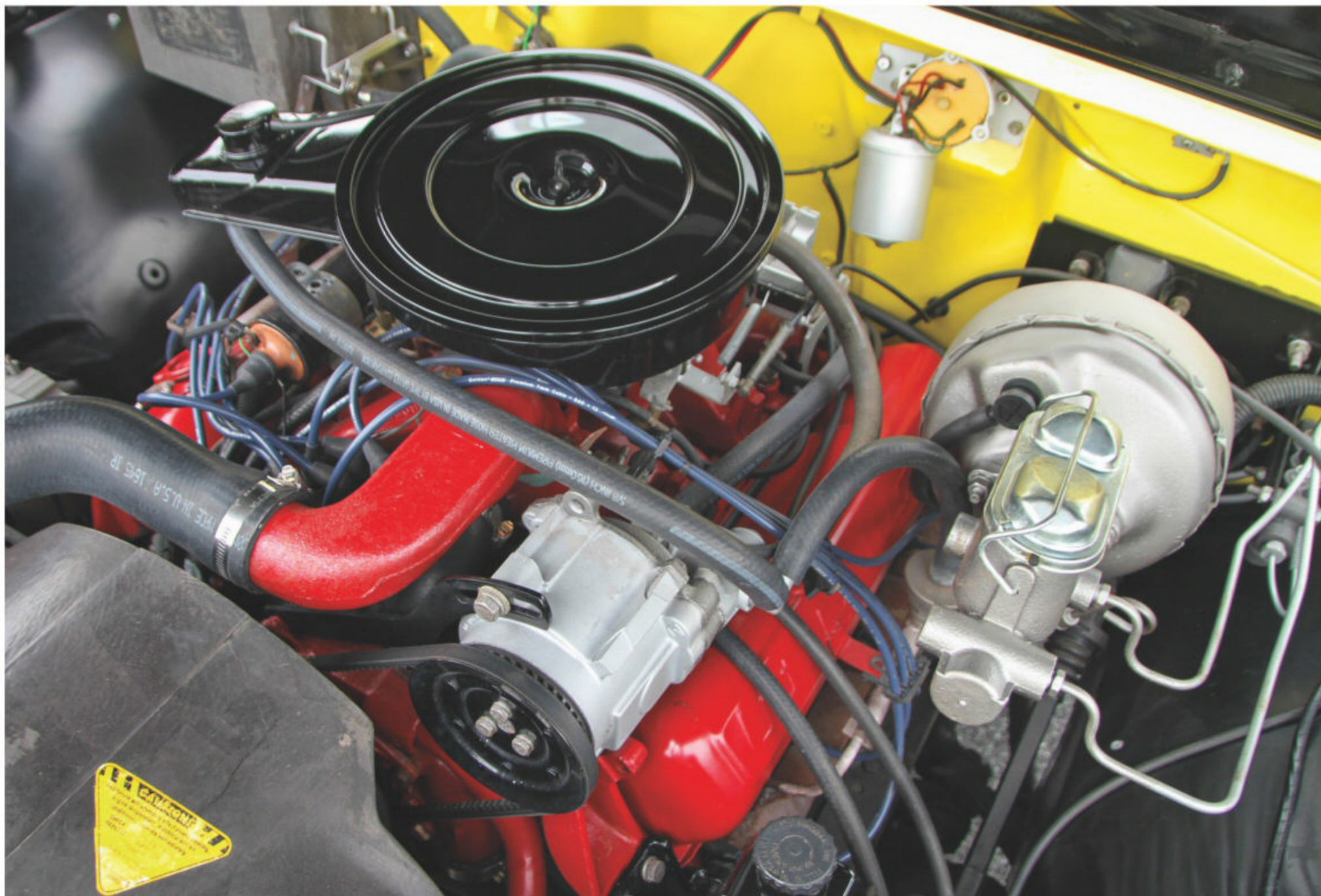
A 345-cu.in. International V-8 is rated at about 150 hp but has ample grunt to power this '74 half ton. The engine has been overhauled once, as has the TorqueFlite automatic it's paired with.
