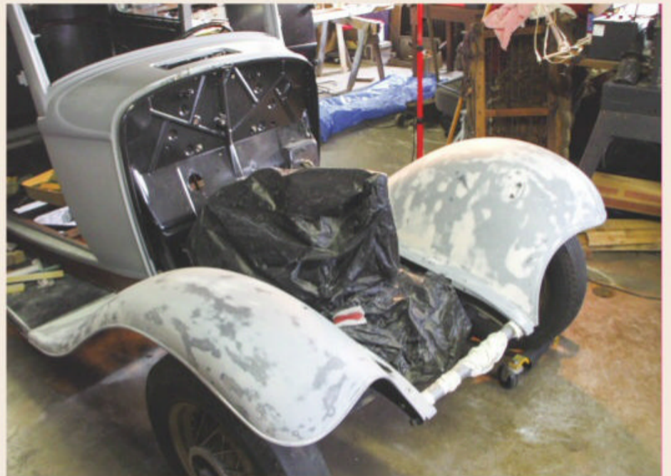
The body was reunited with the chassis and preassembled a few times to check and correct panel and fender fit. Afterward, the shell was block sanded/wet sanded from 220 grit up to 600 grit (not shown).
