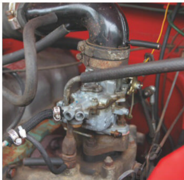
The 70-hp, 2.25-liter four-cylinder OHV gasoline engine was derived from the diesel. Introduced for the Series II, it would remain the standard Land Rover engine into the 1980s.
