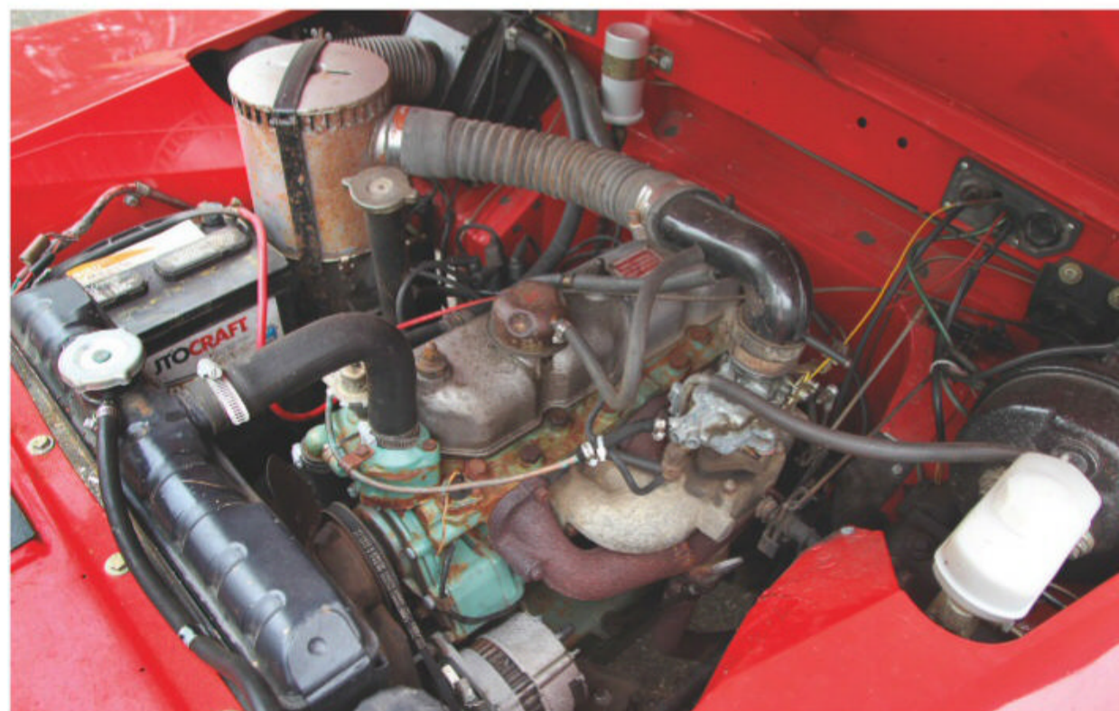
The 70-hp, 2.25-liter four-cylinder OHV gasoline engine was derived from the diesel. Introduced for the Series II, it would remain the standard Land Rover engine into the 1980s.
