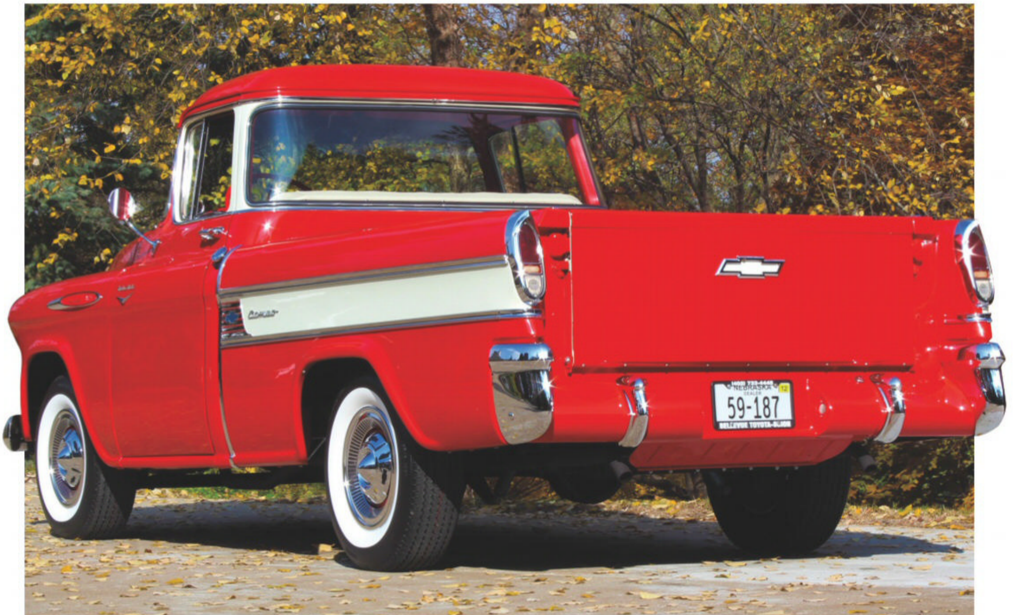
Molded Fiber Glass of Ohio was contracted to build the slab-sided panels and tailgates for the Cameo, which was the most obvious design change.
