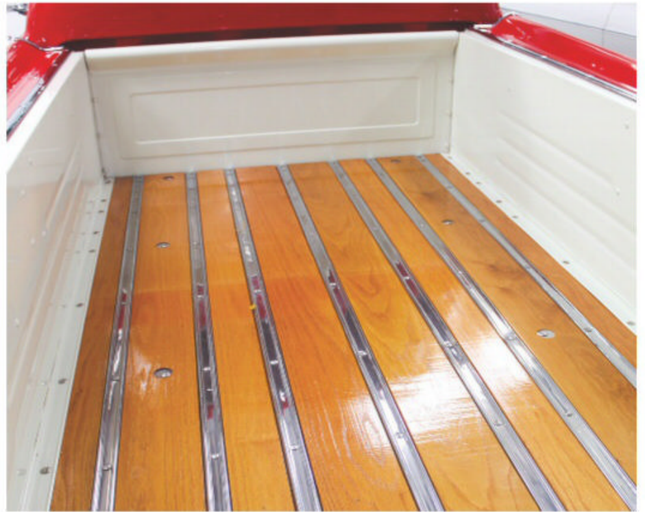
The stock stepside bed was used, but with built-out fiberglass panels attached, as shown. The previous owner dressed up the bed with oak slats and chrome-plated rails.
