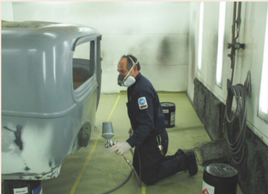
Bud transported the shell to WyoTech where Gary used the school's spray booth after hours to apply multiple coats of PPG high-build primer. Bud then brought it back to his shop.
