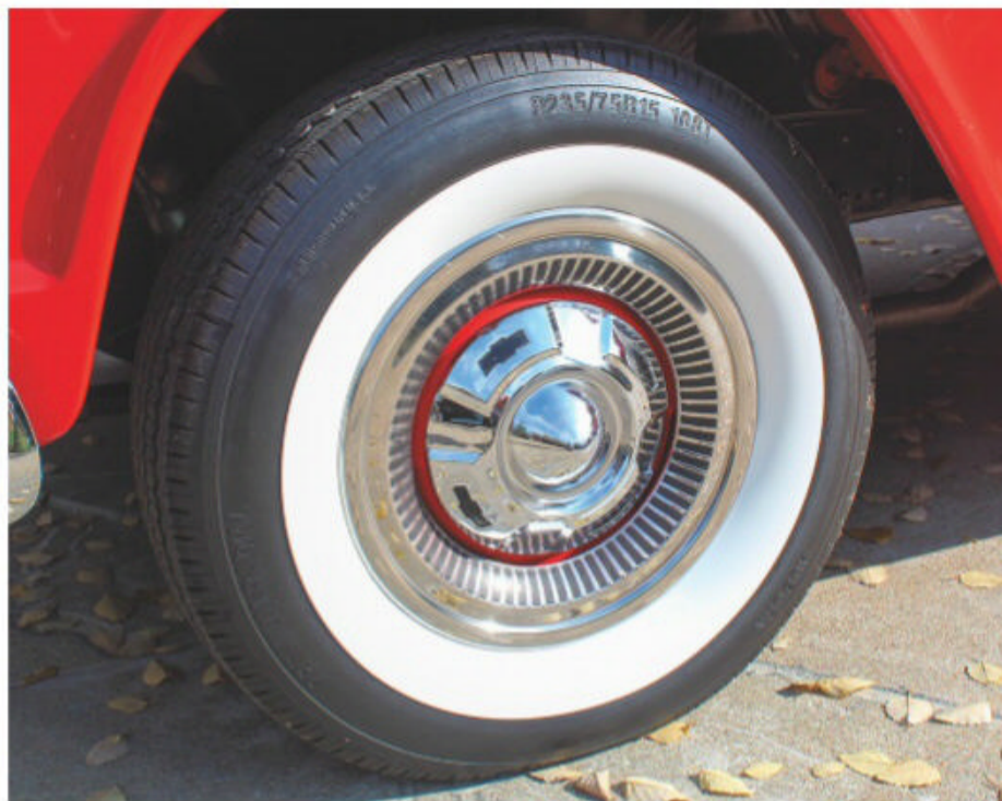
The wheels and tires consist of a set of Diamond Back 3-inch whitewall P235/75R15 radials, mounted to stock steel wheels with correct hubcaps and beauty rings.
