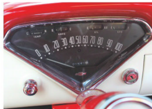
The instrument cluster includes gauges for temperature, amps, oil pressure, and fuel level, along with a 100-mph speedometer. This truck's odometer was reset to zero at time of restoration, and now shows just 1,541 miles.
