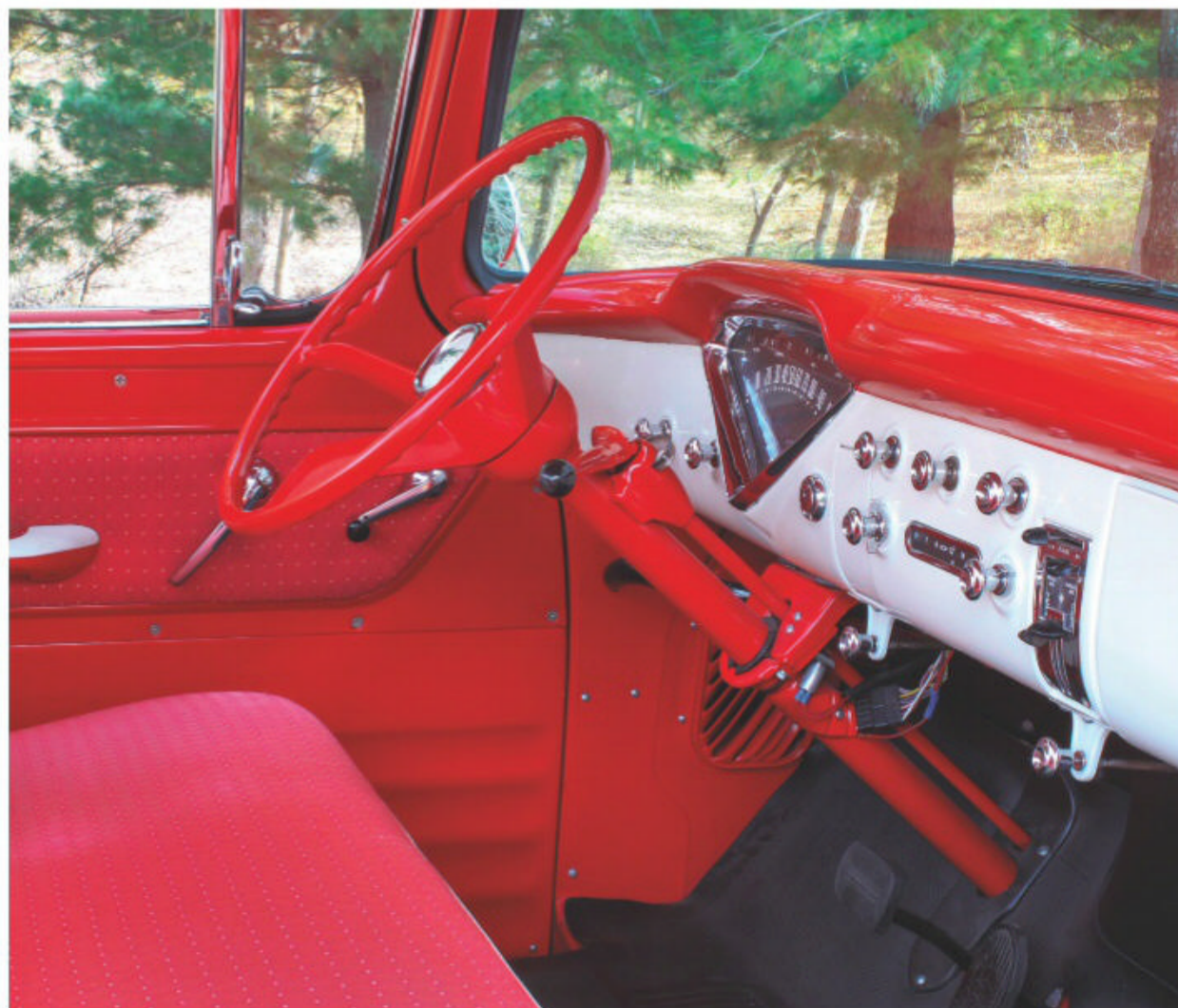
The stock interior, though plain by today's standards, includes a cloth and vinyl upholstered bench seat, padded door inserts with armrests, rubber floor mats, two-tone dash, AM radio, and a heater/defroster.
