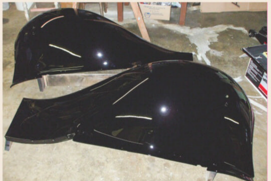
Once the paintwork was completed, these front fenders, like the rest of the body, were wet sanded with 1,000-, 1,500-, and 2,000-grit paper. Next, the finish was buffed and polished using 3M products to reveal the shine.
