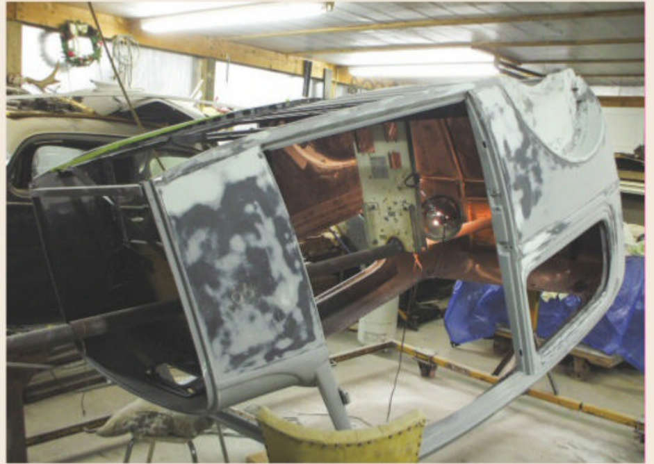
The body filler was sanded with 80-grit paper, then a glazing putty with a hardener was applied to fill minor imperfections and the areas were sanded with 180-grit paper.
