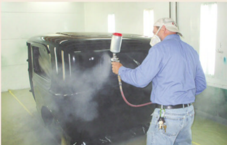
Back at WyoTech, after cleaning the surfaces, masking the window and roof openings, and wiping down the body again, Gary applied a single coat of black sealer followed by three coats of PPG paint in black and then three coats of clear. He repeated the process on all the body parts.
