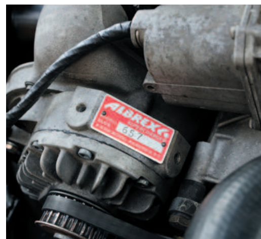
◁ M117 V8 was modified to produce 400bhp.
