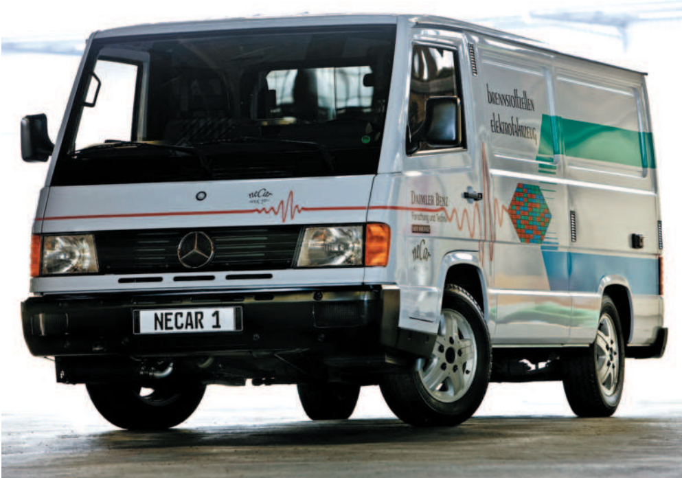
△ The NECar 1 from 1993 was the first working prototype to feature fuel cell technology, with the system filling the entire load area of the van.
