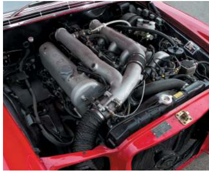
△ Ancillaries made the M100 a large engine to package.
