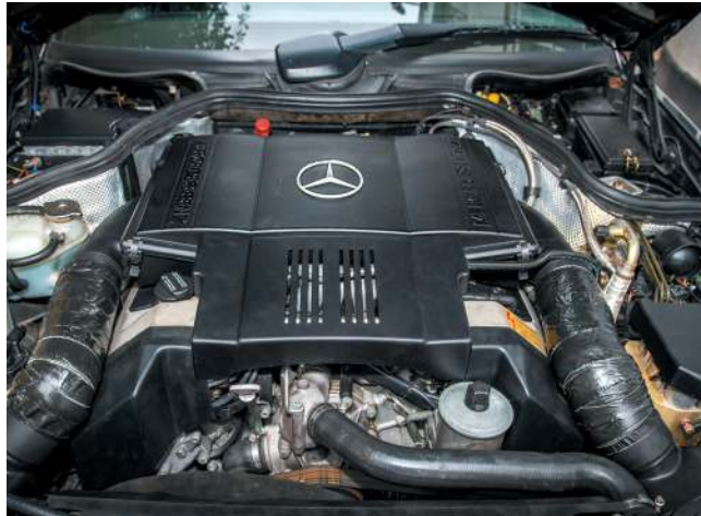
M119 V8 is a reliable unit, but as with all 124-series engines, does suffer from wiring loom issues.
