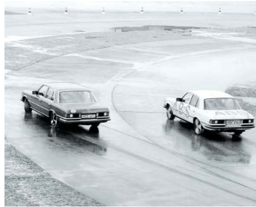
▽ Braking too late can trigger understeer as the tyres are overloaded.
