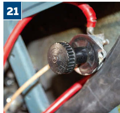
21 Dan also took the opportunity to remove this crude battery cut-off switch from the car's rear inside quarter; he'll replace it with one that allows power to the onboard security system but kills a feed to anything else that might drain the battery
