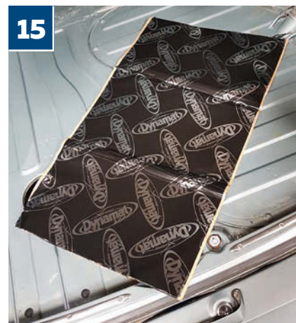
15 A bulk box of Dynamat Xtreme contains nine sheets measuring four square feet each; the luggage area of Dan's car took 44sq.ft. of material
