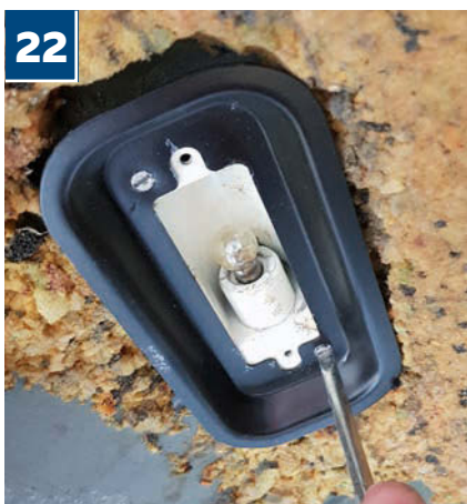
22 Don't forget to remove all brackets, fixtures and fittings, including the interior light fitting on the inside of the boot lid, before applying Dynamat Xtreme.
