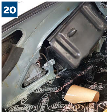
20 A heavy coating of Waxoyl (presumably carried out during the car's earlier restoration at the hands of a previous owner) appears to have preceded Dan's work in the luggage area
