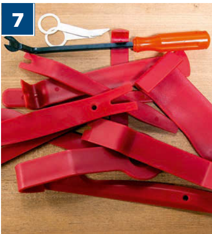
7 More excellent gear for the job at hand: this Phyles fourteen-piece interior trim removal kit was to prove useful when Dan was working his way through the car
