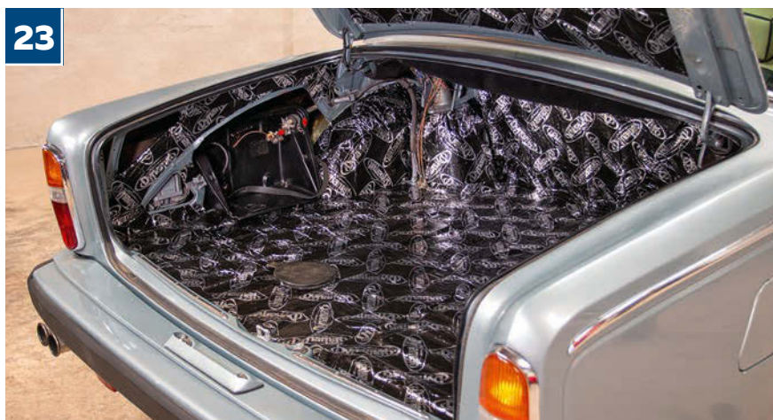
23 It might have taken two days in total, but with the inner wheel arches, rear bulkhead, floor and inside the boot lid and fuel filler cavity covered, this might well be the world's quietest Silver Shadow II luggage area
