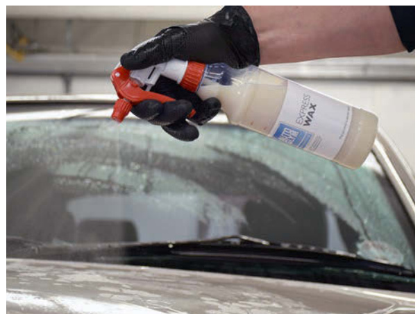
Once rinsed, instead of drying the Arnage straight away, Ryan applied Autoglym's Express Wax. This is a product that can go on to a soaking wet car and is effectively applied as you towel it dry. It's an easy way of building up a protective layer.
