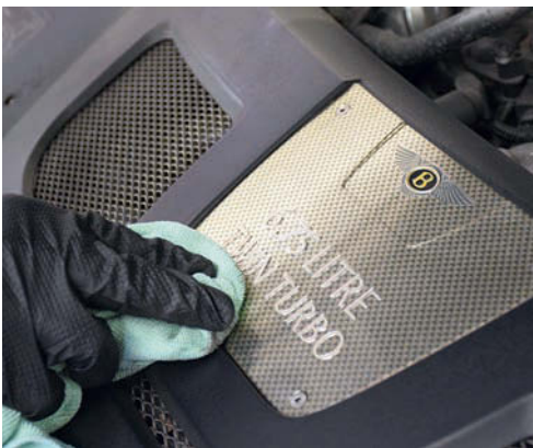
We'll cover the subject of engine bay detailing in a future issue, as this is an area that deserves its own dedicated section. In the case of the Arnage, however, the engine – being mainly covered and recently cleaned – was simply wiped down with a damp cloth before being dressed on the cover with Autoglym's plastic and rubber product.
