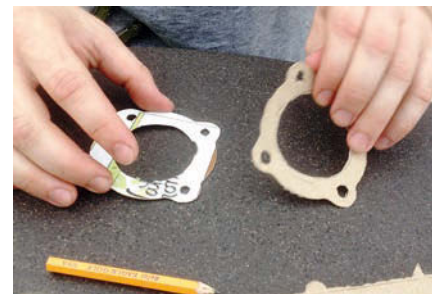
A new thermostat gasket was fashioned from a granola bar box!
