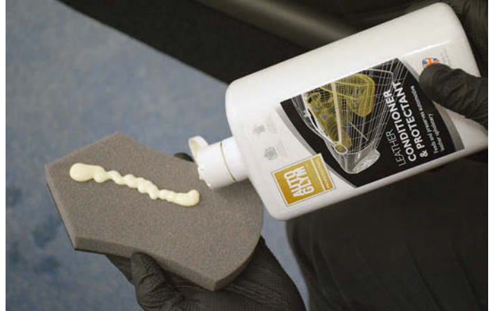
Once the upholstery (which obviously included the door trims as well as the seats) was thoroughly cleaned, Autoglym's logically labelled Leather Conditioner was applied to all surfaces to protect the hide and to nourish the surface. A product like this should also enhance the leather smell of the whole interior.
