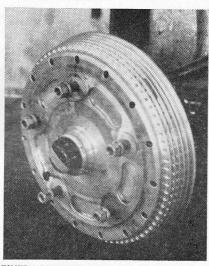
FINELY MACHINED is this Spyder brake drum, with each fin drilled for cooling and weight-saving. The dark patch between the fins is a balance weight.
