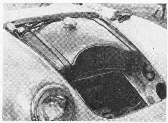
FUEL TANK (above) of the Spyder is mounted in front of the driver and has a "cutaway" to accommodate the spare wheel.
