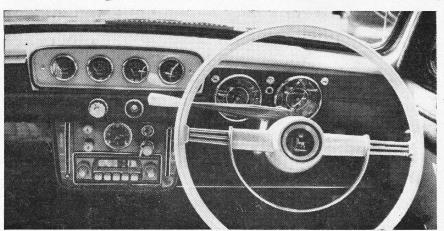
RARE TREAT nowadays, to find such a comprehensive and practical instrument lay-out. Gauges for water, fuel, oil and amps. are in the centre, with rev.-counter and speedometer in front of the driver. The steering column gear lever, however, seems a strange choice for such a car.
