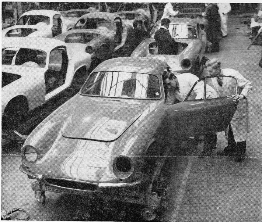
LOTUS ELITE bodies coming off the production line at the Plastics Department of Bristol Aircraft.
