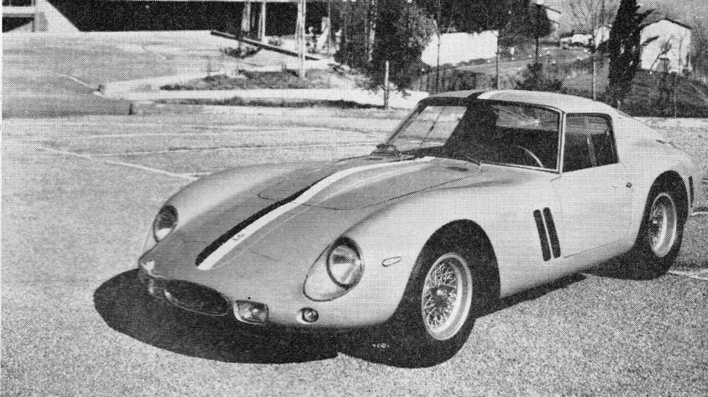
GRAND TOURER: The 1962 250 GTO Berlinetta Ferrari, with a dry weight of 880 kg. The 2,953 c.c. (73 mm. x 58.8 mm.) V-12 engine gives 300 b.h.p. at 7,400 r.p.m.
