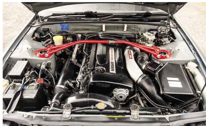
Above and previous page: R32 (the grey car) revived the 'Skyline GT-R' name in 1989 after 16 years of dormancy; its R33 successor (black) was heavier but no less impressive. Below: twin-turbo straight-six was designed to handle huge power increases
