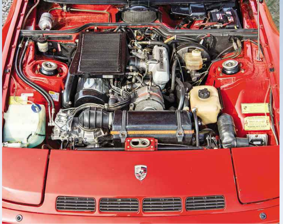
Above: add-on arches allowed the race cars to run wider rubber. Right: addition of intercooler helped wring up to 320bhp from 2 litres, though standard CGT had 207bhp
