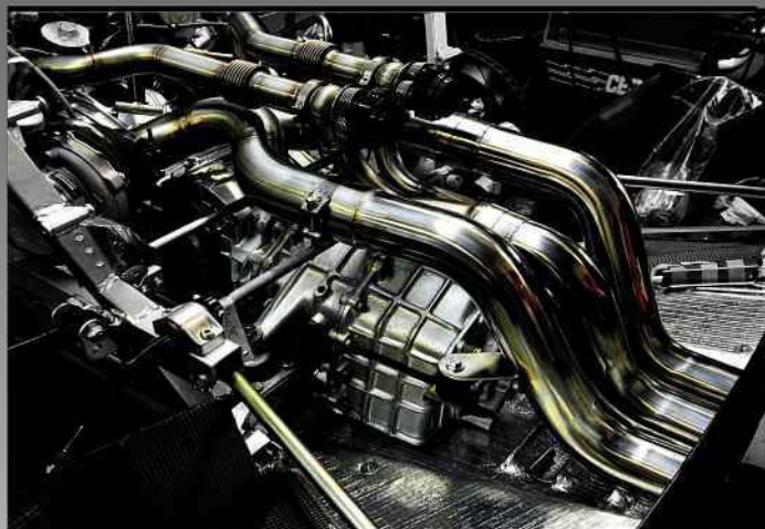
Ferrari F40 uprated to 720 Bhp; In-house work included full engine transmission and suspension re-build, carbon fibre work, interior trim, paintwork and exhaust system plus fitment of the latest hybrid turbos and Motec ECU's.
