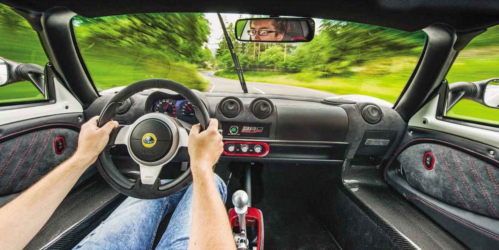
Above: front diveplanes and louvres plus a bigger rear wing contribute to 200kg of downforce at the 175mph top speed, though Lotus says the effects can be felt at just 60mph. Below: cosy cabin uses reams of Alcantara; note the skeletonised gearshift mechanism and the carbonfibre sills
