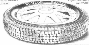
TYRE TYPE: 5 STUD FITTERA, 30x7.9 ORIGINAL EQUIPMENT 1924 BUGATTI 13
