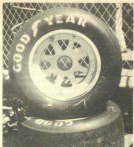
"The Alfa Romeo team and Italian Campagnolo cast magnesium alloy wheels. They are an old established Italian wheel firm from near Bologna."
