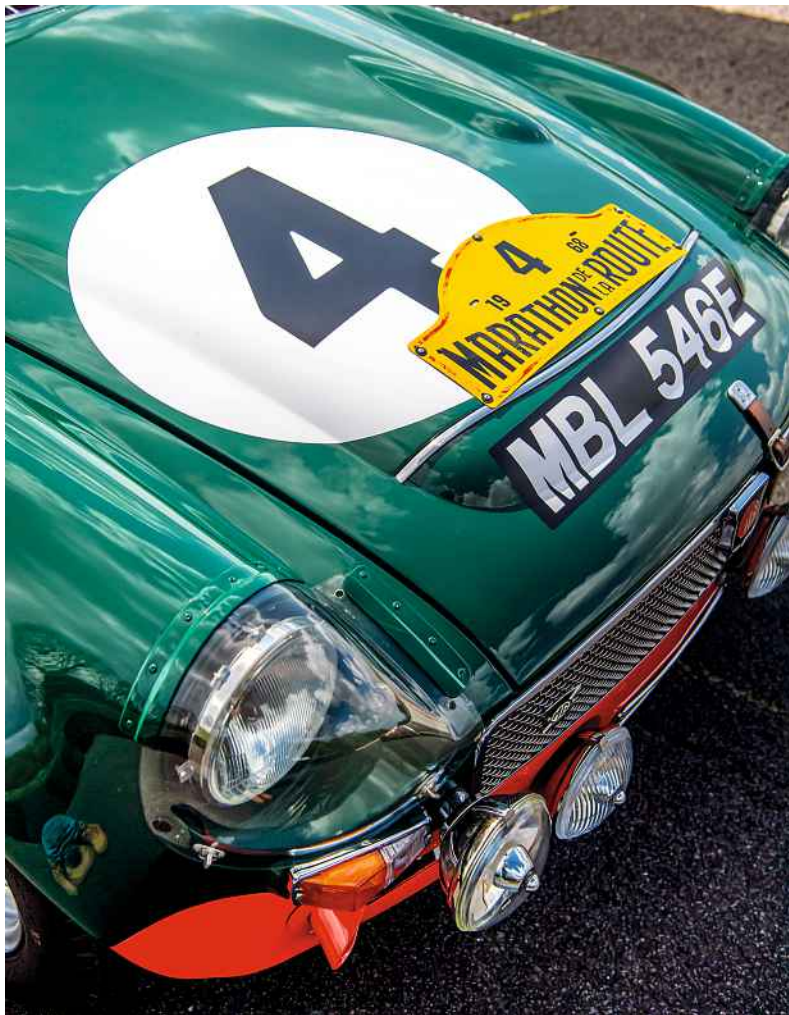
Clockwise, from above Bonnet hump clears straight-six beneath; GTS handles somewhat better than standard MGC; its first outing, the 1967 Targa Florio, driven by Paddy Hopkirk with Timo Mäkinen, with a tuned B-series and MGB bonnet...
