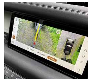
From top Need a good tow vehicle? Look no further; clever camera tech makes trailer hook-up easy.
