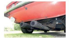
Each of these twin silencers is a Cherry Bomb and a half. The result takes much of the treble snarling out of the exhaust note, leaving a pleasant cruising grumble with a full-throated roar when pushing on.
