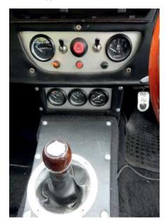
Instrumentation is now rather more comprehensive, and includes an oil temperature gauge as well as coolant temp.
