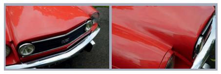
Additional bodywork on the bonnet was executed in welded sheet steel and filler. The extra lights and grille are interesting and practical.
