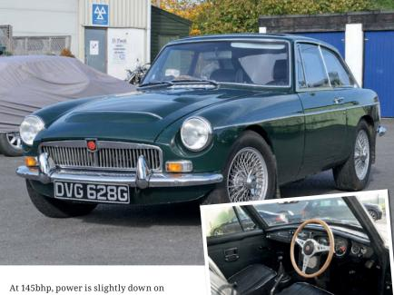
the TR6 (150bhp), but the difference in performance is negligible, and in any case the C has more torque. We're talking about a 0-60mph time of 8.2 seconds for the TR and 10 for the MG, though the gap is even smaller with the post-'73 125bhp TR.
