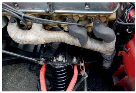
Wrapping the manifolds reduces engine bay heat, but does so by transferring the heat further down the exhaust system. You have to decide where it goes.
