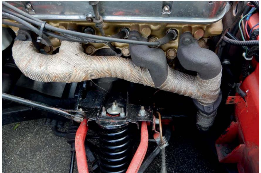
Wrapping the manifolds reduces engine bay heat, but does so by transferring the heat further down the exhaust system. You have to decide where it goes.
