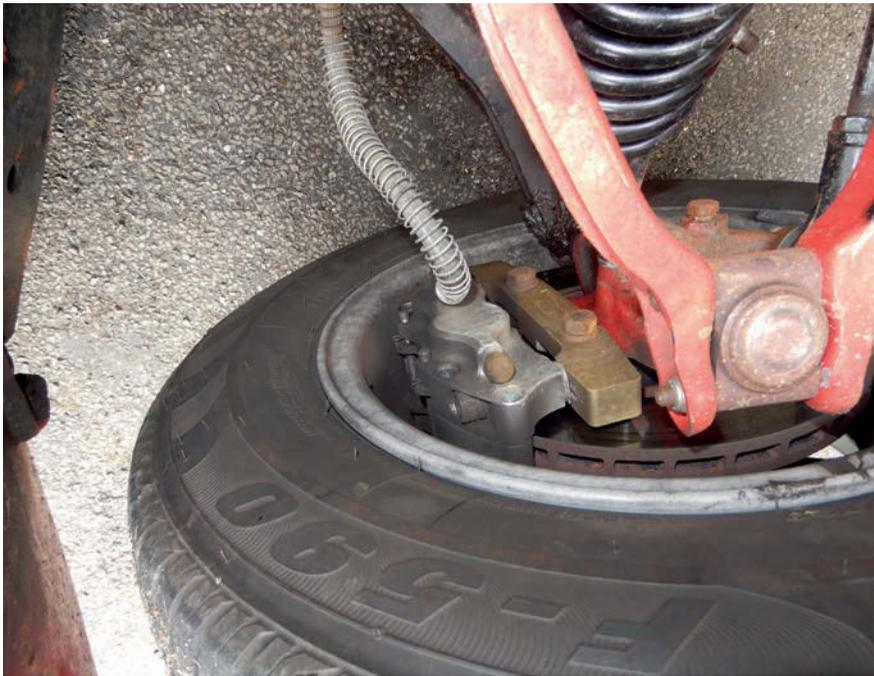
GT6 suspension and spring rates stiffen up the front a little, as the all-iron Triumph straight six is a lot heavier than the all-alloy Rover V8.
