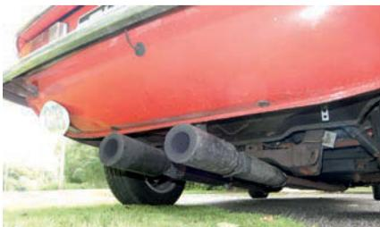
Each of these twin silencers is a Cherry Bomb and a half. The result takes much of the treble snarling out of the exhaust note, leaving a pleasant cruising grumble with a full-throated roar when pushing on.
