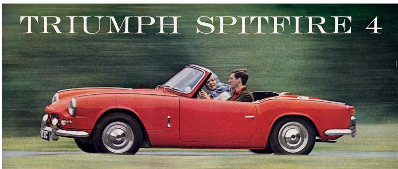
**W**hen the original Triumph Spitfire first appeared on the scene way back in 1962, the concept couldn't have been any simpler. Take one Herald-derived backbone chassis, fit twin SU carburettors to the existing 1147cc engine, clad the whole lot with a sexy, sporty body and you had the perfect recipe for an MG Midget and Austin-Healey Sprite competitor.
