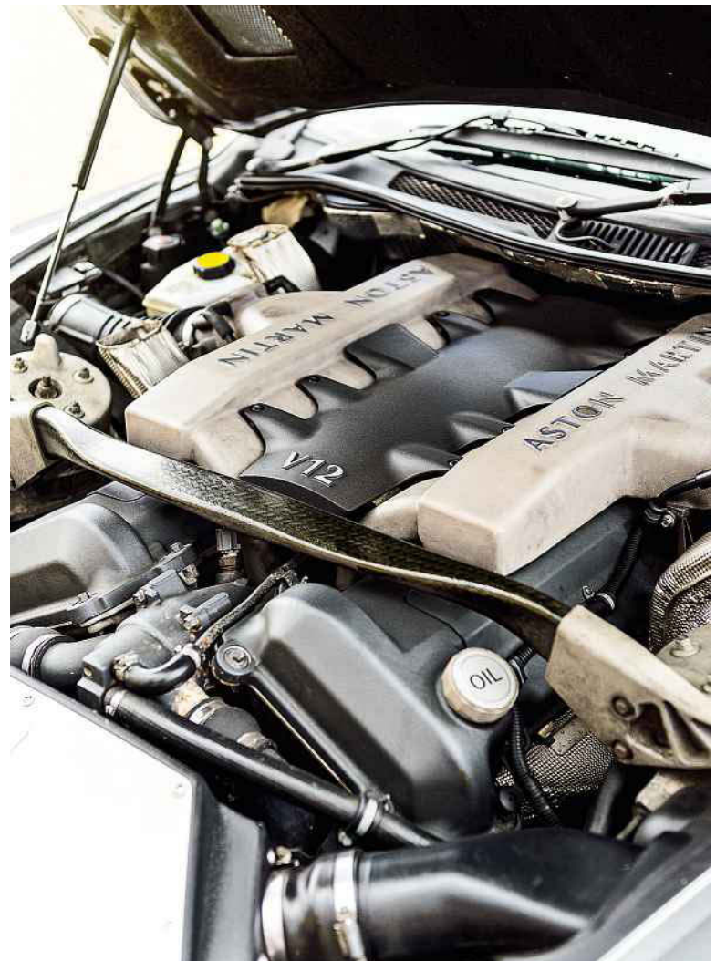
Left and below Auto conversion is integrated seamlessly, so you still use the original selector buttons on the centre stack and the paddle-shifters for manual gearchanges, just as you would with the original automated manual. Six-speed auto complements the original 5.9-litre 460bhp V12 beautifully, too.
