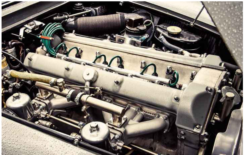
Above and left Street corner near the Mews is as busy and bustling today as it was in 1968, and everyone loves the Aston. Below: twin SUs, as original, but the engine has benefited from an RS Williams conversion from 3.7 to 4.2 litres. There was a three-carb Vantage engine option in period, but the majority of Convertibles had standard engines
