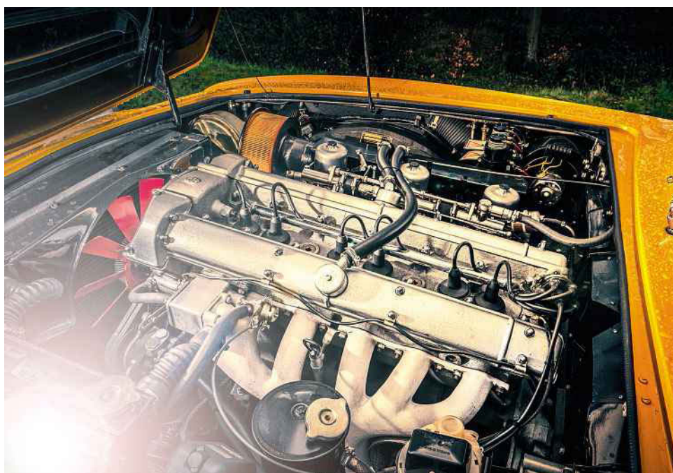
Left and below Moore actually got a credit for Sir Brett's tailoring. Well, it was the '70s. Below: popping the bonnet reveals the DBS's 4-litre straight-six with its trio of SU carbs
