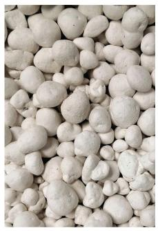
Each tonne of Blue Planet calcium carbonate aggregate can capture and sequester up to 440 kg., or 920 lbs., of carbon dioxide gas.
