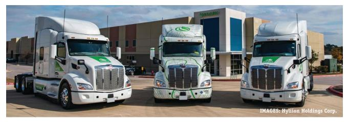
Holcim US has spec'ed Hyliion Hypertruck ERX electric powertrains for 10 tractors serving Texas and Oklahoma cement and concrete operations, plus sister roofing product businesses. Batteries powering the Hypertruck ERX draw from an onboard generator running on compressed natural gas (CNG) or renewable natural gas (RNG), consumption of which compares favorably against diesel fuel when measuring carbon dioxide emissions.
