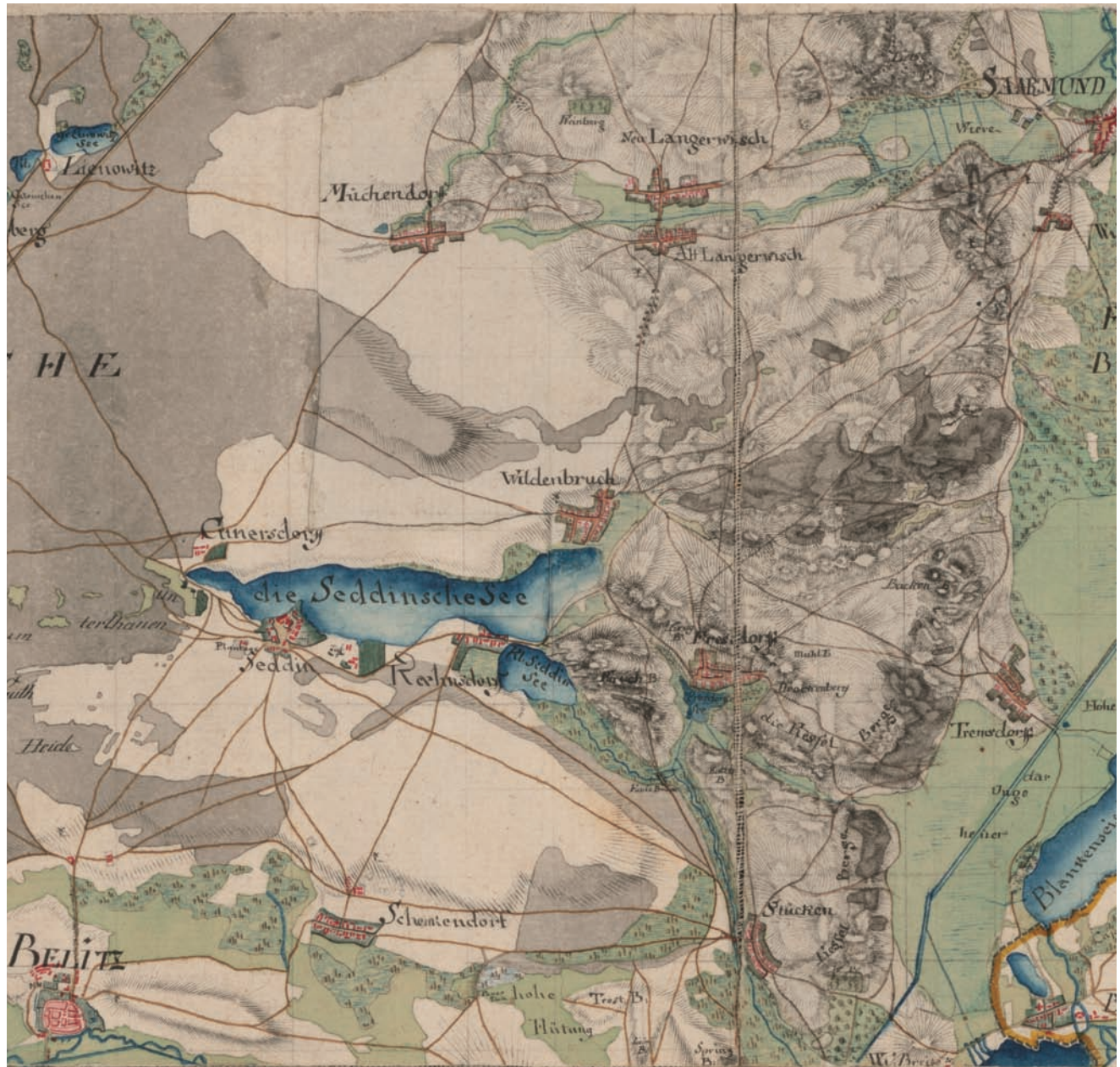
FIG. 829. DETAIL FROM SHEET 89 (BELITZ) OF THE “SCHMETTAUSCHE KABINETTSKARTE,” BY FRIEDRICH WILHELM CARL VON SCHMETTAU (1767–87). Manuscript; 1:50,000. Roads, individual buildings, and land cover are shown, with relief indicated by hachures and shading, in the area around Seddiner See, south of Berlin.
