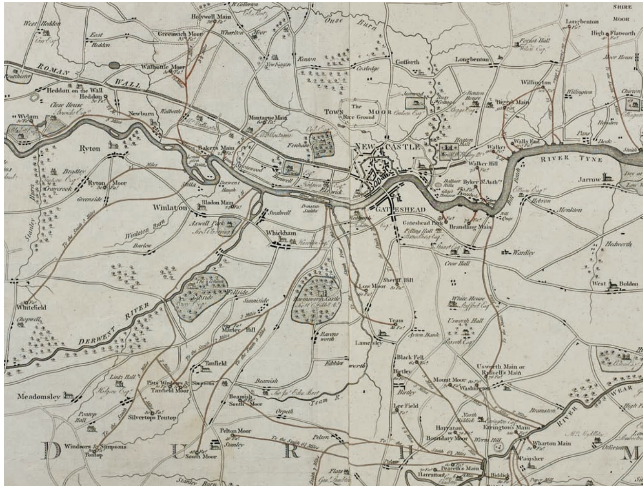
FIG. 794. DETAIL FROM JOHN GIBSON, PLAN OF THE COLLIERIES ON THE RIVERS TYNE AND WEAR ALSO BLYTH, BEDLINGTON AND HARTLEY , 1788. This map of collieries shows their depth in fathoms and the wagon ways (in red) by which the coal was moved to the
