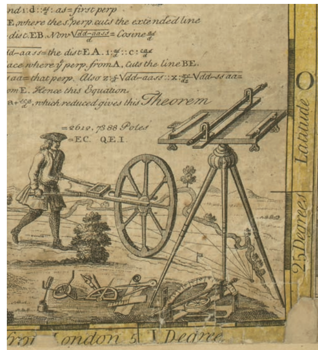
FIG. 834. VIGNETTE OF PERAMBULATOR, PLANE TABLE, AND OTHER SURVEYING INSTRUMENTS FROM A CARTOUCHE ON HENRY BEIGHTON'S MAP OF WARWICKSHIRE (1728). Beighton surveyed Warwickshire from 1722 to 1725 ( A Mapp of Warwick-shire . . . Actually Survey'd in the Years 1722, 1723, 1724, 1725 ). The wheel of the perambulator shown here appears much smaller than that for which Beighton had advocated.
