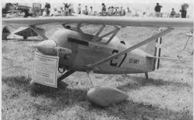
This big Curtiss Racer by Ralph Brunner was powered by a Quadra 40. It weighs 26 lbs. and has a wingspan of 95 inches.
