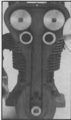
Dual over head cams are belt driven.
