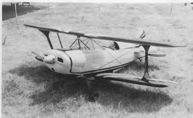
A huge 90-inch span Pitts by Gim Goodemote weighing 37 lbs. It is powered by a 10 hp Sachs engine.
