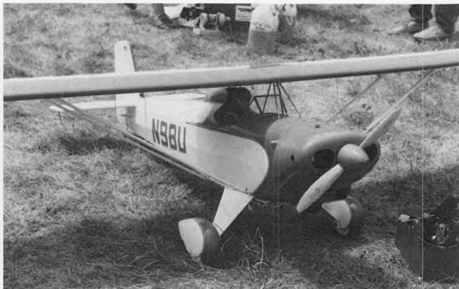
Great Planes makes this nice kit for a Corben Baby Ace. This one, seen at Olean was built by Bruce Knox and was powered by an O.S. .80 two-stroke. Plenty of power for this 11 lb. craft.
