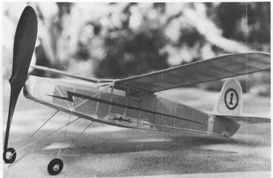
Long-nosed version of the Moth using carved balsa blank from Oldtime Modeler Supply to keep the nose light.
