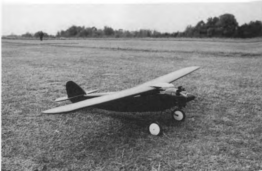
John Mountjoy's Cessna AW was scratchbuilt and covered with Permagloss Coverite. Flying weight is 8.8 lbs. Uses a sport cobalt 60 with 21 1200 cells. It's 1/6 scale.
