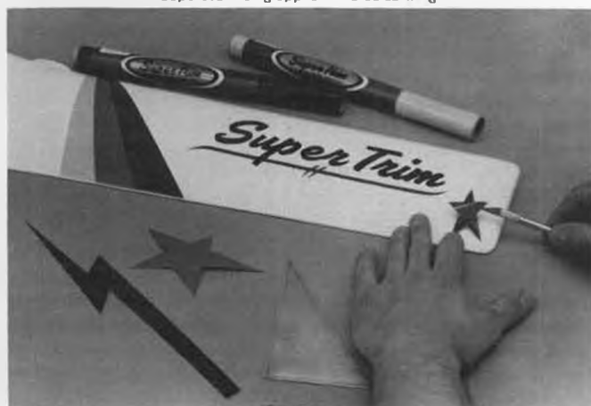
SIG molded foam wing covered with white Supercoat and decorated with SuperTrim.
