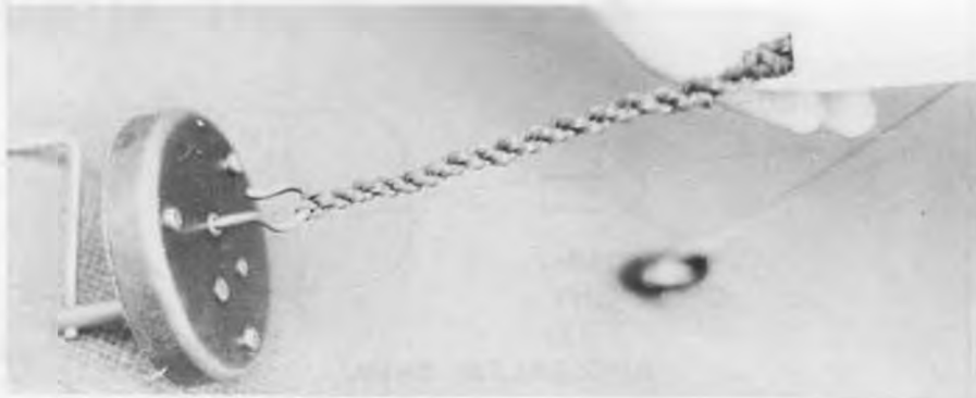
A braided motor helps control rubber bunching in the tail and the C.G. shift and stall that results. Details in text.
