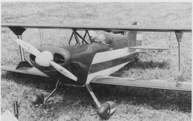
A very aerobatic Weeks Special was powered by a Saito 270 and was scratchbuilt by William Morlan.
