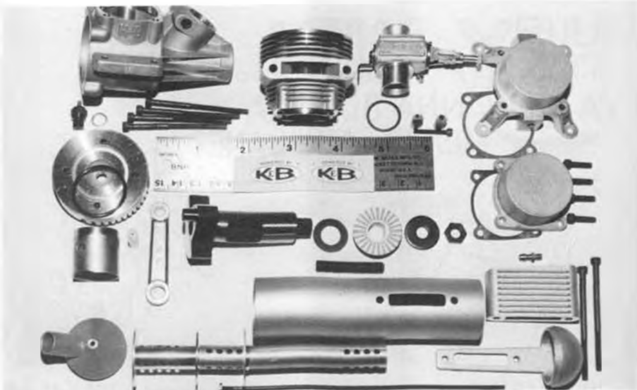
Engine has about 60 parts, including clever auxilliary "spider" mount in top right corner for firewall mounting. Crankshaft's disc is .415 inches thick and contributes to excellent idle performance through its rotating mass. The muffler is the most effective to date.
