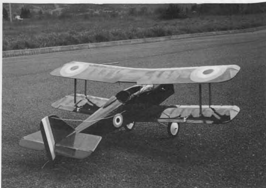
JP Foley's SE5A with a geared 25 cobalt. It hasn't flown yet; too heavy at 100 oz.
