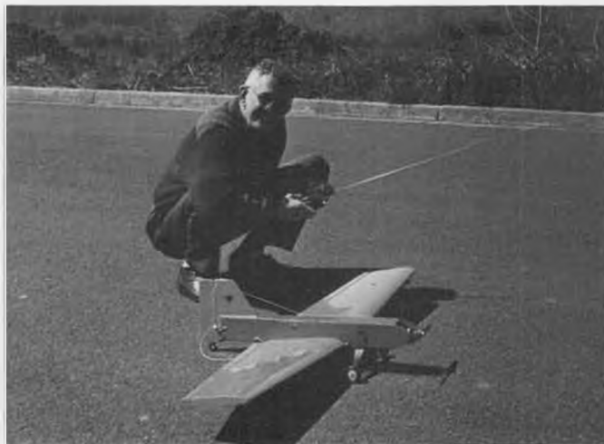
A wild plane in the air, it's Bill Evans' Scimitar Slo Motion. Direct drive, 14 1200 cells and a 25 cobalt motor.
