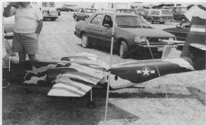
This semi-scale 54 pound DeHavilland Caribou was built by Stan Dzon. Model is 1/7 size and powered by two Sachs 3.1 engines.
