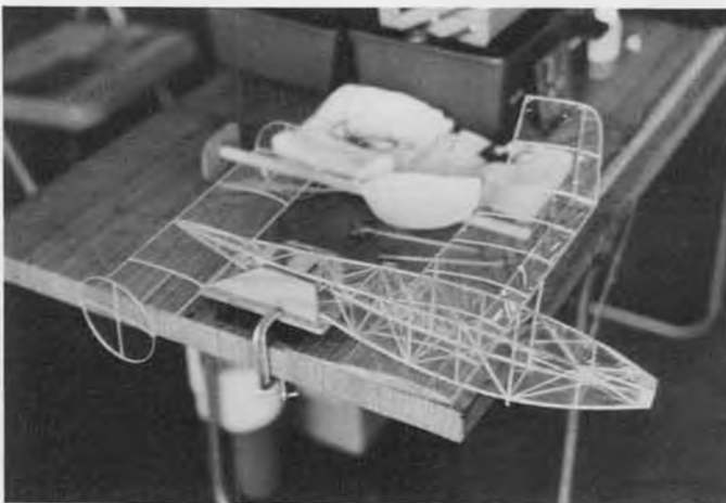
MIAMA's Tony Becker uses stooze to wind his twin tail Manhattan Cabin model.
