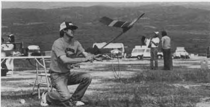
Terry Thorkildsen VTO's his 1/4A Top Banana in Nostalgia. Model is powered by a Nostalgia-legal Cox TD .020.
