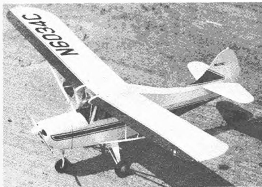
Wing lights, gas caps, antenna, typify details that make a stand-out craft. Cabin side slope automatically provides the dihedral.
