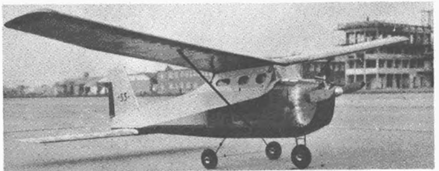
Built for an altitude attempt, 80-in. job, Harald Kurth, Germany, 8 lbs., .60 engine, one channel.
