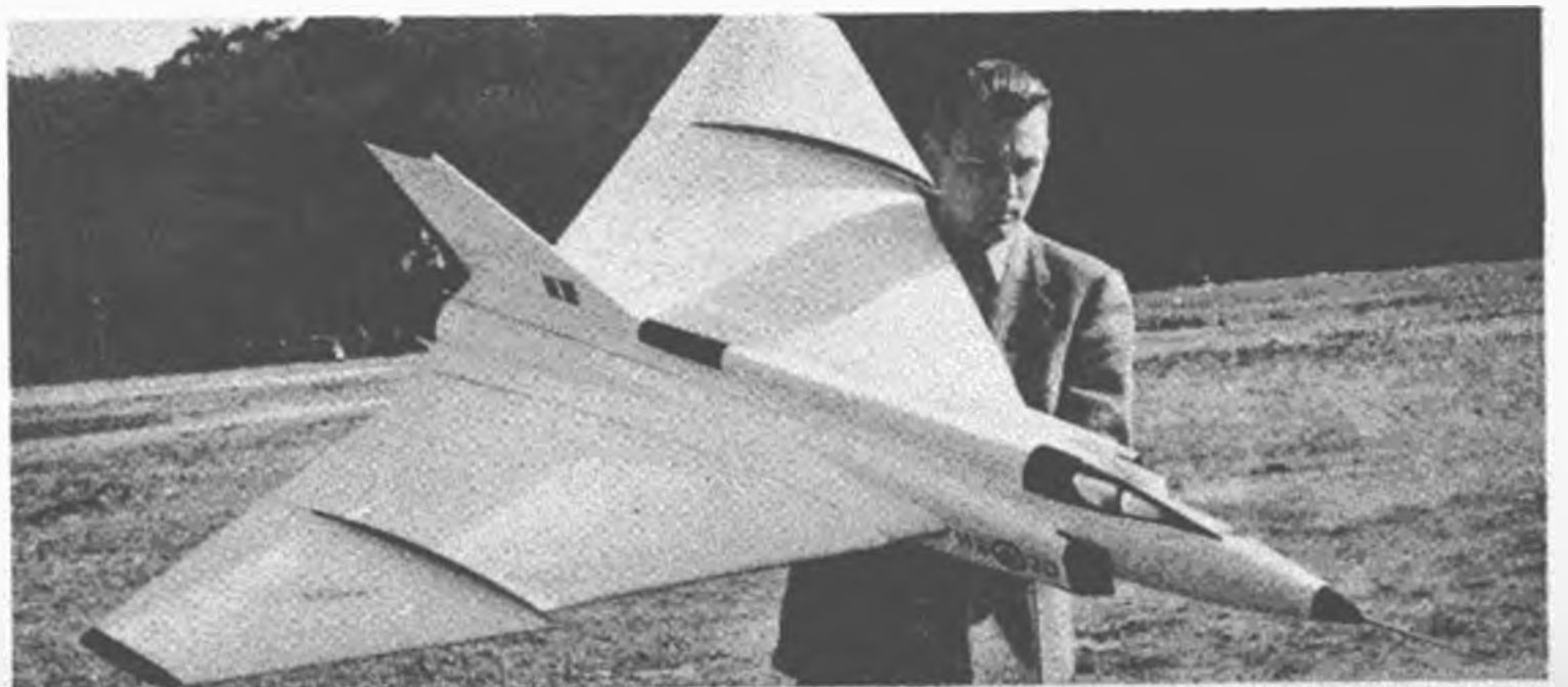
Arvo Arrow, G. Kittner, Germany, 70-in. delta, with K & B .35 power. Weighs 7½ lbs., single channel.
