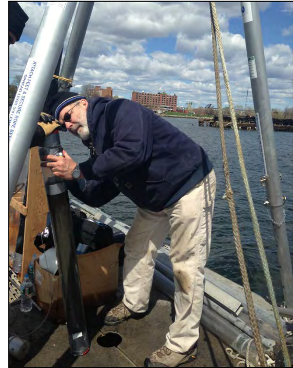
Figure 2-8. Limited geological sediment sampling consisting of biological coring and vibracoring was conducted in the Green Jacket Shoal marine archaeological study area in early May 2015 to assess the area’s archaeological sensitivity and potential of the shoal to contain preserved elements of a formerly exposed submerged paleocultural landscape. URI-GSO CML graduate student, Brian Caccioppoli, monitors vibratory coring operations (left image); URI-GSO CML graduate students Casey Hearn and Brian Caccioppoli and URI-GSO professor and CML director, John King, taking a biological core (center image); John King labeling a recovered biological core (right image) (source: photographs by David Robinson, CML).
