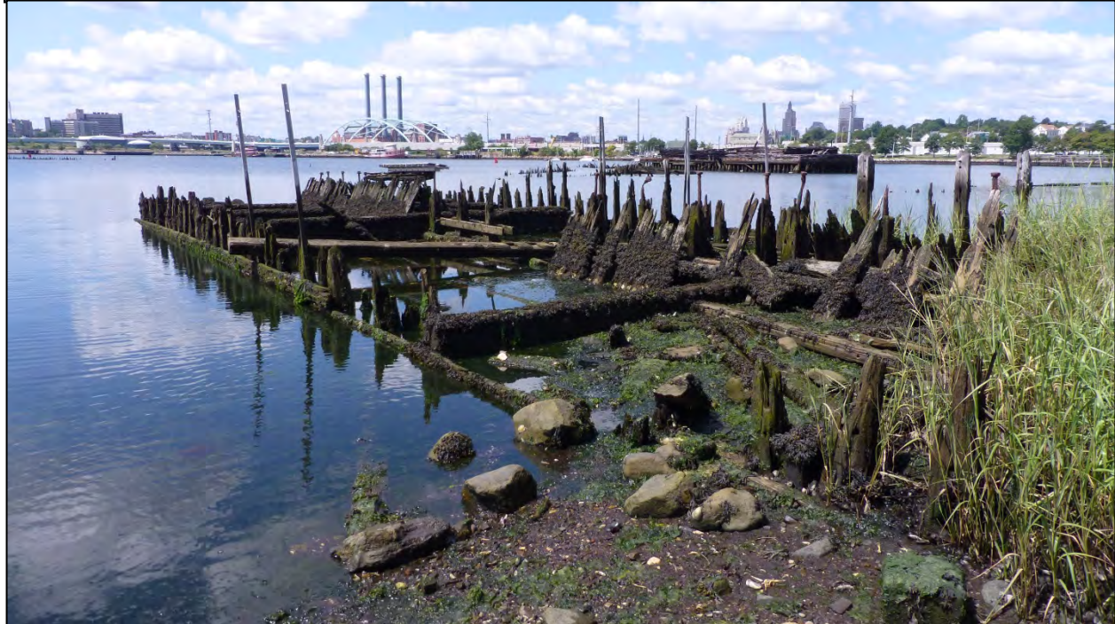
Figure 5-7. Different types of scow barges present in the study area – SW-2, a large modern (less than 50 years old) ocean-going barge (note curved end) (upper image) and an historical (more than 50 years old) inland waterway work-barge (SW-7) with centerline framing designed to help support weight on deck, rather than to carry bulk cargoes inside its hull (source: photographs by David Robinson, CML).
