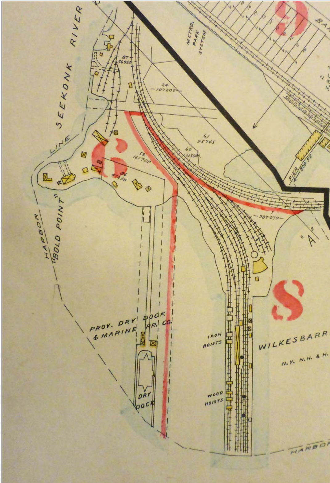
Figure 4-8. Detailed depiction of the Providence Dry Dock and Marine Railway Company property in 1917. Note the unique “tuning-fork” shape of the dry dock pier and the shape of the floating dry dock slipped within the pier (source: Richards Standard Atlas 1917).
