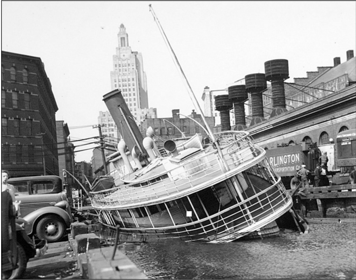
Figure 3-7. Photograph showing some of the damage in Providence from the New England Hurricane of 1938 (September 21), which brought with it into the city a storm surge of 17.6-foot (5.4 m) (source: David Robinson, CML [personal collection]).
