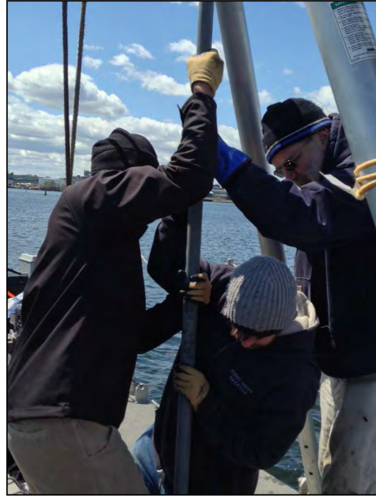
Figure 2-8. Limited geological sediment sampling consisting of biological coring and vibracoring was conducted in the Green Jacket Shoal marine archaeological study area in early May 2015 to assess the area’s archaeological sensitivity and potential of the shoal to contain preserved elements of a formerly exposed submerged paleocultural landscape. URI-GSO CML graduate student, Brian Caccioppoli, monitors vibratory coring operations (left image); URI-GSO CML graduate students Casey Hearn and Brian Caccioppoli and URI-GSO professor and CML director, John King, taking a biological core (center image); John King labeling a recovered biological core (right image) (source: photographs by David Robinson, CML).
