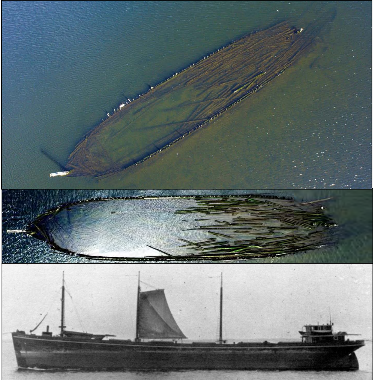
Figure 5-8. SW-12 is the remains of a large schooner-barge representing the last chapter in the history of America's merchant sailing vessel developmental chronology. The reduced sailing rig of a schooner-barge required a smaller crew and was less costly to operate. The rig was intended primarily for auxiliary purposes and could be used in the event of a break in the tow-line to the steam-tug that would have pulled a string of several schooner-barges joined together. Schooner-barges were employed in the bulk-cargo carrying trade and most often carried stone, grain, lumber and coal. The after-half of SW-12's hull remains is full of rough-cut logs that may be unused pier piles that were discarded in the hulk (source: aerial photographs by Glenn Anderson; image of the schooner-barge underway from Morris 1984).
