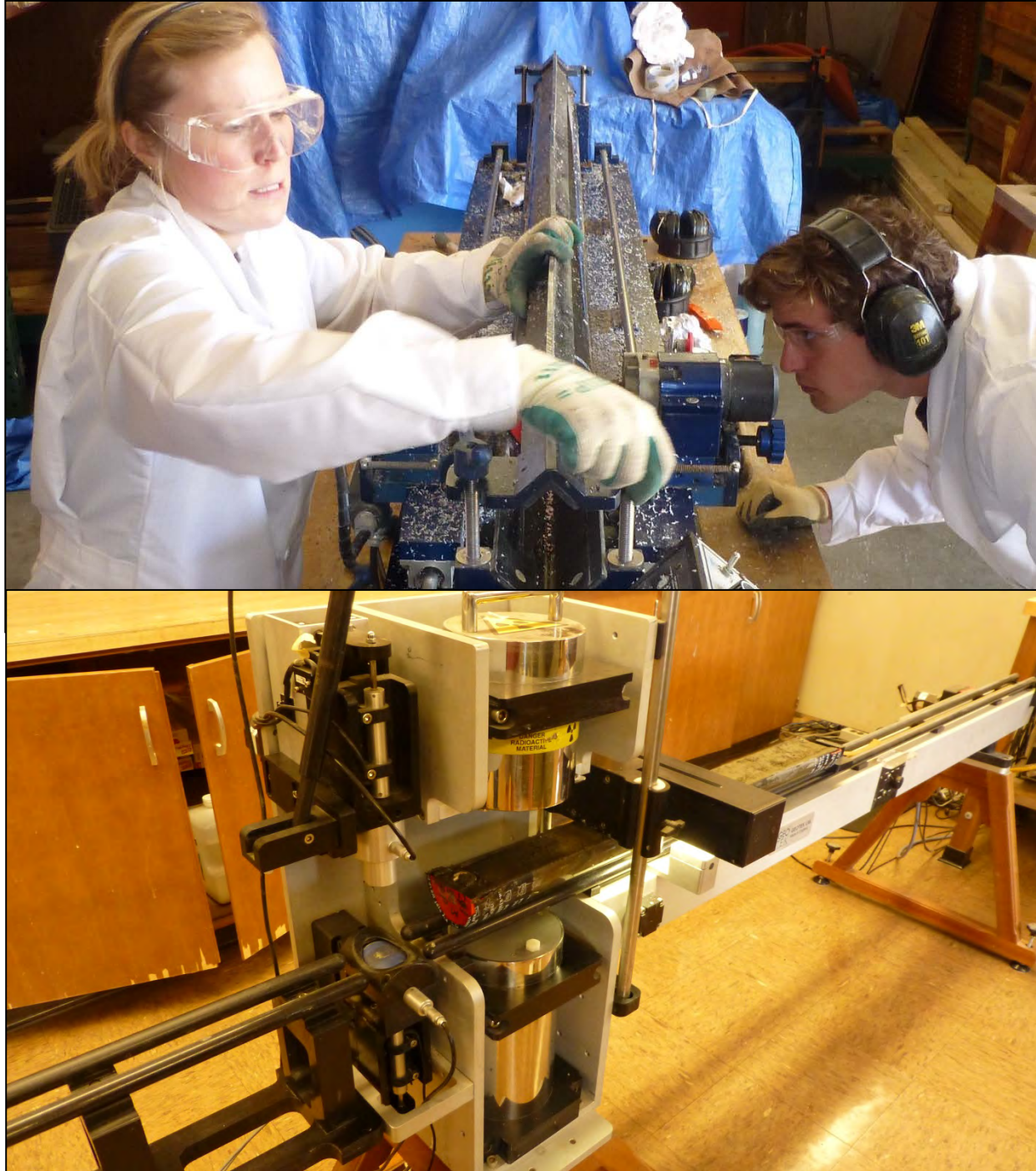
Figure 2-9. CML's lab manager, Danielle Cares, and project volunteer, Michael Robinson, splitting a core sample (upper image); core logging on CML's Geotek core logging machine (lower image) (source: photographs by David Robinson, CML).
