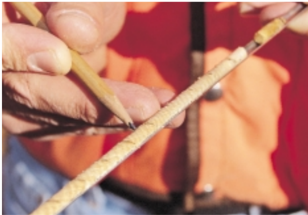
School Forest Manager Alex Finkral counts the rings on a piece of a tree’s stem that was extracted by an instrument called an increment core. Counting the rings and examining their size determines a tree’s age and radial growth rate, and is an important part of dendrochronological research. Such research is used in examining disturbance history, climate change trends, and growth responses to silvicultural treatments.
