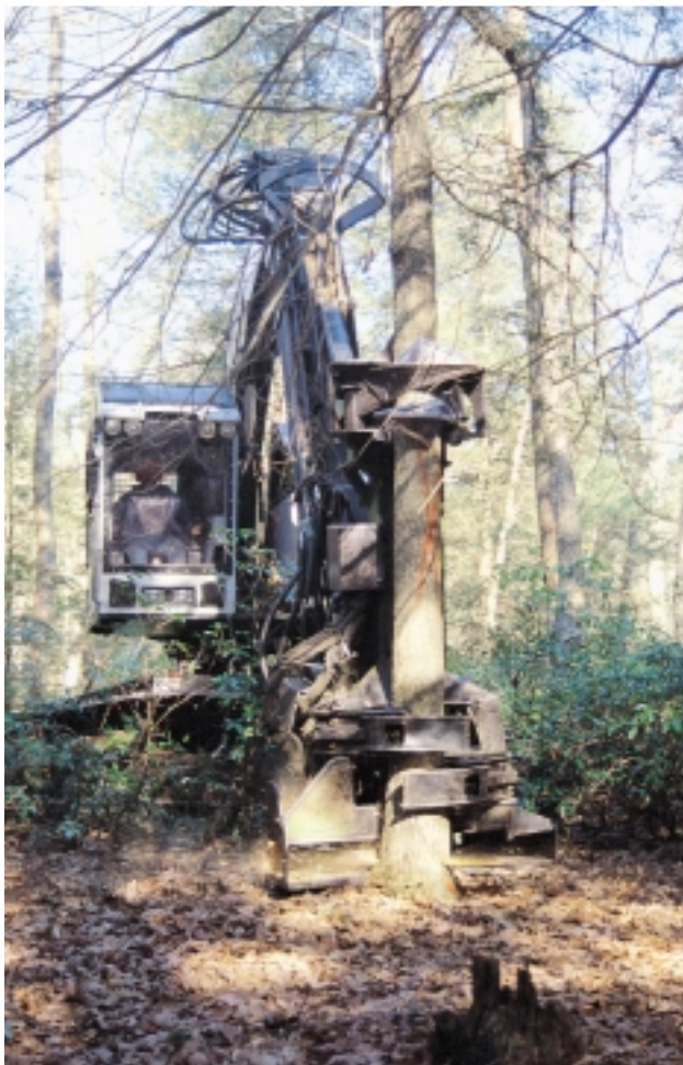
To prepare for the timber harvest, Tom Bernier operates a machine that grips a tree with a vice-like arm, strips trees of their limbs, cuts timber to merchantable length, and neatly deposits the debris on the forest floor.
