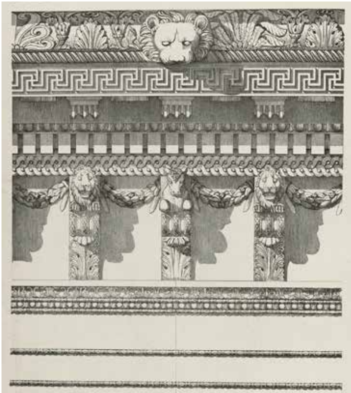
Fig. 52 Reconstruction drawing of cornice, Temple of Jupiter Heliopolitanus
