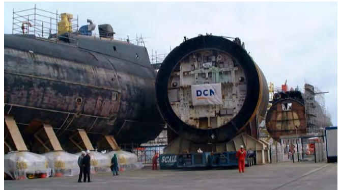
Removal of a reactor unit © DGA
