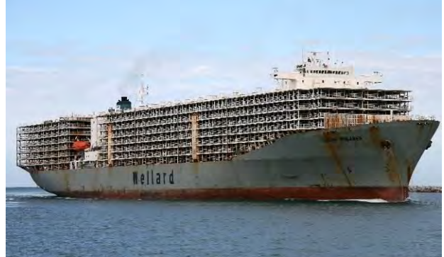
12 Ocean Shearer . The ex container ship could take 120,000 sheeps on cruise from Australia to the Middle East.
