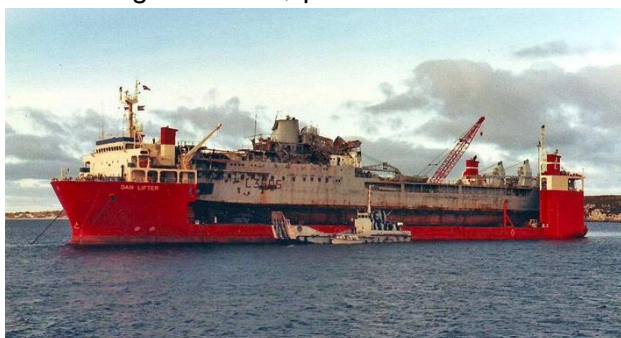
Late 1982, the heavy load carrier Dan Lifter is bringing back home the landing ship Sir Tristram damaged in the Falklands war. © Ken Griffiths
