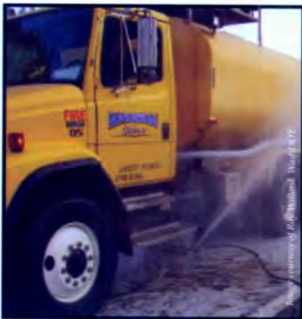
"An affordable weed washer (innovative portable invasive species rinse off and reclaim system) designed for highway construction and maintenance" equipment now exists.
