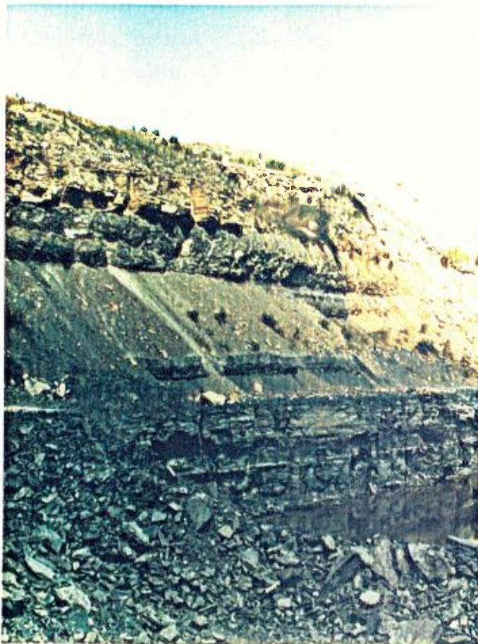
Plate 3. Interbedded sequence of claystone and laminite with a thin sandstone lens (top) exposed in the operating pit of Wearn Industries Pty Ltd at Mulgoa.
