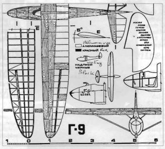
December 2000-January 2001, p7). Part of the plans – complete with the grain of the wood – for the Russian G-9: is a prototyple Esprit twin-engine wing span, 12.07m; wing area, 13.0m²; length, 3.77m; aspect ratio, 11.3; ultralight motorglider, designed by max L/D, 17.5; and empty weight, 150kg. See Soviet Aerobatics (below left)
