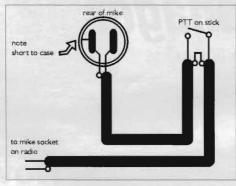
Fig 4: a simple microphone wiring circuit
