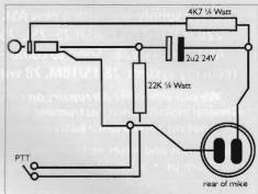
Fig 5: a simple two-terminal microphone circuit
