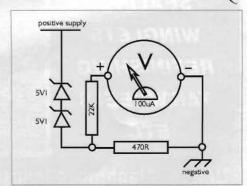
Fig 6: Suppressed zero meter. Calibrate before use!
