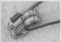
Above: a suitable supply filter can help prevent noise in the cockpit
