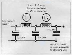
Fig 1: Circuit for a supply filter (see photo above right)
