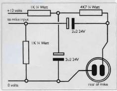
Fig 2: a two-terminal microphone circuit
