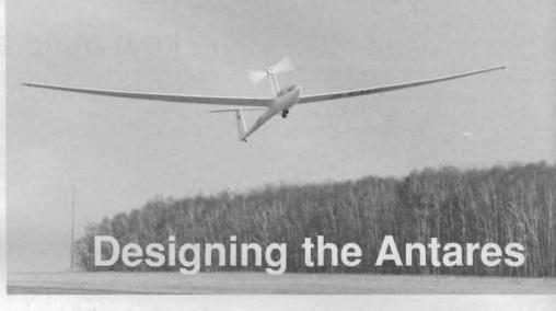
and sound emission less than 40dB – very quiet. The powerful lightweight NiMH batteries, in the inner wings, allow a climb to 1,750m. Engine use is via a simple one-lever control system and an electronic management system. The propulsion system is safe, compact, powerful, silent and vibration free, a development, until recently, considered unlikely.
