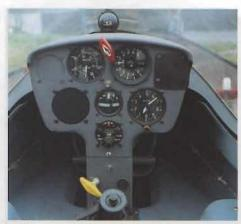
The front panel's cover swings up with the canopy frame
