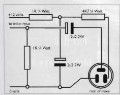
Fig 3: a three-terminal microphone circuit
