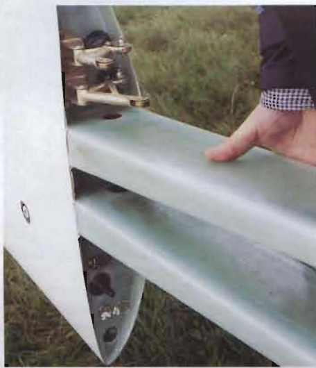
Automatic connections for controls and single pin slot
