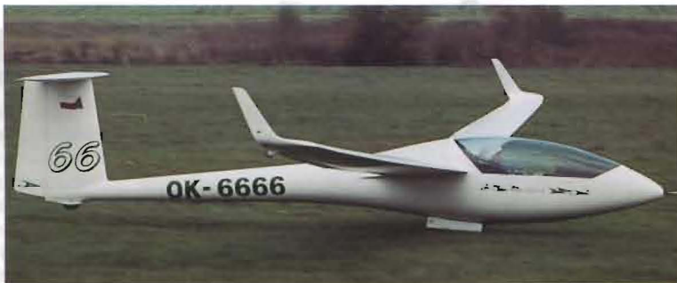
Winglets are elegant, but slightly reduce aileron size; control still good on the ground, though
