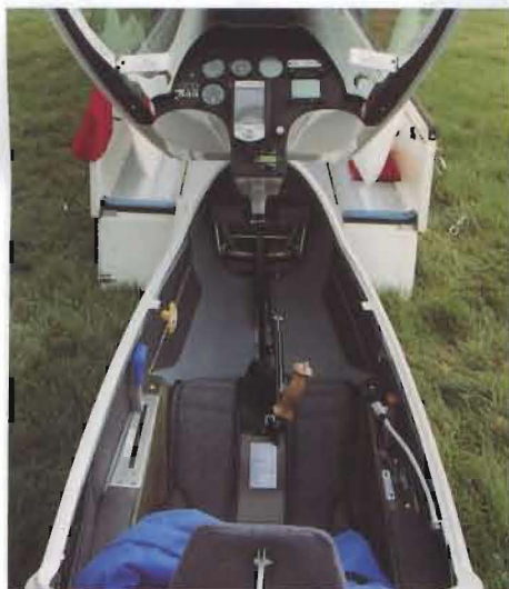
Cockpit is roomy; parallelogram stick and wood handles
