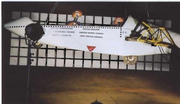
Above: the two-seater hoisted in position for a test against the backdrop of the sight screen. The lights enabled the use of high-speed video to record each of the six tests
