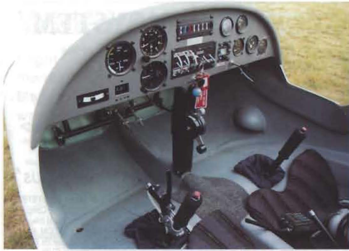
UFM 13/15 Lambada: cockpit and instrument panel
