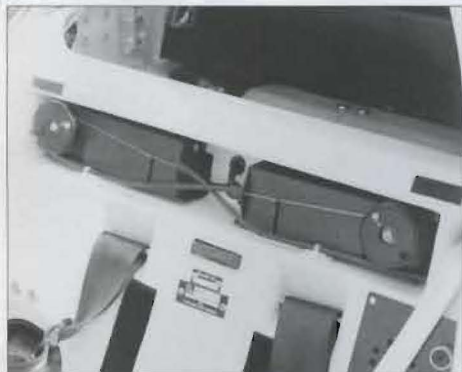
Electronic bugwiper system concealed behind the seat
