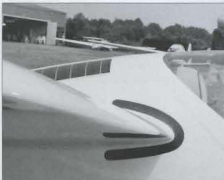
Housing for bugwipers, and optional solar panels fitted
