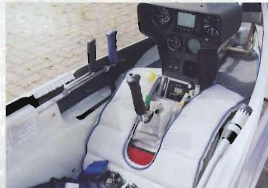
The cockpit, with the low side walls typical of DG gliders
