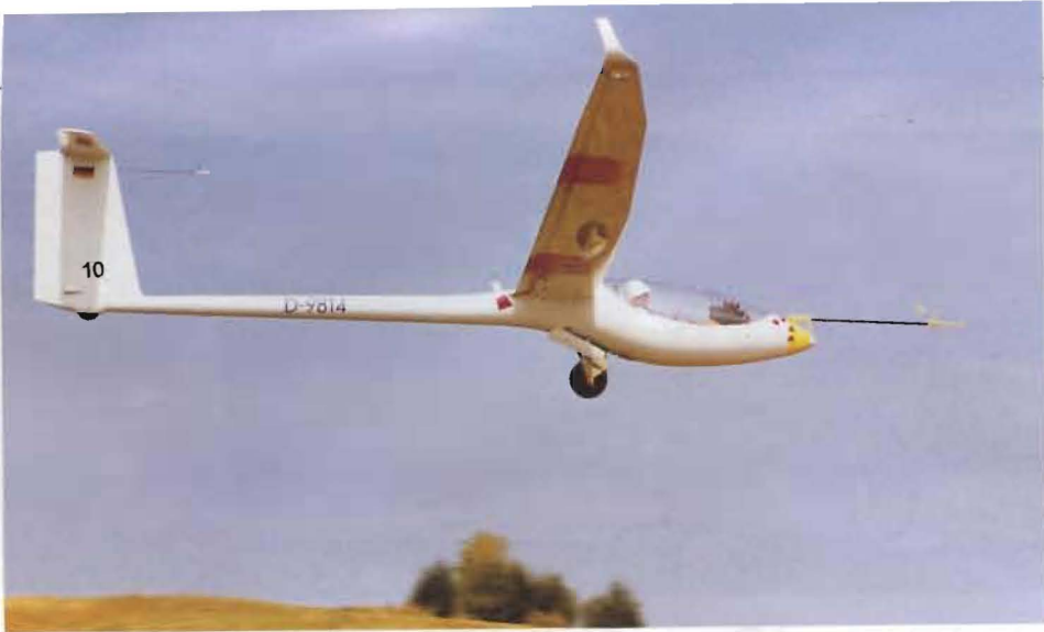
Above: new SB-14 with angle-of-attack/slip probe and fluid under the wing to determine the laminar separation line
