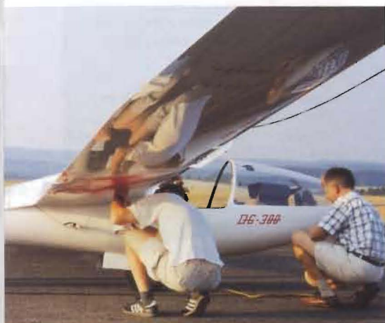
Spraying indicator paint under the DG-300's wing as part of a new method to locate the laminar separation bubble, using protective plastic film on aerotow
