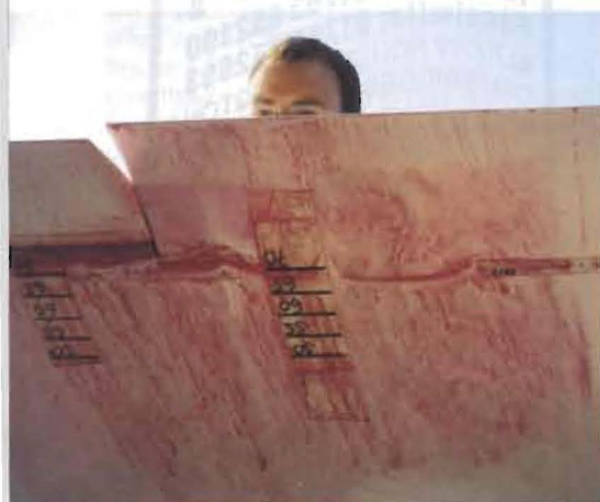
A "fluid flow picture" of the airflow under the wing after flight. The dark red line marks the beginning of the laminar separation bubble
