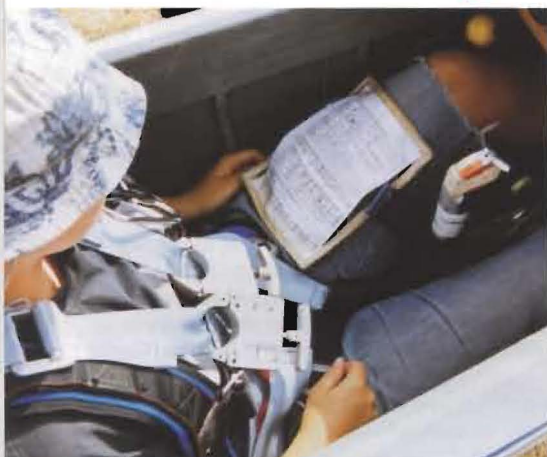
Zacher's legacy: flight test recording form, control force meters on the straps and stick position tape measure. For an obituary of Hans, edited by Manfred Reinhardt, see the news archives at www.glidermagazine.com
