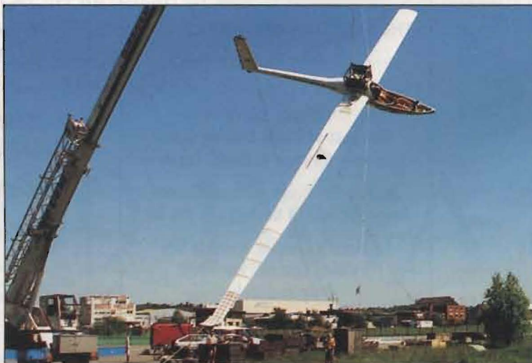
A crash test on a glider which has lost a wing in a mid-air collision.
