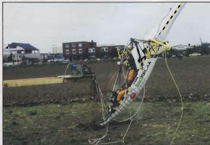
Glider ground-impact tests at FH Aachen, Germany.
