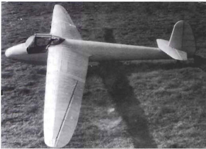
A swing-wing glider in 1944 with twin, retractable wheels! The Hirth 21, with the wings swept forward.
