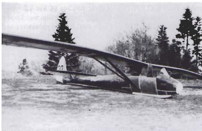
The CW-5 which Waclaw Czerwinski designed and which first flew in 1931. Note the all-moving tail mounted on high hinges to keep the tips of the tailplane off the ground. Photo Peter Startup.
