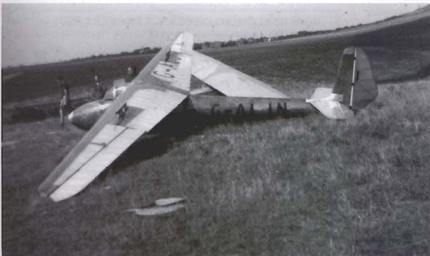
Dudley Hiscox's Chilton Olympia at Dunstable in 1950-52, showing the varnished wood and clear doped fabric. Photo Les Moulster.
