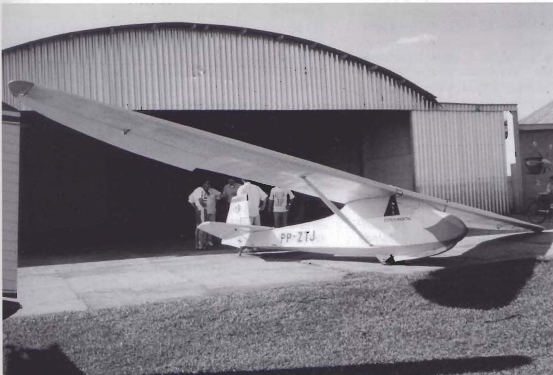
30 Grunau Babies were built in Brazil in the 1940s with a wheel, wooden struts, rounded nose and modified ailerons. Photo Frederico Fiori.
