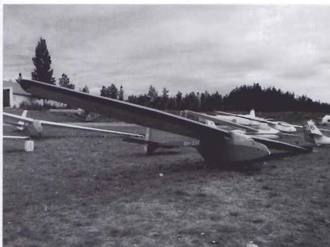
An unfamiliar glider from Finland. A Pik-5 which is now 50 years old. The wing was originally designed by Wacław Czerwiński for the Polish Salamandra. Photo Taisto Saarinen
